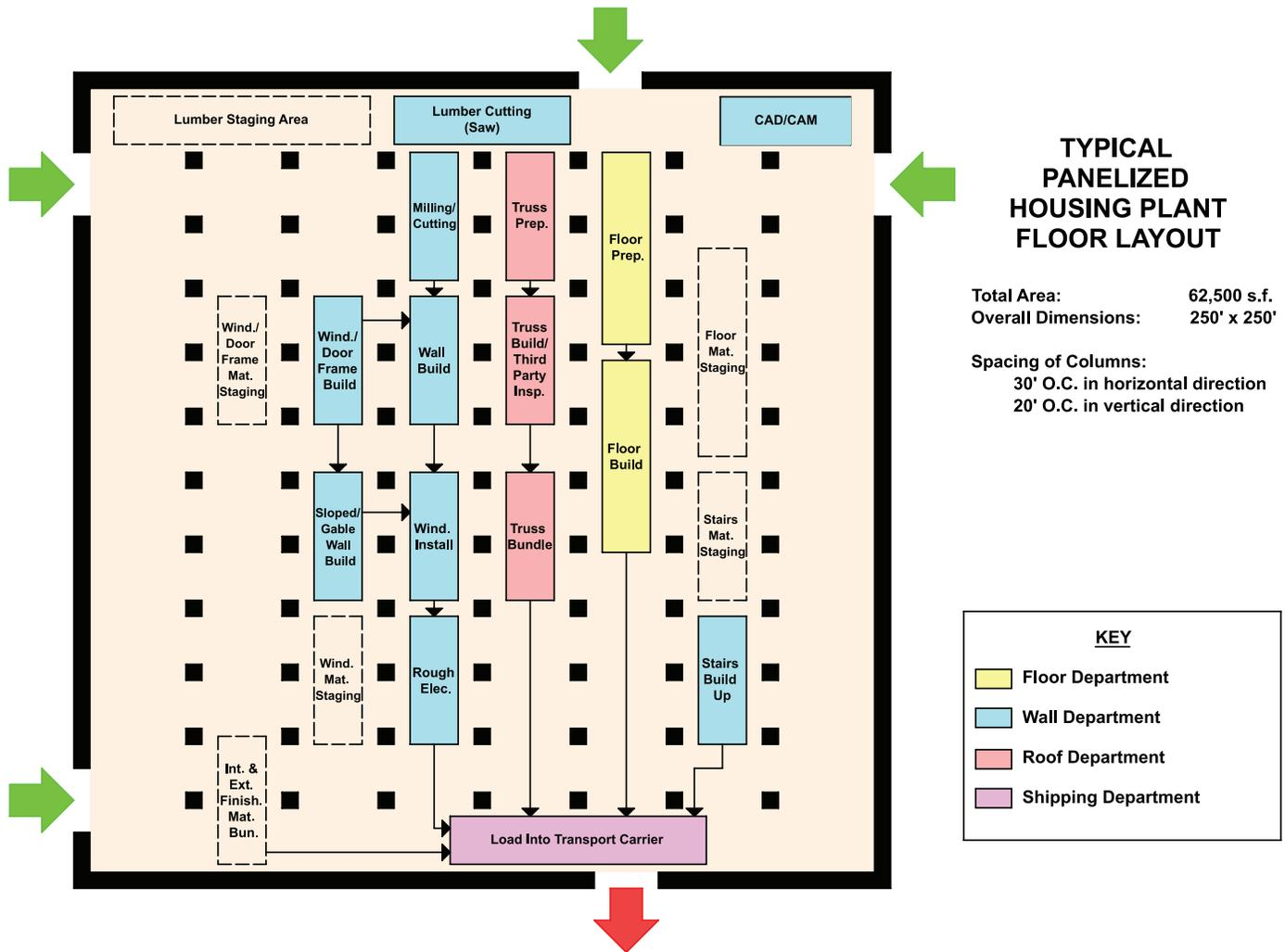
Figure 4-2: Typical Panelized Whole-House Plant Process Flow
