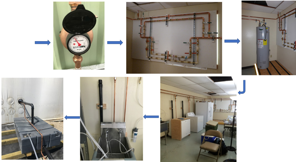
Note: Shown clockwise from the upper left are the water meter, removable pipe sections, hot water heater, appliances, sink, and tank that collects water from the system. Source: U.S. Environmental Protection Agency— https://www.epa.gov/emergency-response-research/water-security-test-bed
