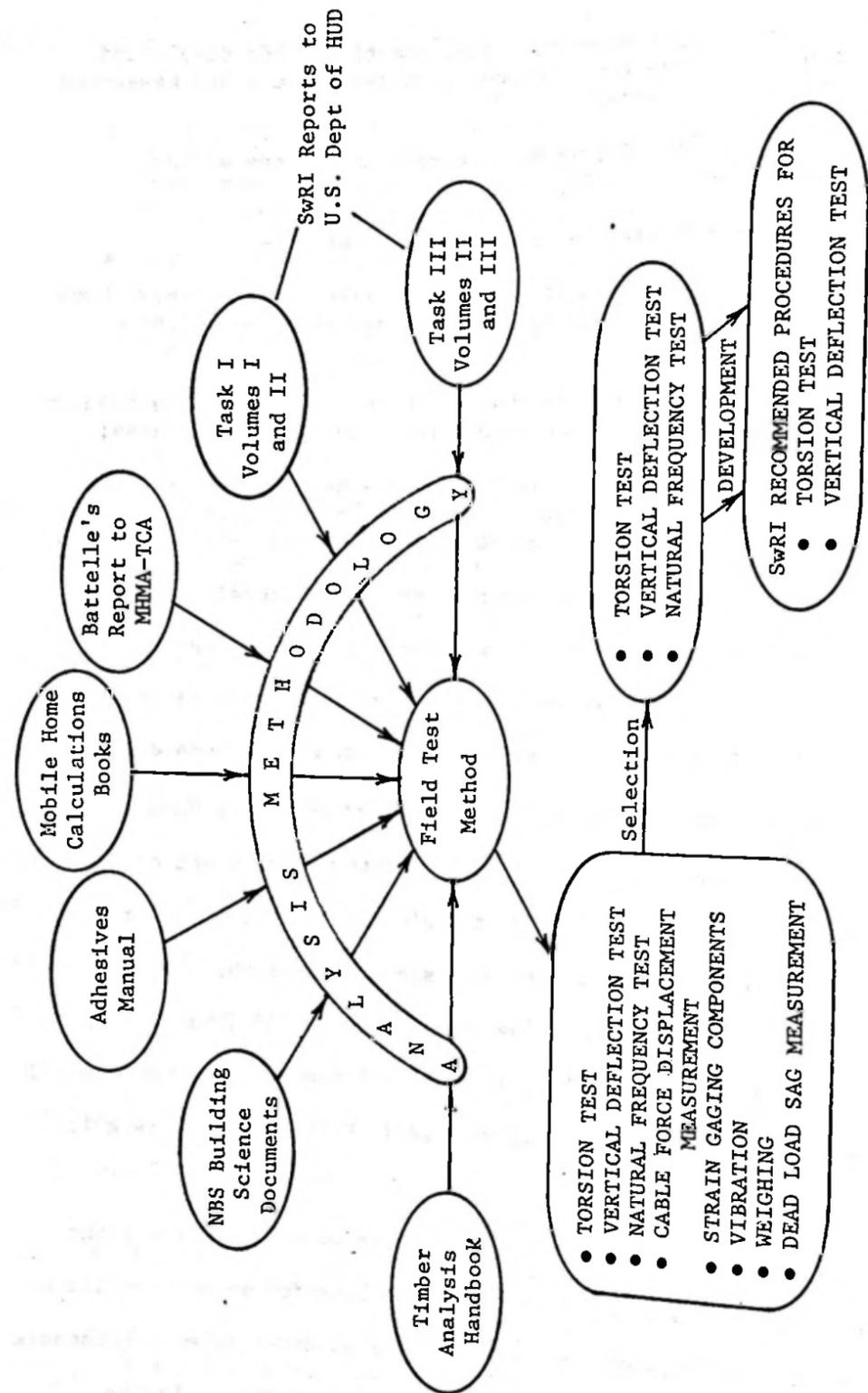
Figure 1. Flow Chart of Development of a Plan to Create a Field Test Method
