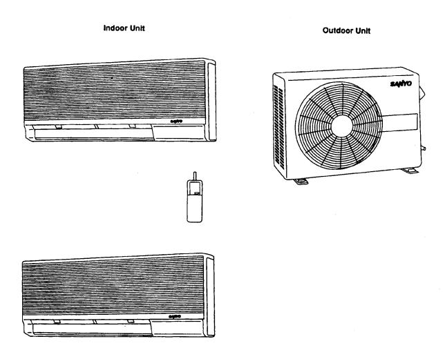
Figure 2. Two-Zone Ductless System Courtesy of Sanyo Fisher Corporation
