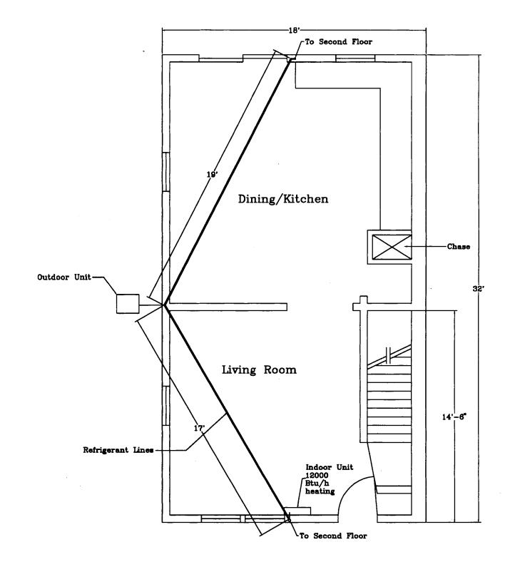
Figure 4. Demonstration Home - First Floor (Note: Refrigerant lines may be run outside or in basement.)
