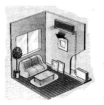
Figure 1. Typical Ductless Heat Pump System Courtesy of Sanyo Fisher Corporation
