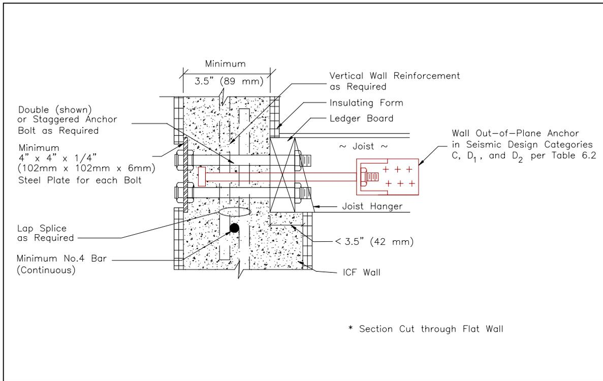
**Figure 6.7 Floor Ledger-ICF Wall Connection (Through-Bolt Connection)**
