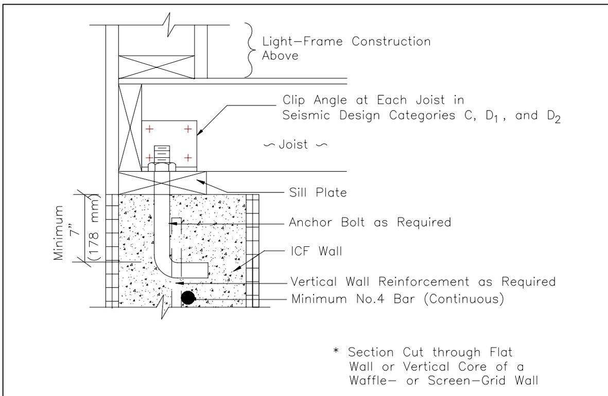
**Figure 6.2 Floor on ICF Wall Connection (Top-Bearing Connection)**
