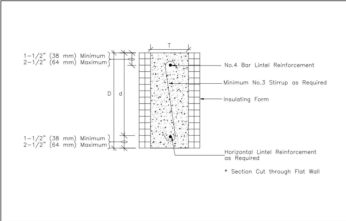
**Figure 5.3 Flat ICF Lintel Construction**
