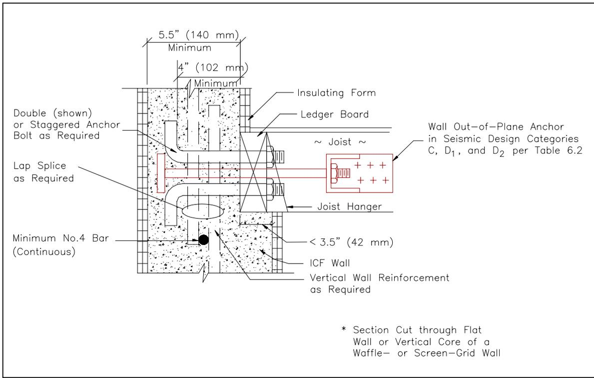
**Figure 6.5 Floor Ledger-ICF Wall Connection (Side-Bearing Connection)**
