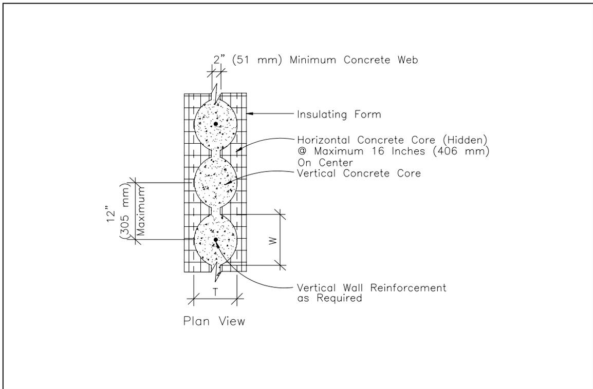
**Figure 2.2 Waffle-Grid ICF Wall System Requirements**
