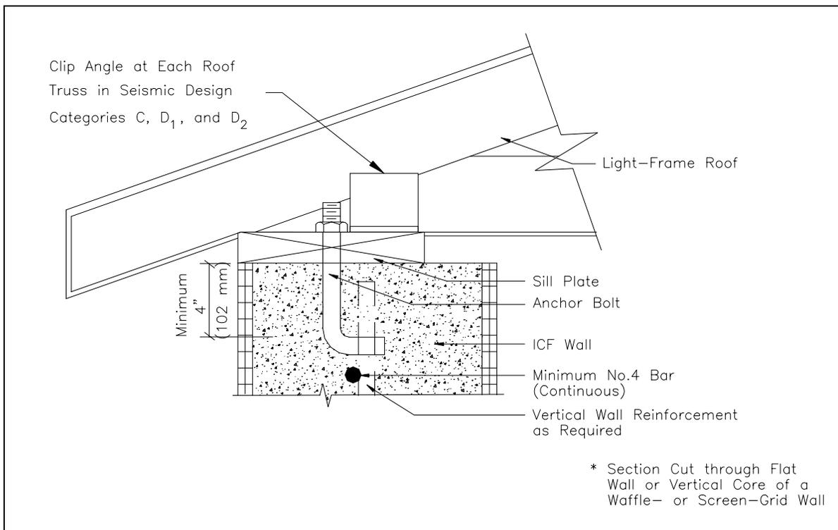
**Figure 6.8 Top Wood Sill Plate-ICF Wall System Connection**
