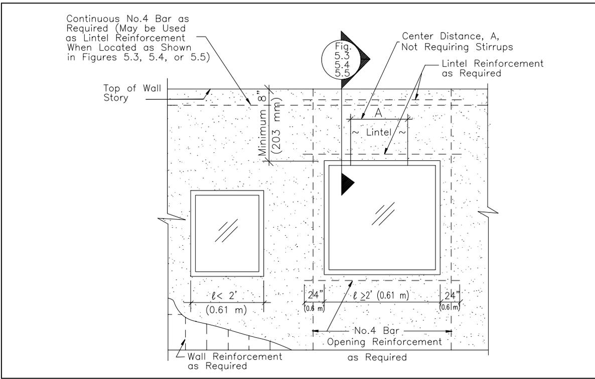
**Figure 5.2 Reinforcement of Openings**
