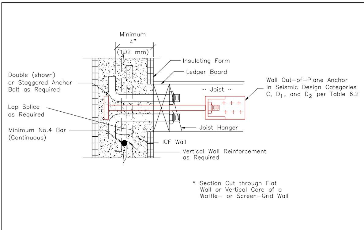
**Figure 6.4 Floor Ledger-ICF Wall Connection (Side-Bearing Connection)**
