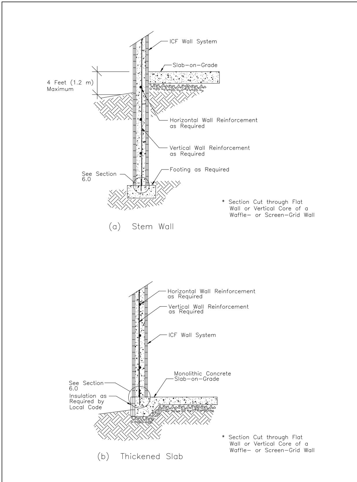
**Figure 3.1 ICF Stem Wall and Monolithic Slab-on-Grade Construction**
