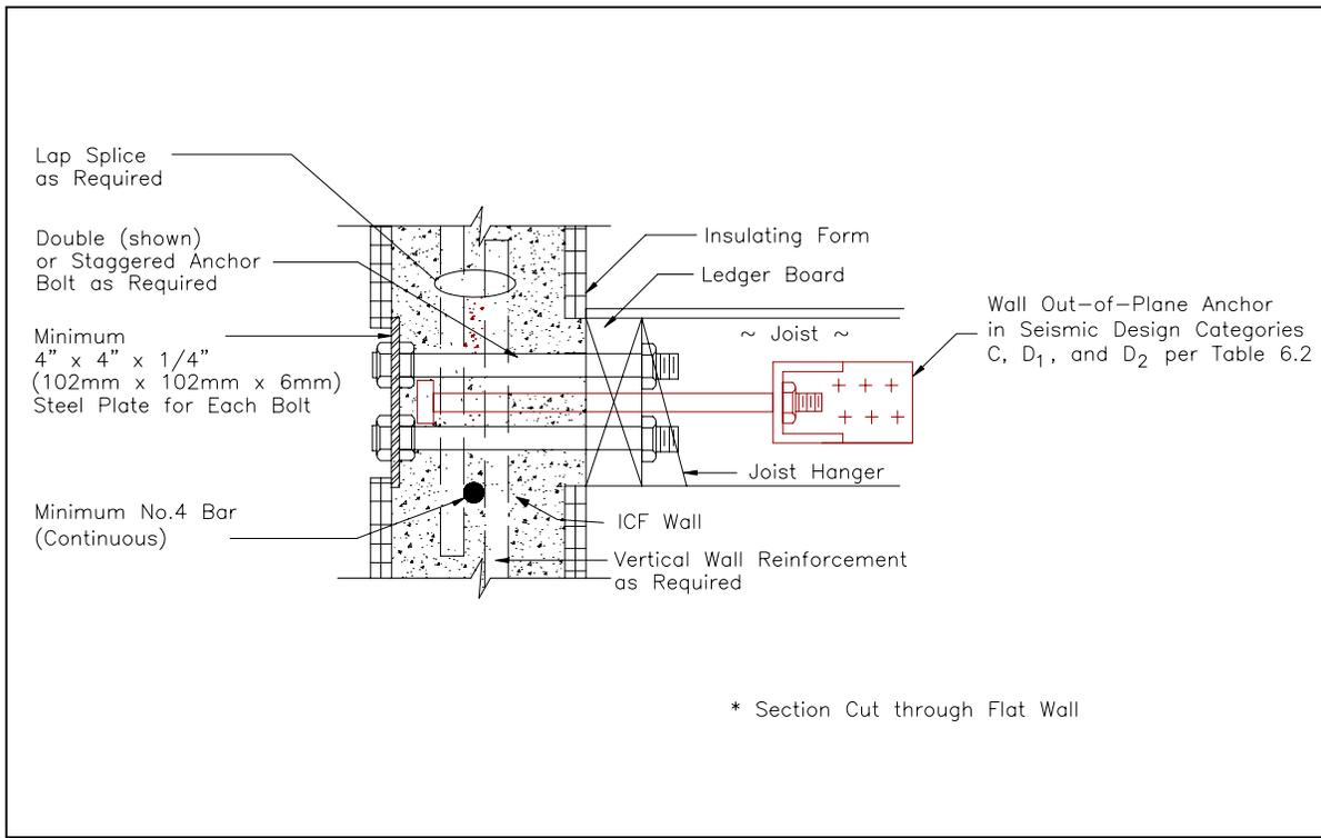
**Figure 6.6 Floor Ledger-ICF Wall Connection (Through-Bolt Connection)**
