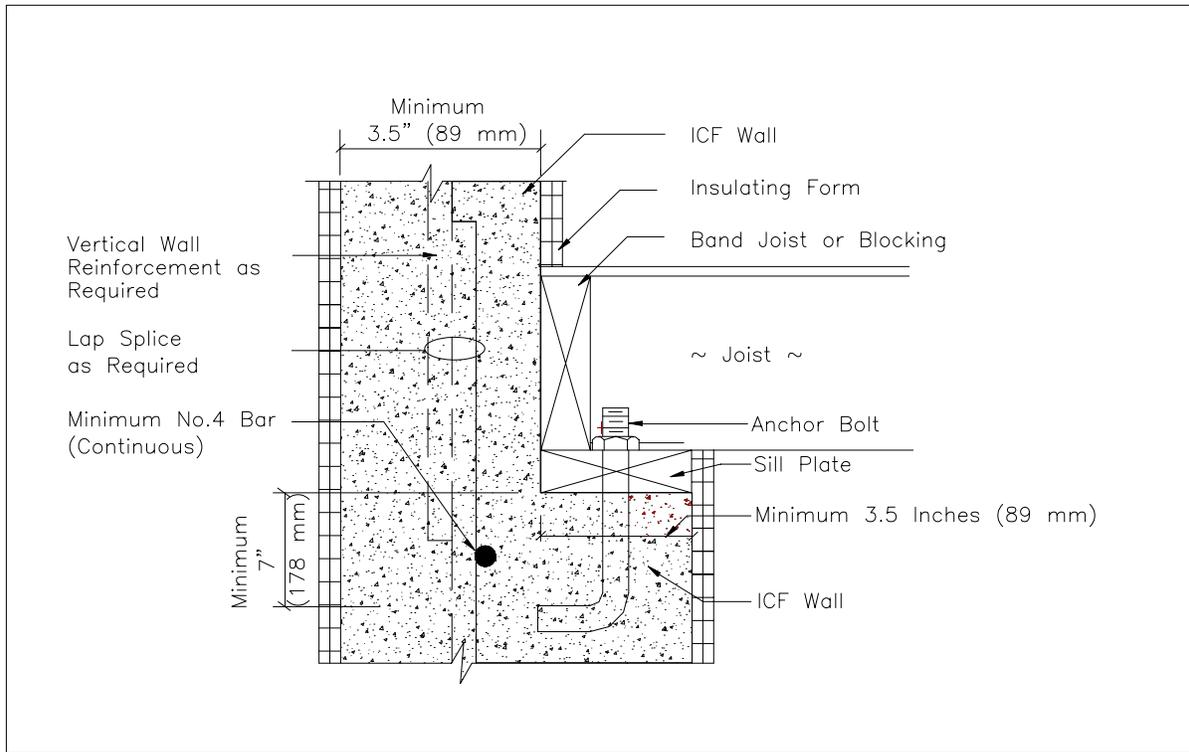
**Figure 6.3 Floor on ICF Wall Connection (Top-Bearing Connection)**
