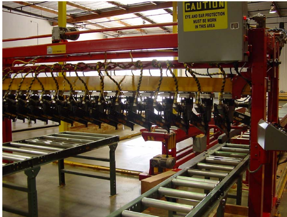
Gang-nail panel machine in a wood-frame open-wall panel factory in California
