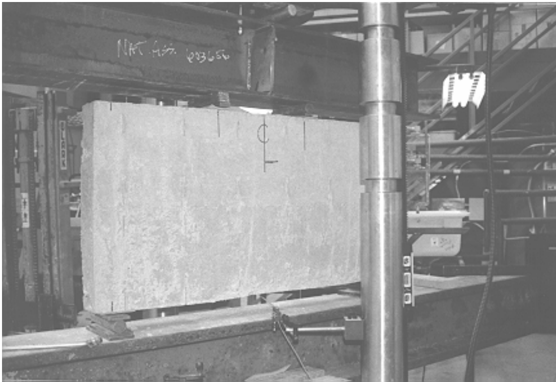
Figure 2 Flat 4x12 Specimen in Universal Test Machine
