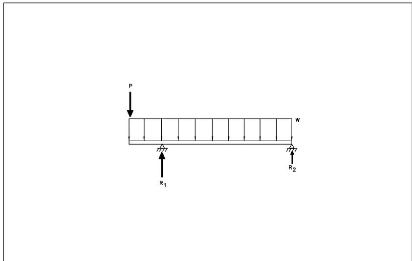
**Cantilever Joist Load Diagram****Find**
