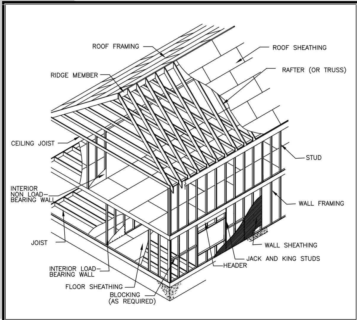
Each system can be complex to design as a whole; therefore, simple analysis usually focuses on the individual elements that constitute the system. In some cases, “system effects” may be considered in simplified form and applied to the design of certain elements that constitute specifically defined systems. Structural elements that make up a residential structural system include:
