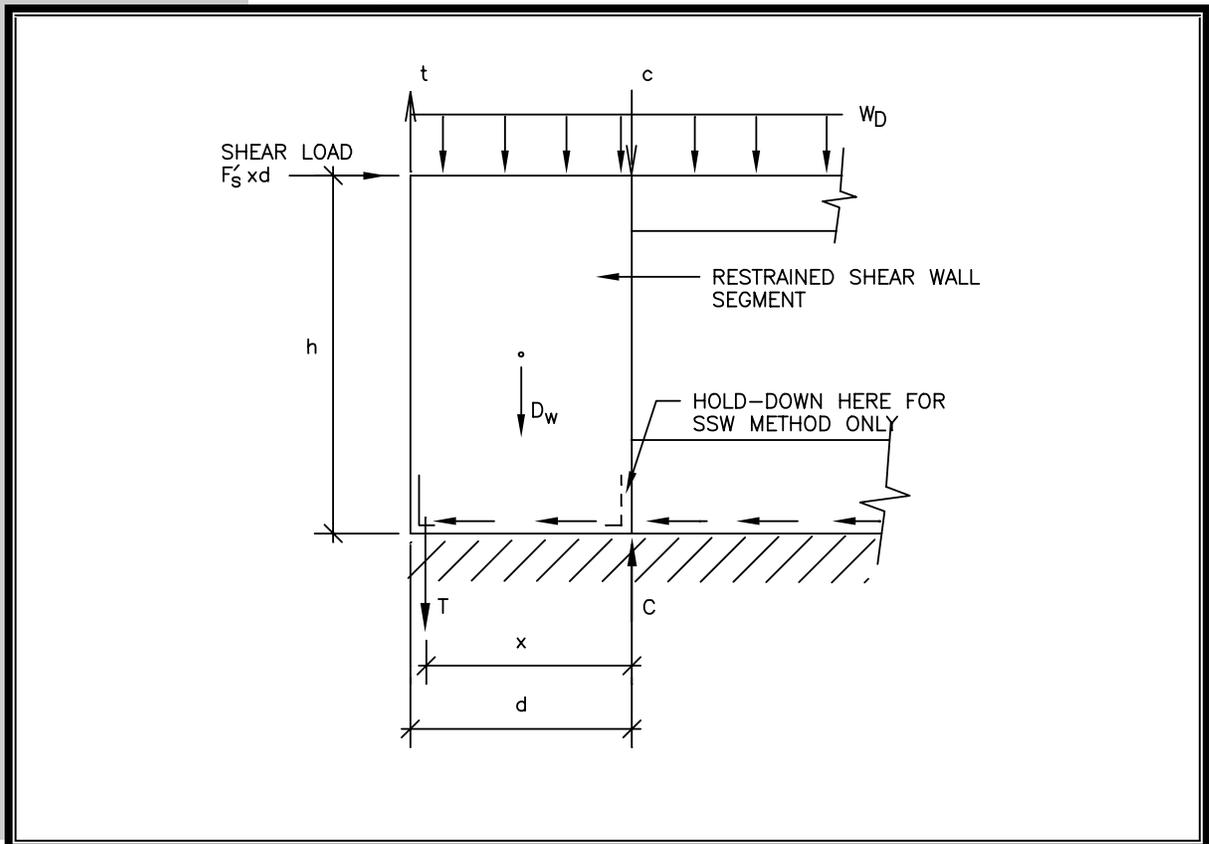
For a more simplified analysis of overturning forces, the effect of dead load may be neglected and the chord forces determined as follows using the symbols defined as before:
