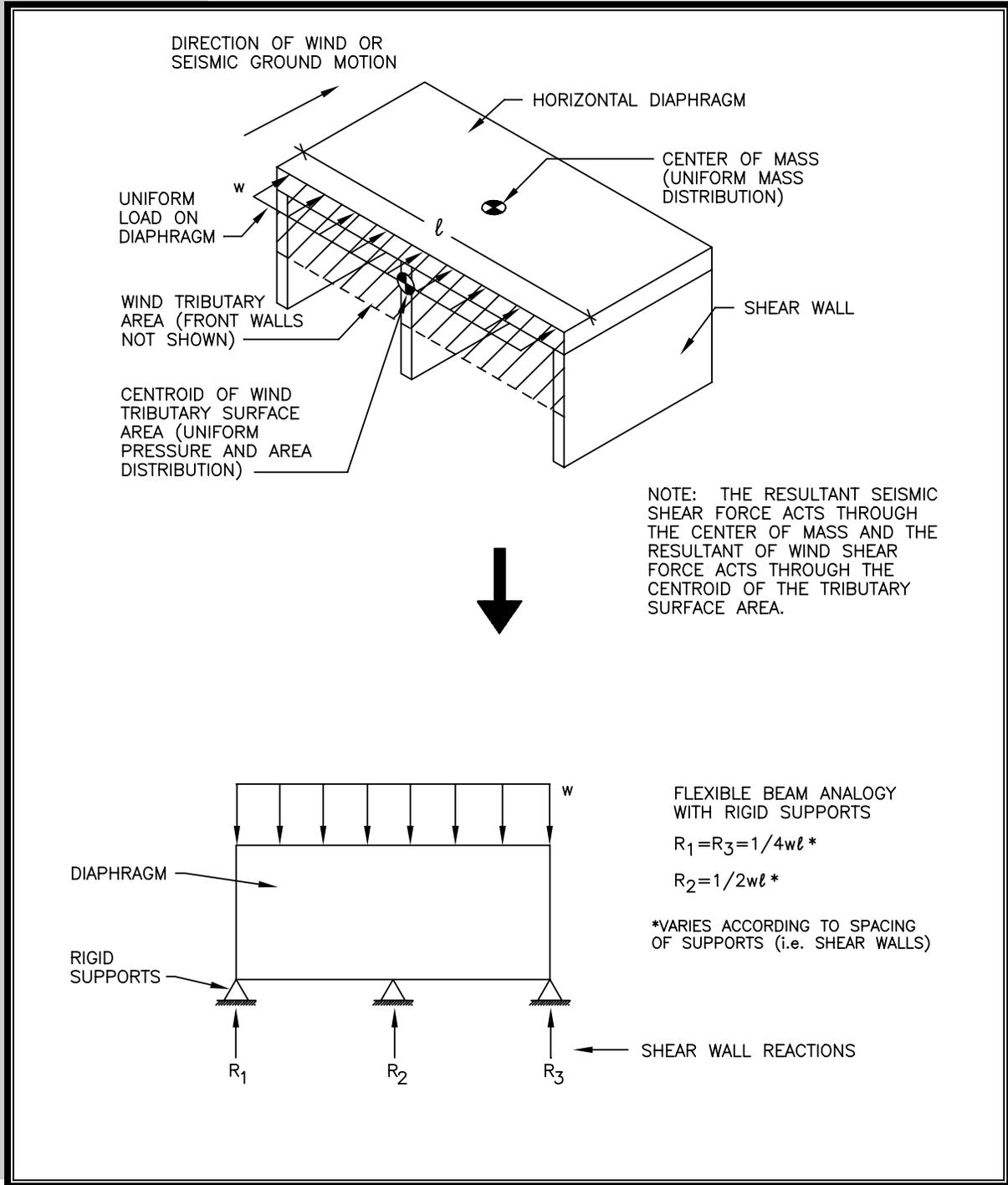
In seismic design, tributary areas are associated with uniform area weights (i.e., dead loads) assigned to the building systems (i.e., roof, walls, and floors) that generate the inertial seismic load when the building is subject to lateral ground motion (refer to Chapter 3 on earthquake loads). In wind design, the tributary areas are associated with the lateral component of the wind load acting on the exterior surfaces of the building (refer to Chapter 3 on wind loads).
