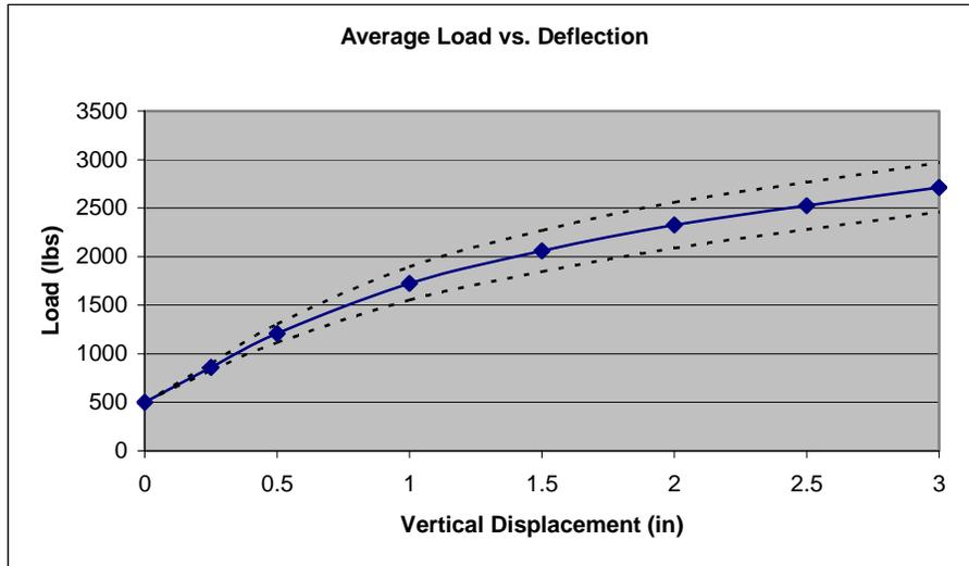
**Figure 3.2.** Average Load vs. Deflection Plot for 90 Degree Axial Withdrawal Tests (n=6) at Georgia Site Using Minuteman 50-inch Anchors with ¾” Shaft and 6” Single Disc (MM650)
