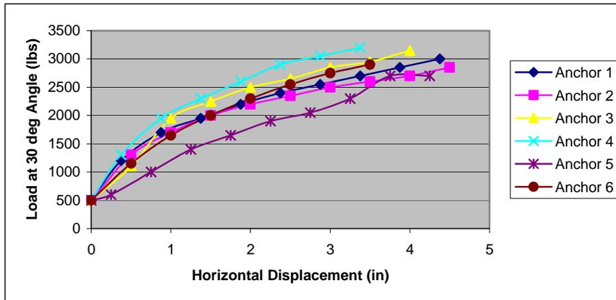
**Figure 3.4.** Load at 30 degree angle vs. horizontal displacement for 30 Degree Angle Pull Tests (n=6) at Georgia Site Using Minuteman 50-inch Anchors with 3/4" Shaft and 6" Single Disc and 17" Stabilizer Plates (MM650+MM17)
