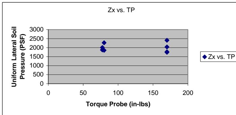
**Figure 4.5.** Scatter plot of Torque Probe readings at 12'' depth vs. lateral soil pressure acting on stabilizer plate based on assumed uniform pressure distribution over surface area of plate reacting horizontal component of angle pull force at anchor head.
