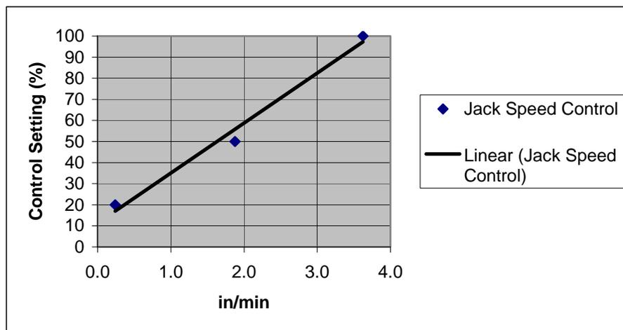
**Figure 2.6.** Displacement rate control of screw jack actuator.
