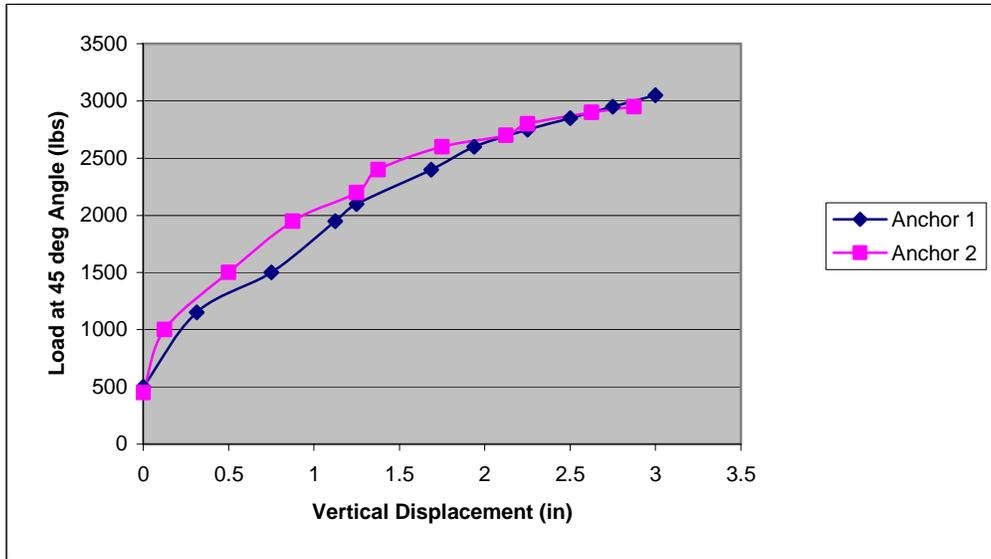
**Figure 3.9.** Load at 45 degree angle vs. vertical displacement for 45 Degree Dual Anchor Axial Pull Tests (n=2) at Georgia Site Using Tie Down Engr 48” x 6” Single Disc Anchors with 3/4” Shaft (TD648)
