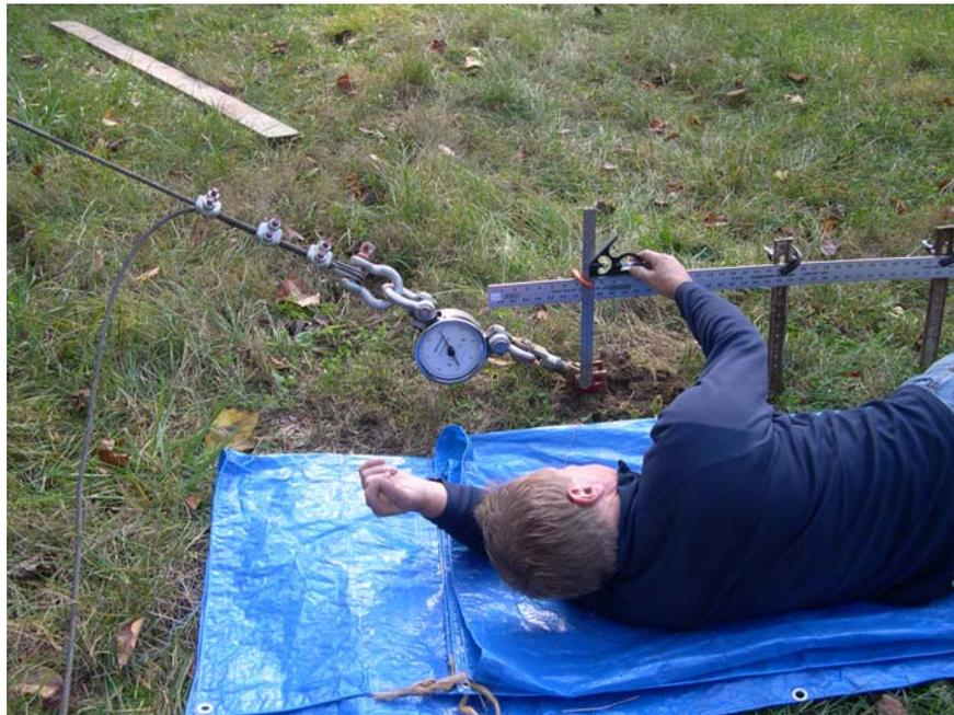
**Figure 2.9.** Deflection measurement technique for angle pull tests.
