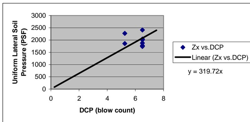
**Figure 4.6.** Scatter plot of DCP blow count at 12'' depth vs. lateral soil pressure acting on stabilizer plate based on uniform pressure distribution over surface area of plate reacting horizontal component of angle pull force at anchor head.
