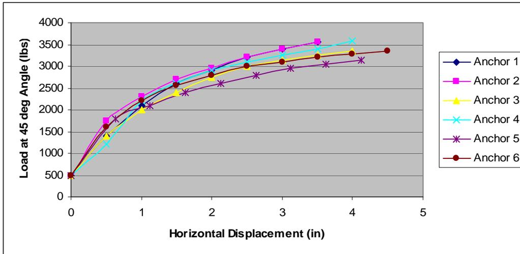
**Figure 3.5.** Load at 45 degree angle vs. horizontal displacement for 45 Degree Dual Anchor Angle Pull Tests (n=6) at Georgia Site Using Minuteman 50-inch Anchors with 3/4” Shaft and 6” Single Disc and 17” Stabilizer Plates (MM650+MM17)
