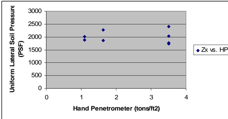
**Figure 4.4.** Scatter plot of Hand Penetrometer (Humbolt Model 4200) readings at 6'' depth vs. lateral soil pressure acting on stabilizer plate based on assumed uniform pressure distribution over surface area of plate reacting horizontal component of angle pull force at anchor head.
