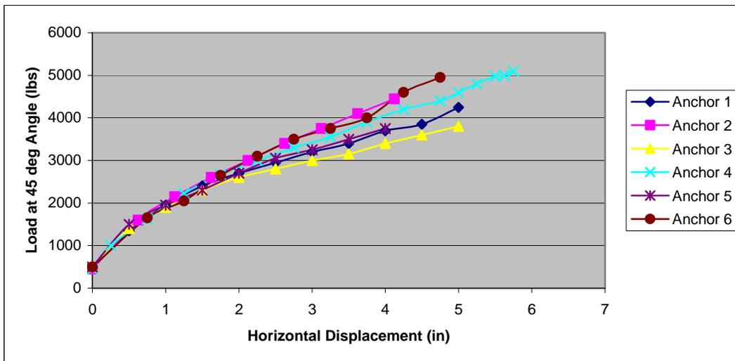
**Figure 3.6.** Load at 45 degree angle vs. horizontal displacement for 45 Degree Dual Anchor Angle Pull Tests (n=6) at Georgia Site Using Tie-Down Engr 48-inch Galv. Anchors with 5/8" Shaft and 6" Single Disc and 17" Stabilizer Plates (TD648+TD/MM17)
