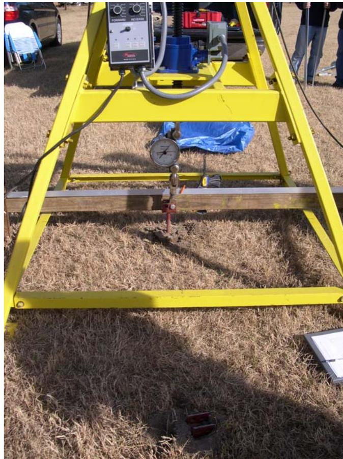
**Figure 2.7.** 90 degree in-line (axial) pull test set-up.
