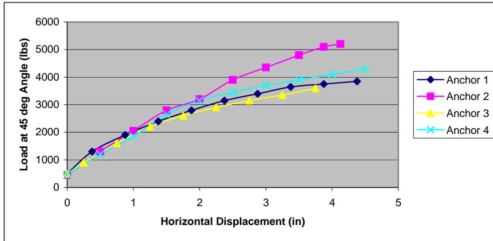
**Figure 3.8.** Load at 45 degree angle vs. horizontal displacement for 45 Degree Dual Anchor Angle Pull Tests (n=4) at Georgia Site Using Home Pride 60” x 8” Single Disc Anchors with 3/4” shaft and 17” Stabilizer Plates (HP860+TD17)
