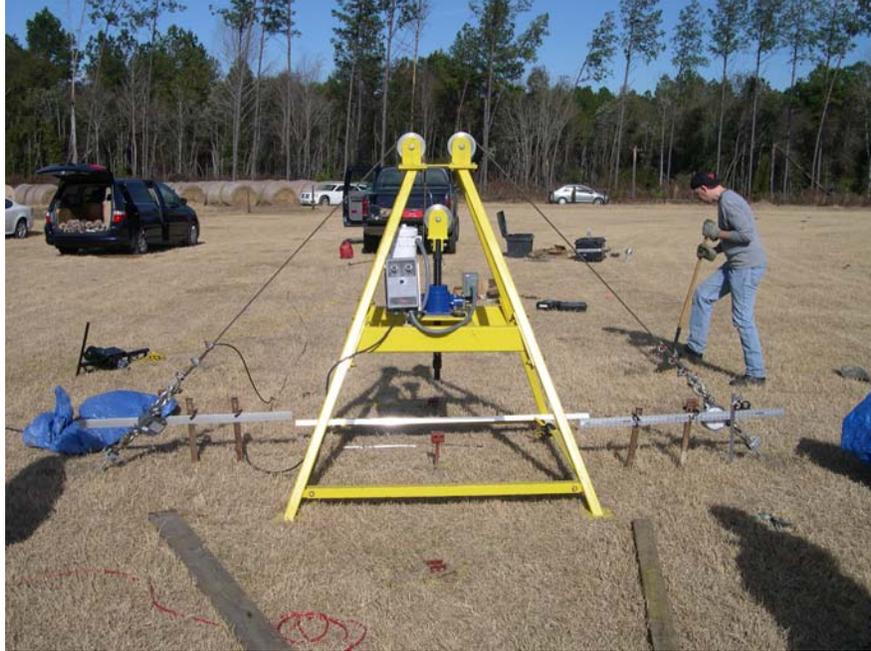
**Figure 2.8.** Angle pull test set-up
