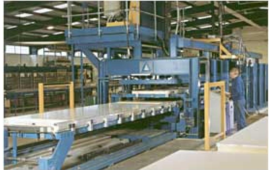
*Plastic honeycomb panels in fabrication*
