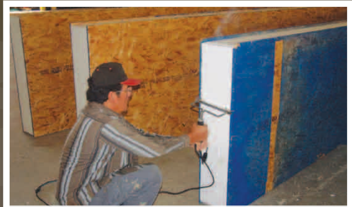
SIPs manufacturing plant worker finishing panels
