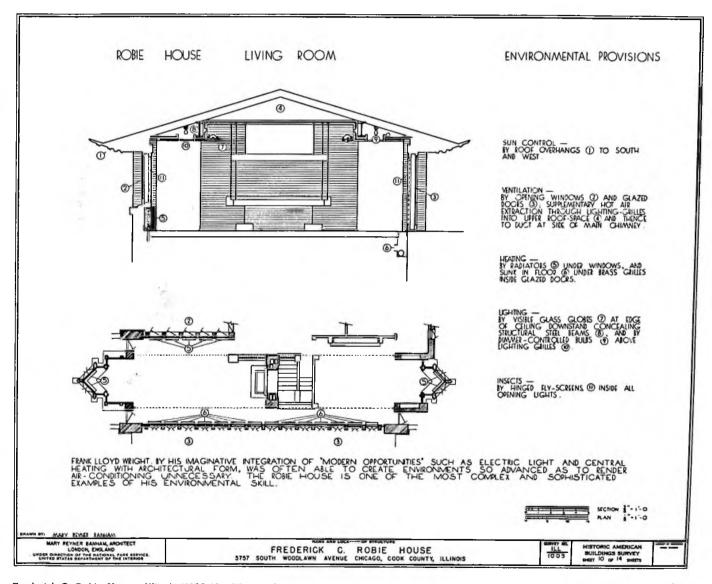
Frederick C. Robie House, Illinois (1908-10). The overhangs are so precisely sized that the midday summer sun just touches the window sills on the south side. The windows and vents are located so that cool air can be drawn up through the house from the basement and exhausted at the ceiling or attic level.
