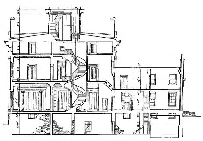
James F. D. Lanier House, Indiana (1840-44). The stairwell serves as an interior lightwell, providing light down through the center of the house. It is lit by a small skylight in the cupola.
