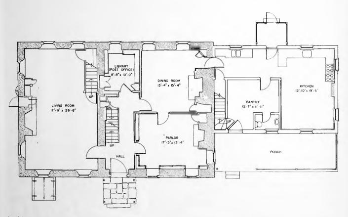
Lundale Farm, Pennsylvania (ca. 1796). The walls of the older sections of this stone furmhouse are about eighteen inches thick with large chimneys set in them. Notice how much thinner the walls are in the 1950 addition and how small the new chimney is. The living room has two other energy saving features, splayed window reveals and a pass-through for firewood next to the chimney.
