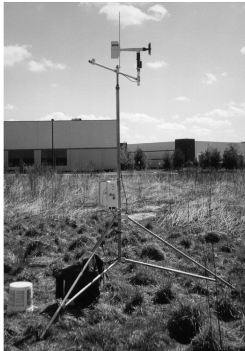
Figure 2 - Portable near-ground wind station with a anemometer at a 10-ft (3-m) height above ground.
