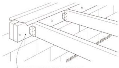
AFTER CUTTING JOISTS BACK TO REMOVE RDT, INSTALL A NEW DOUBLE LEDGER WITH METAL FLASHING
