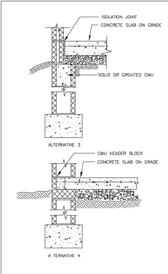
Figure 1-1b: Foundation Stem Wall and Slab on Grade
