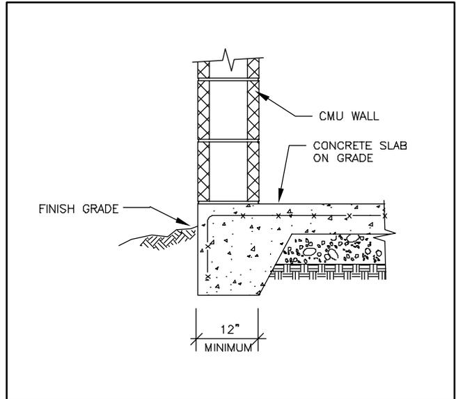
Figure 1-2: Monolithic Slab on Grade (Thickened-Edge Slab)
