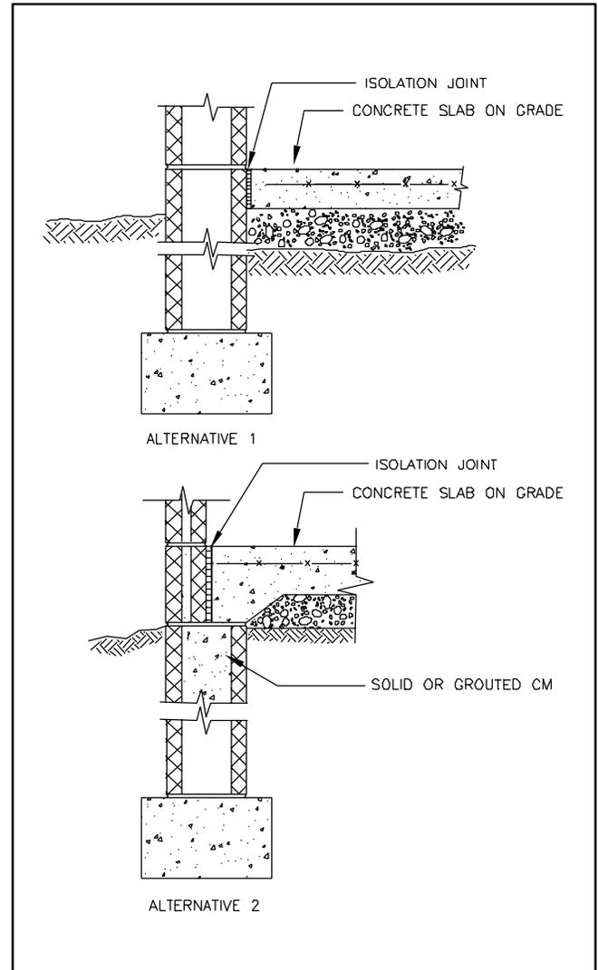
Figure 1-1a: Foundation Stem Wall and Slab on Grade
