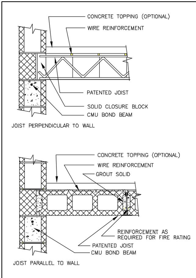
Figure 2-10: Block Joist<sup>®</sup> Floor System
