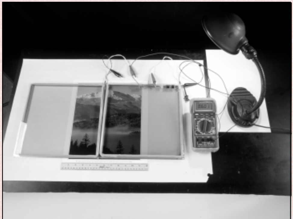
Mid-sized photoelectrochromic window turning dark under a voltage applied by two small PV cells attached to the side of the window.
