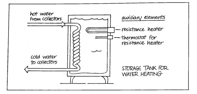
The principles of this temperature stratification are often poorly understood or misused. The importance of stratification is relative to the size of the system. In current computer design programs, only TRNSYS takes stratification into account.
