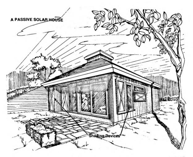
Don't make unrealistic assumptions about the owner's participation in operating the movable insulation or shading devices. The operation of one system depended on the owner to lift out and store twelve separate insulating panels in the morning and to replace them again at night. This is one area where mechanical controls could have been used.
