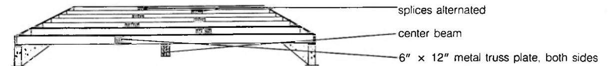
Note: Use lumber with minimum E = 1,400,000 and F = 1,150 (repetitive member). Use glue-nailed plywood floor.
