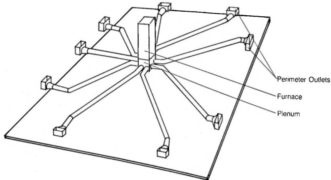
Figure 34. Typical Radial Duct System
