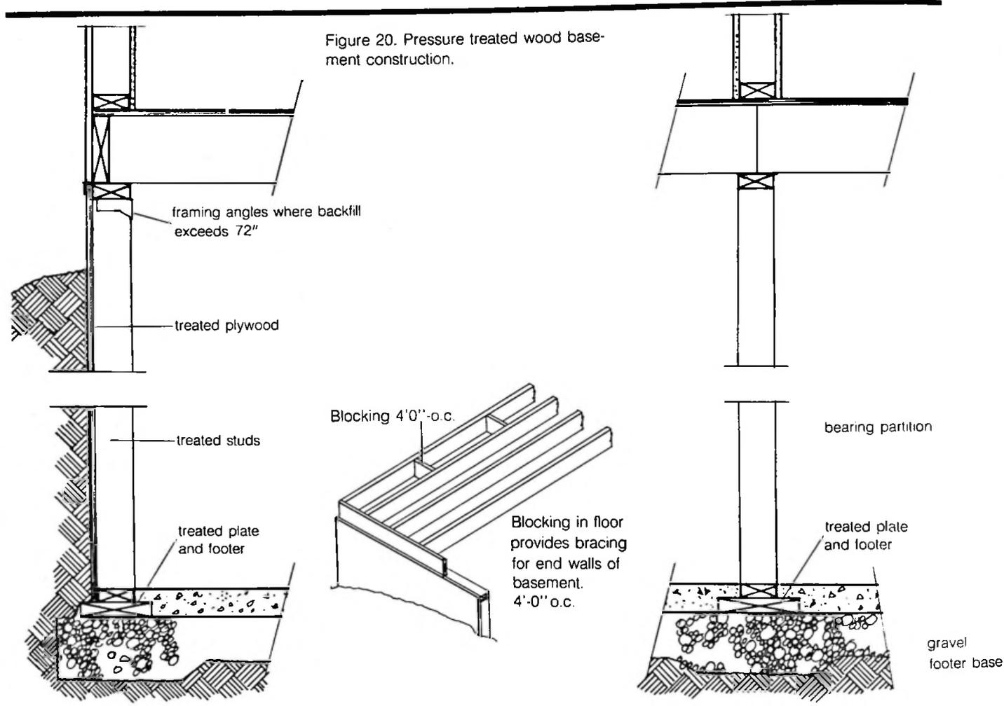
Figure 20. Pressure treated wood basement construction.
