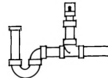
Figure 32. Typical Automatic Vent
