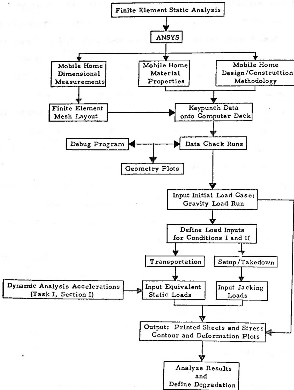
FIGURE 1. FINITE ELEMENT COMPUTER MODEL DEVELOPMENT AND ANALYSIS
