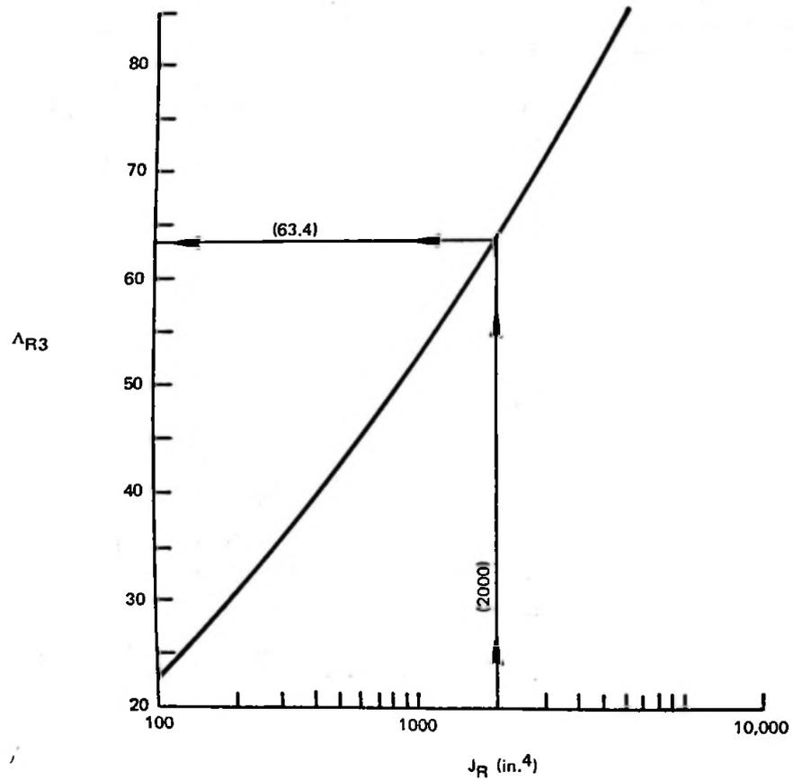
FIGURE 2. EFFECT OF TORSIONAL STIFFNESS ON DYNAMIC RESPONSE PARAMETER
