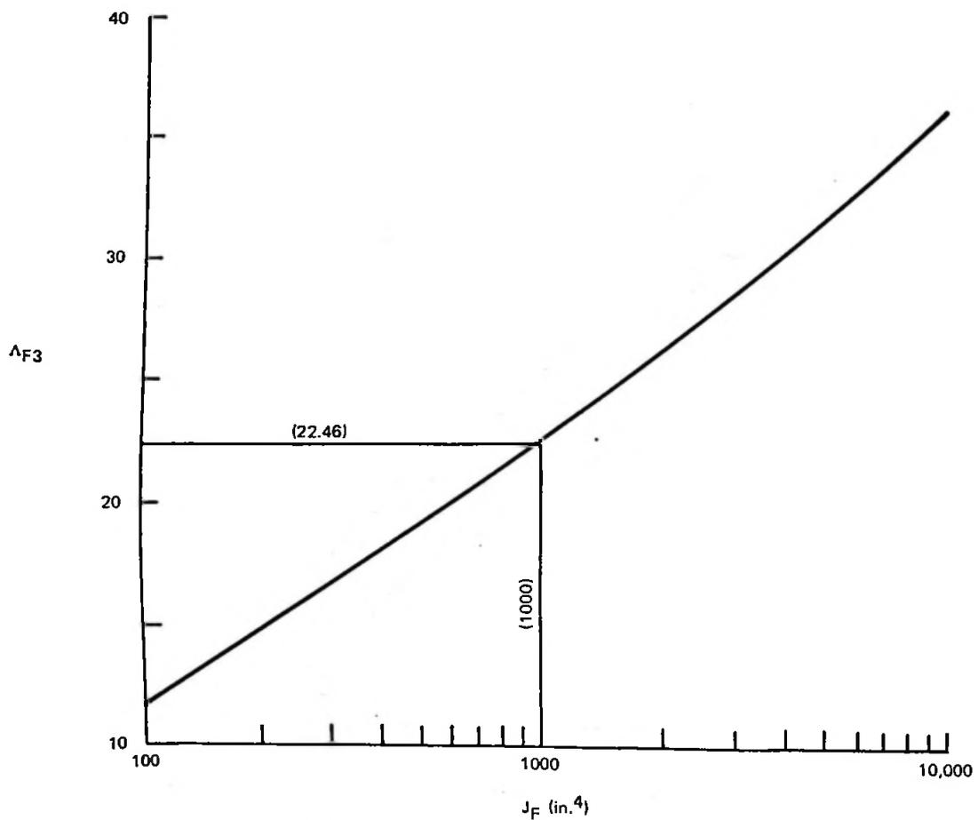
FIGURE 6. EFFECT OF TORSIONAL STIFFNESS ON DYNAMIC RESPONSE PARAMETER
