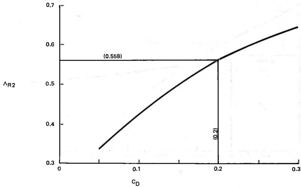
FIGURE 3. EFFECT OF DAMPING ON DYNAMIC RESPONSE PARAMETER
