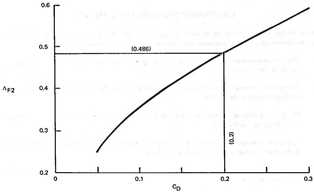
FIGURE 7. EFFECT OF DAMPING ON DYNAMIC RESPONSE PARAMETER
