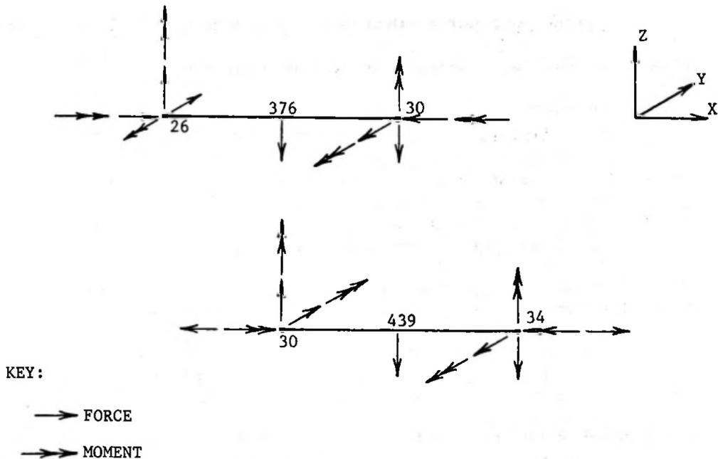
FIGURE B.2. FREE BODY DIAGRAMS OF ELEMENTS 376 AND 439
