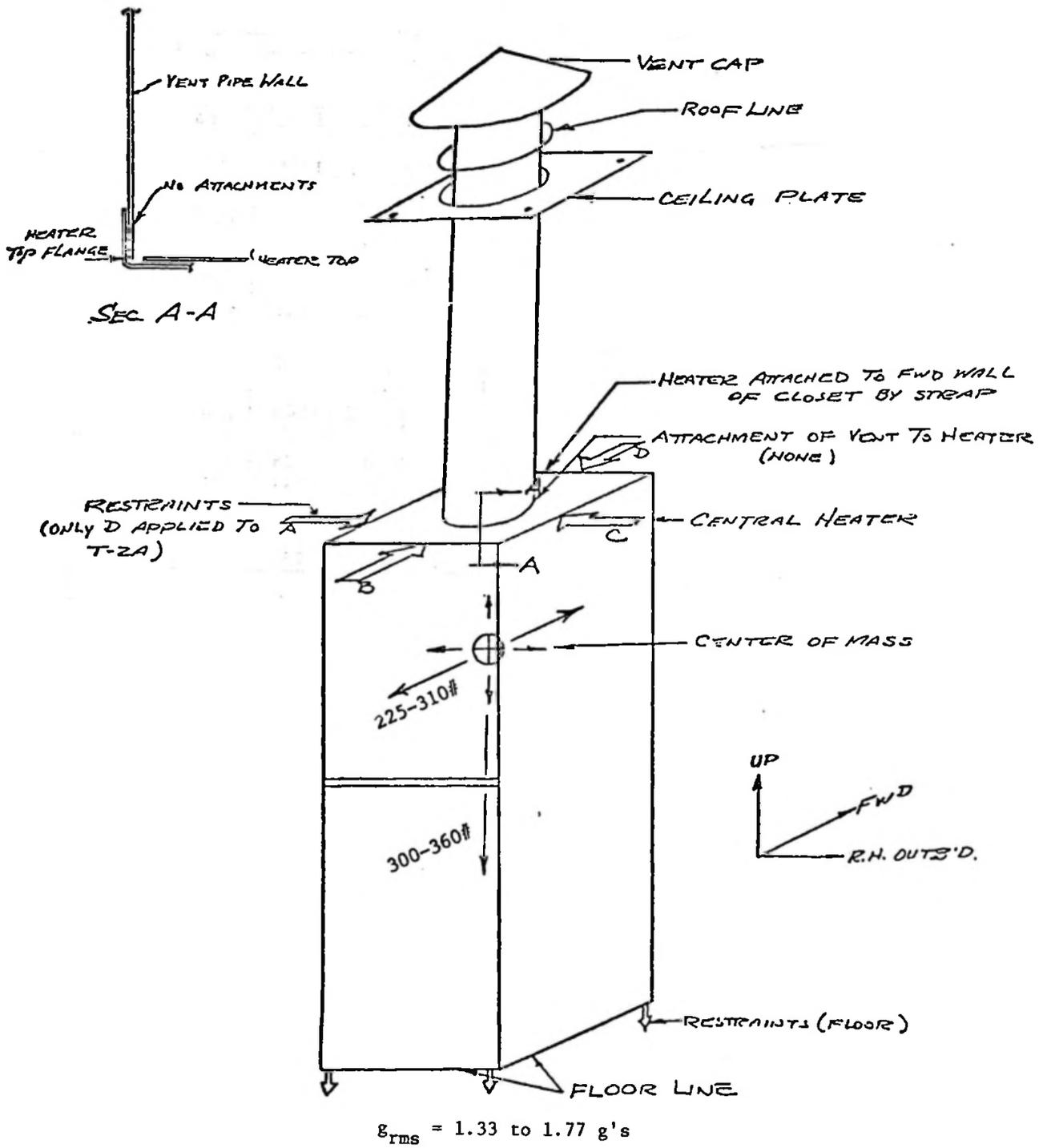
FIGURE 68. T-2A (WET SIDE) DOUBLE-WIDE - CENTRAL HEATER VENT
