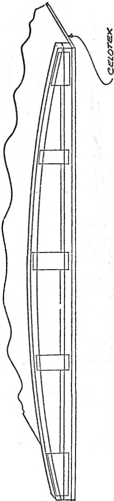
The celotex was not considered as a structural component in the development of the finite element analytical model.
