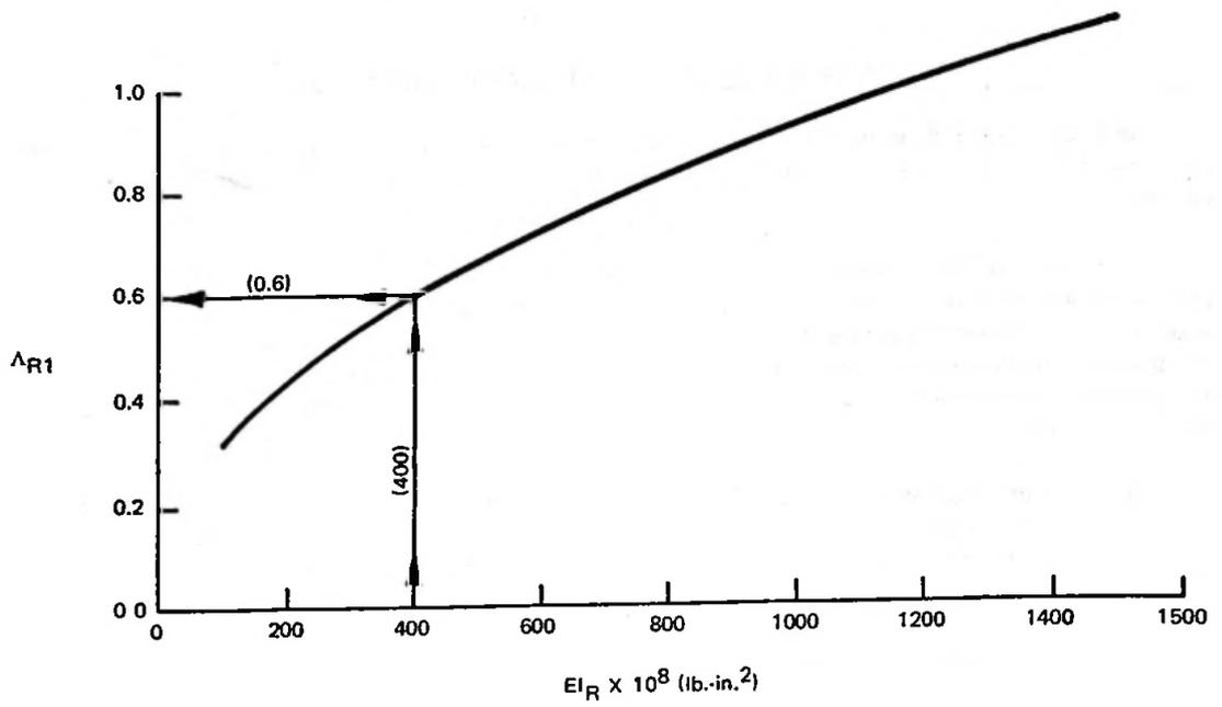
FIGURE 1. EFFECT OF FLEXURAL STIFFNESS ON DYNAMIC RESPONSE PARAMETER
