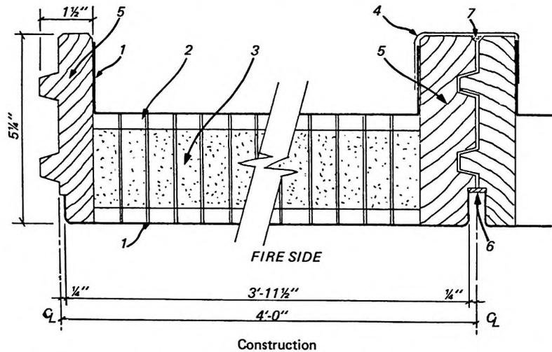
1. 26 ga sheet steel facing bonded to honeycomb core with epoxy adhesive. Steel sheets were galvanized, phosphatized and finished on exterior surfaces with a baked on silicone paint.
