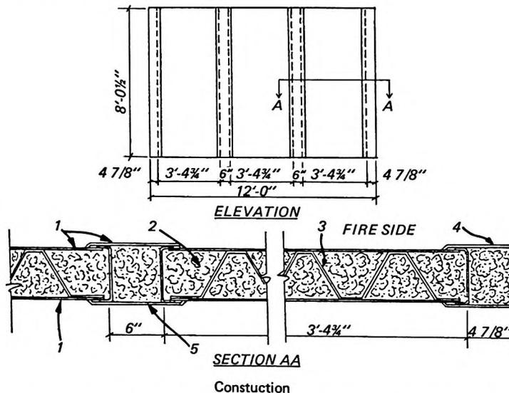
1. 0.080-in thick glass fiber reinforced polyester laminate bonded to stiffeners with adhesive.
