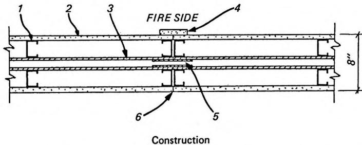
1. 2 1/2 by 1 5/8-in 18 ga steel "C" studs, 24 in o. c.
