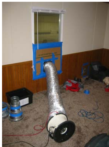
Figure 2-13 Fan simulating clothes dryer exhaust
