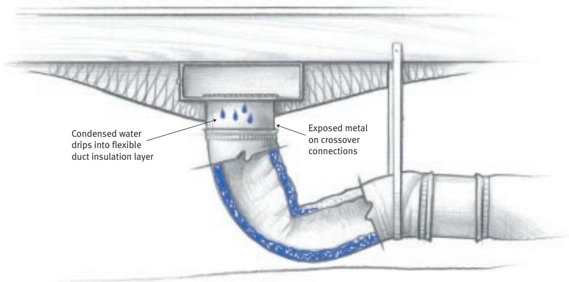
Exposed metal on crossover connections condenses water that can seep into the flexible duct insulation layer. The water builds up until its weight kinks the flexible duct, restricting airflow.
