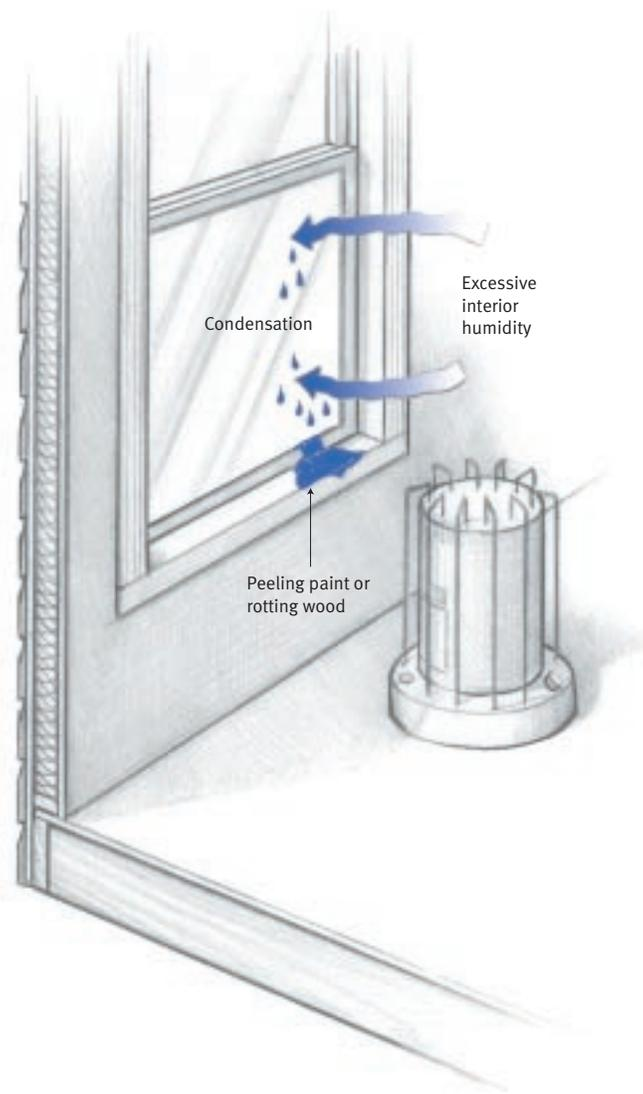
In winter, excessive interior humidity causes water to condense and run down inside the surface of the window glass and damage the sill. Unvented combustion space heaters that give off a good deal of moisture are sometimes the culprit.
