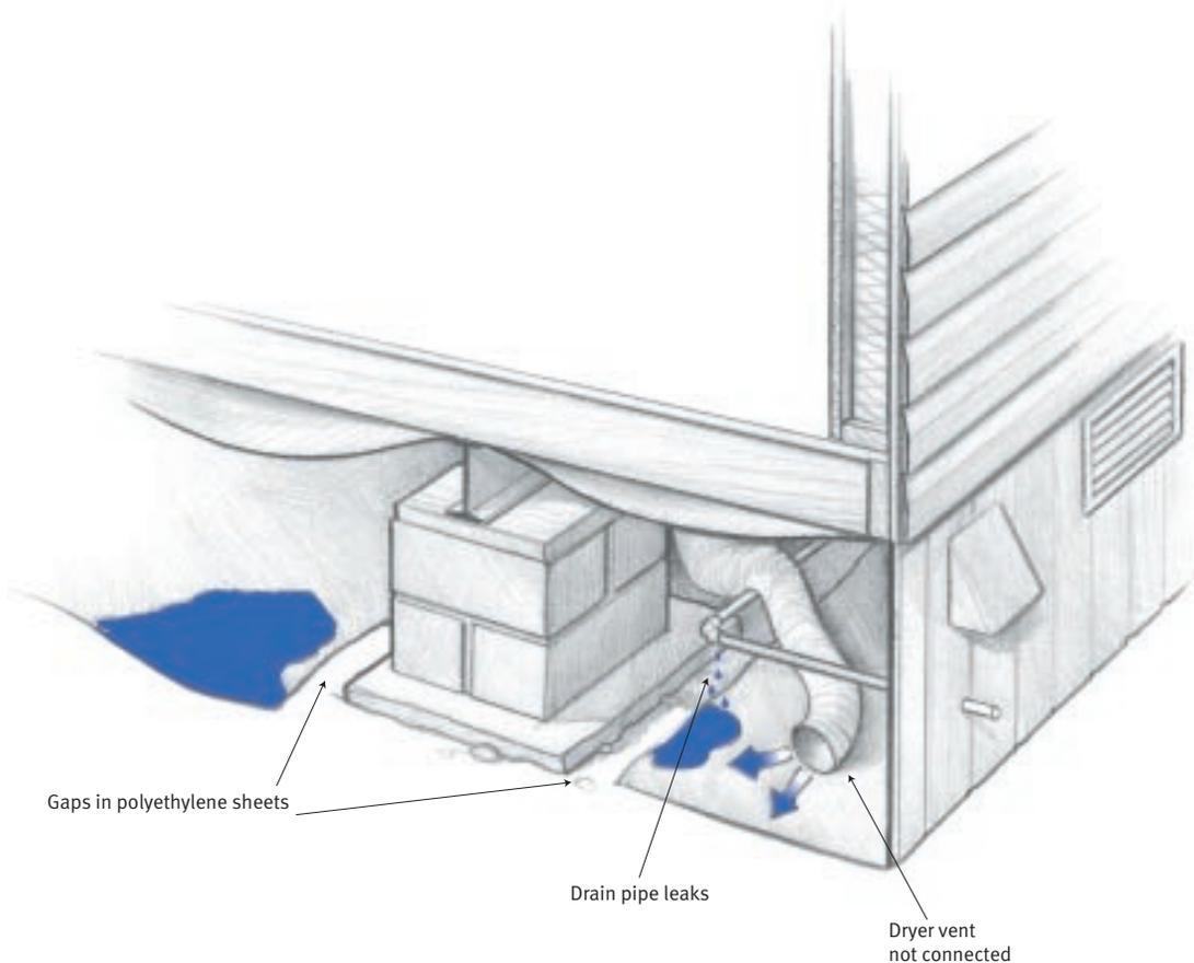
Crawlspaces are a major source of moisture. To keep the crawlspace dry, cover the ground with a continuous polyethylene sheet and install properly sized skirting vents. The dryer should vent and the condensate line should drain to the outside.
