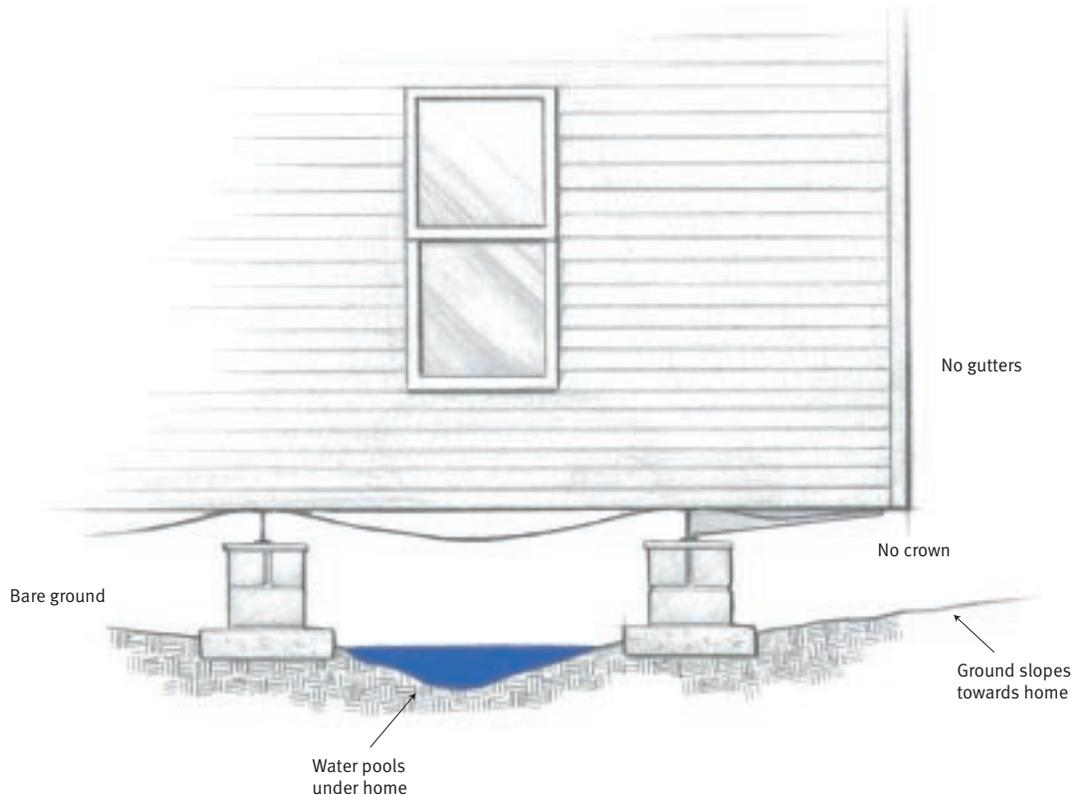
A properly graded site has a crown underneath the home and sloping ground that carries water away from the house, unlike the poor grading job shown above. Gutters and downspouts prevent splash back and direct water away from the foundation. Ground should be covered with a polyethelene sheet.
