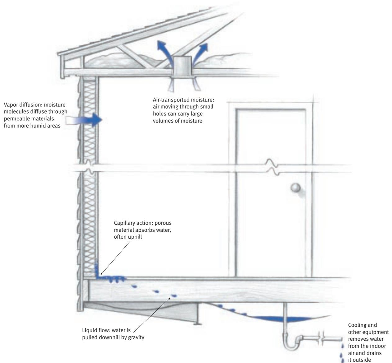
Water moves from one place to another via liquid flow, capillary action, vapor diffusion, air movement, and equipment operation.
