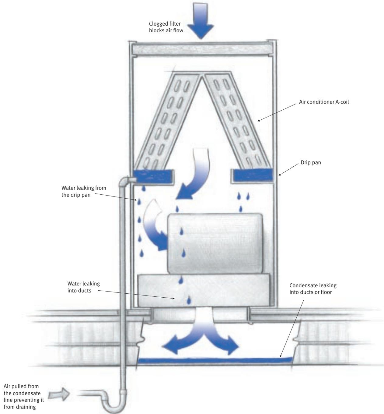
A clogged air conditioner filter blocks return airflow, and the "starved" air handler fan sucks water out of the drain line. Water spills into the air handler cabinet, leaking into ducts and seeping into the floor.
