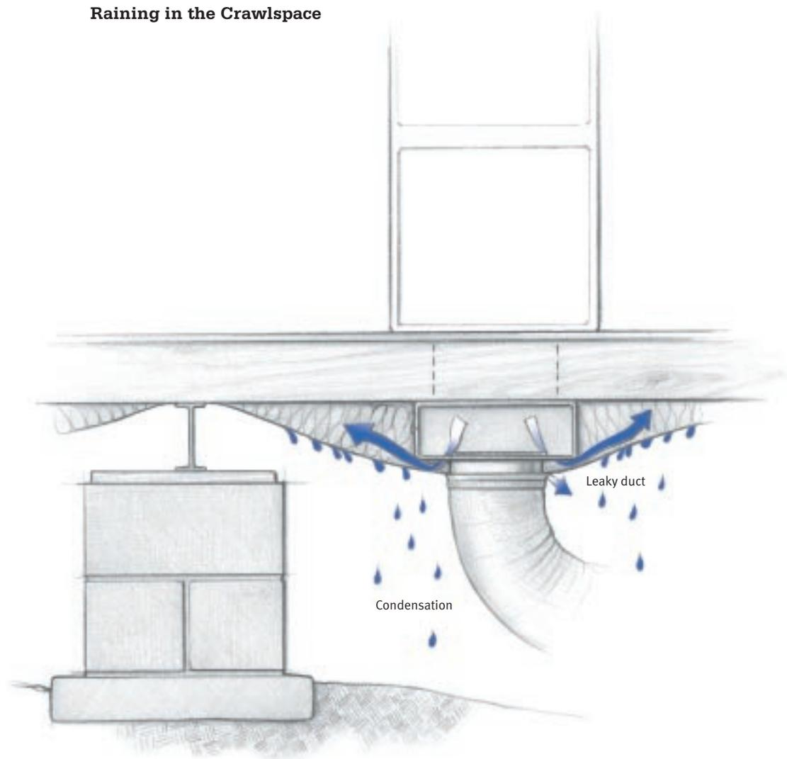
Duct leaks can cause water to "rain" into the crawlspace. Cold air that leaks from the underfloor duct system cools the belly material, supporting the condensation.
