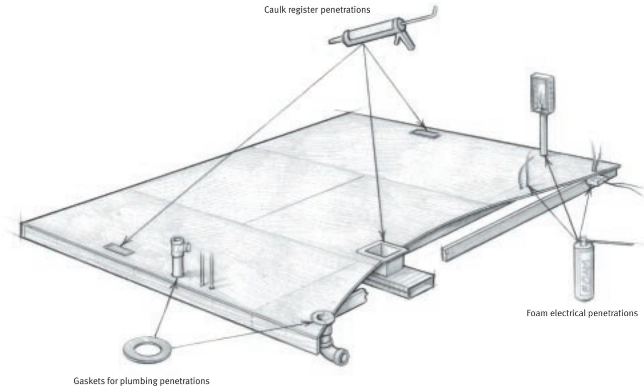
The floor is a natural moisture and air barrier. Keep it intact by sealing all floor penetrations with the appropriate sealant or gasket.
