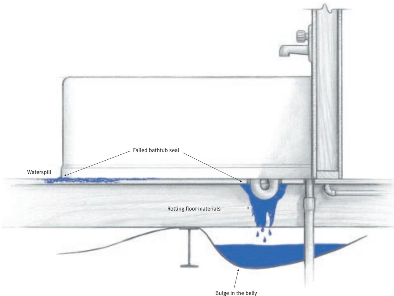
When seals around tubs fail, water drains into the floor cavity and pools on the bottom board. Unchecked, the leaks can rot out floor materials.
