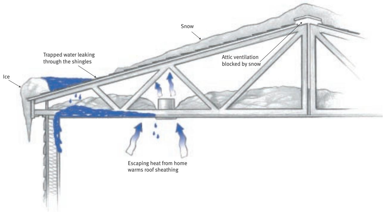
Ice dams occur when attic insulation is insufficient or warm home air enters the attic space. Melting snow or ice on the roof surface backs up and seeps through the shingles into the roof cavity, damaging materials and reducing insulation values.
