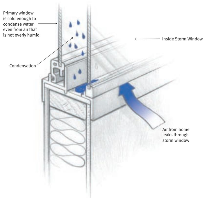
Pressure imbalance in a house will push warm air through leaks in the interior window allowing moisture to condense between the two panes of glass. A durable seal should be applied to the storm window to minimize leaks.
