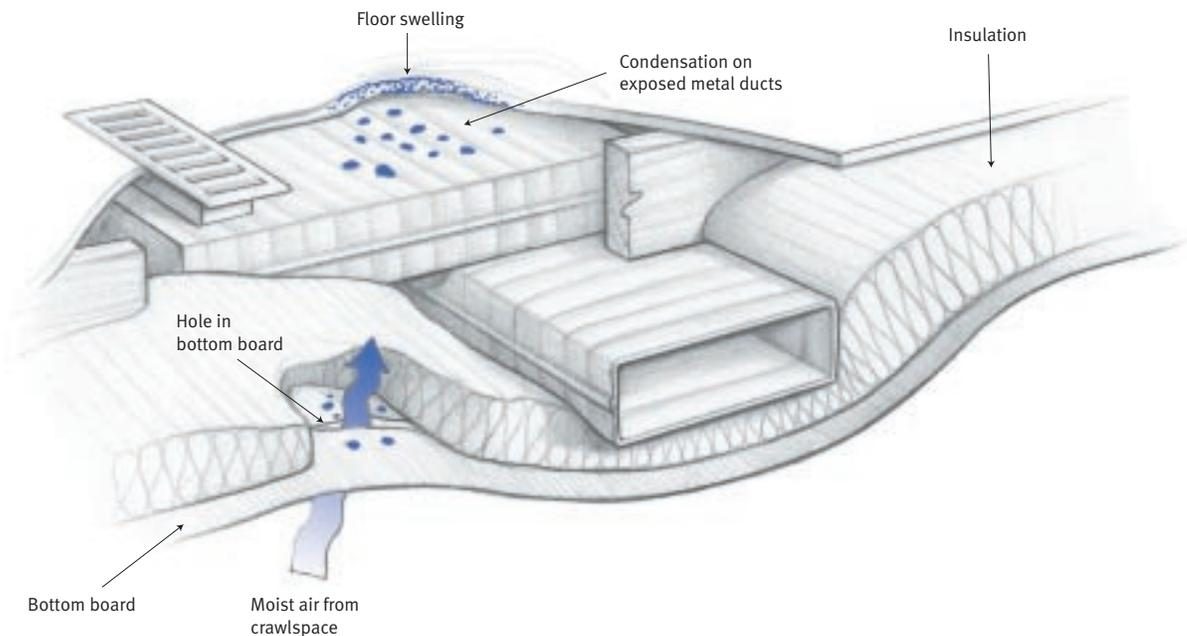
Warping of the floor sheathing can occur when a hole in the bottom board allows moist crawlspace air to condense on exposed metal ducts. Water is absorbed by the floor sheathing, which swells.
