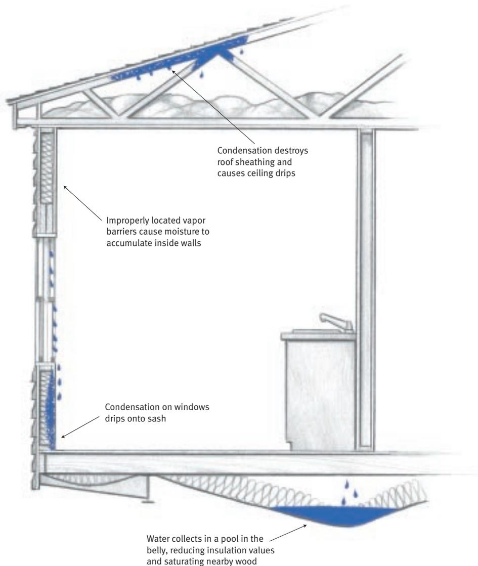
Moisture in a home becomes a problem only when it stops moving and accumulates in damaging amounts.
