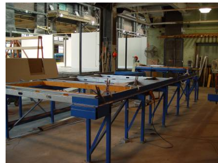
Figure 44 Wall framing station
