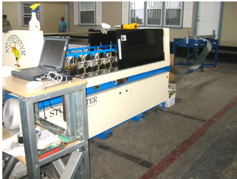
Figure 2-5 Steel studs and other components are produced in the plant
