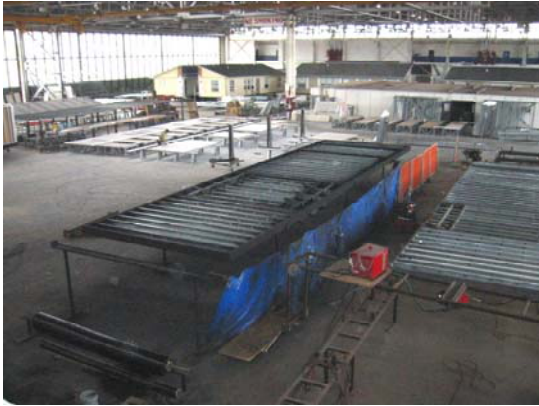
Figure 2-3 Steel chassis being welded on the production line
