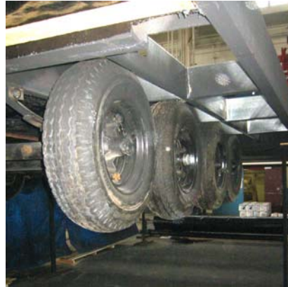
Figure 2-4 Tires are inset into the chassis
