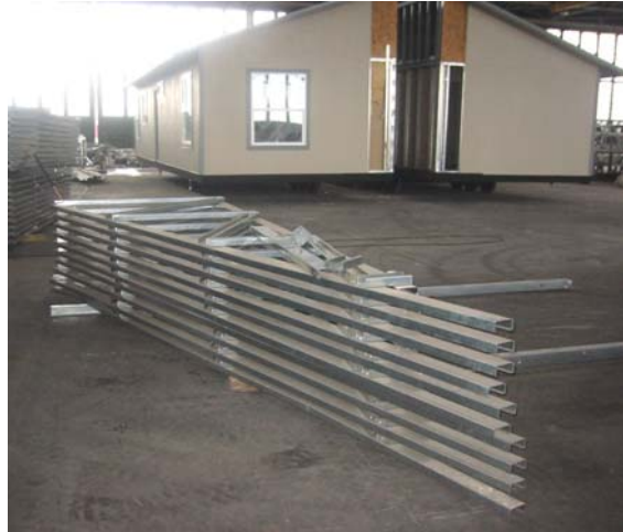
Figure 2-19 Trusses and assembled home sections
