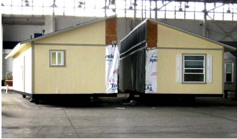
Figure 2-13 Home sections in the finishing station
