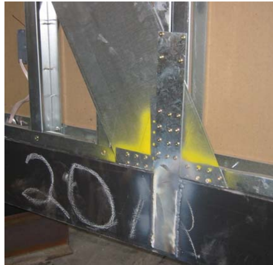
Figure 2-12 Cross-brace connection detail
