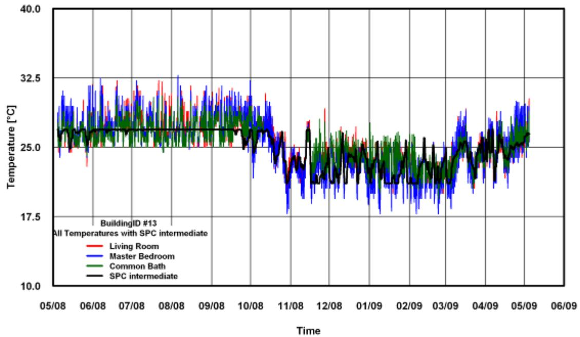
Figure 291: Temperature of SPC 160 Intermediate ANK Modified Method for Building # 13
