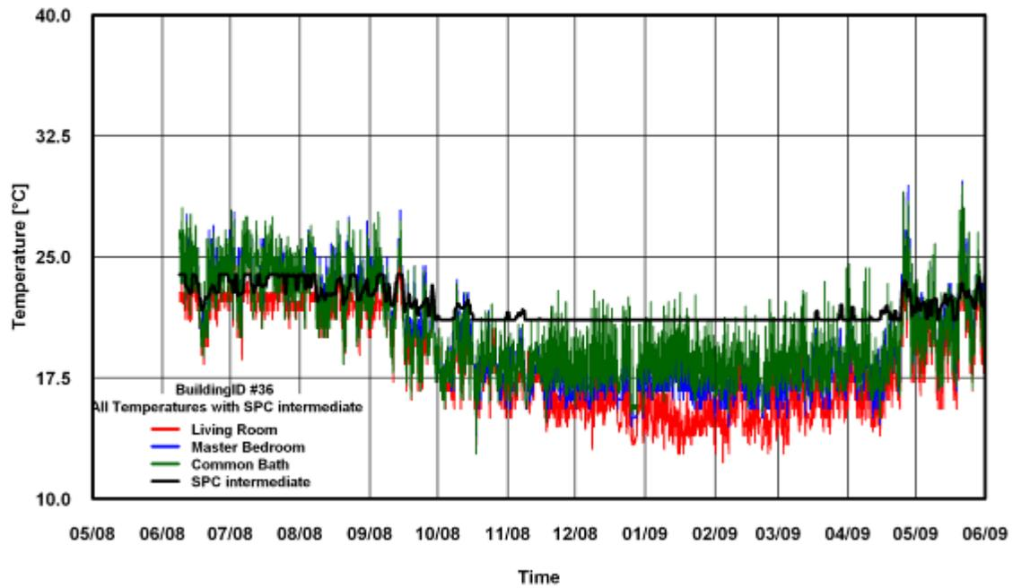
Figure 217: Temperature of SPC 160 Intermediate Method for Building # 36
