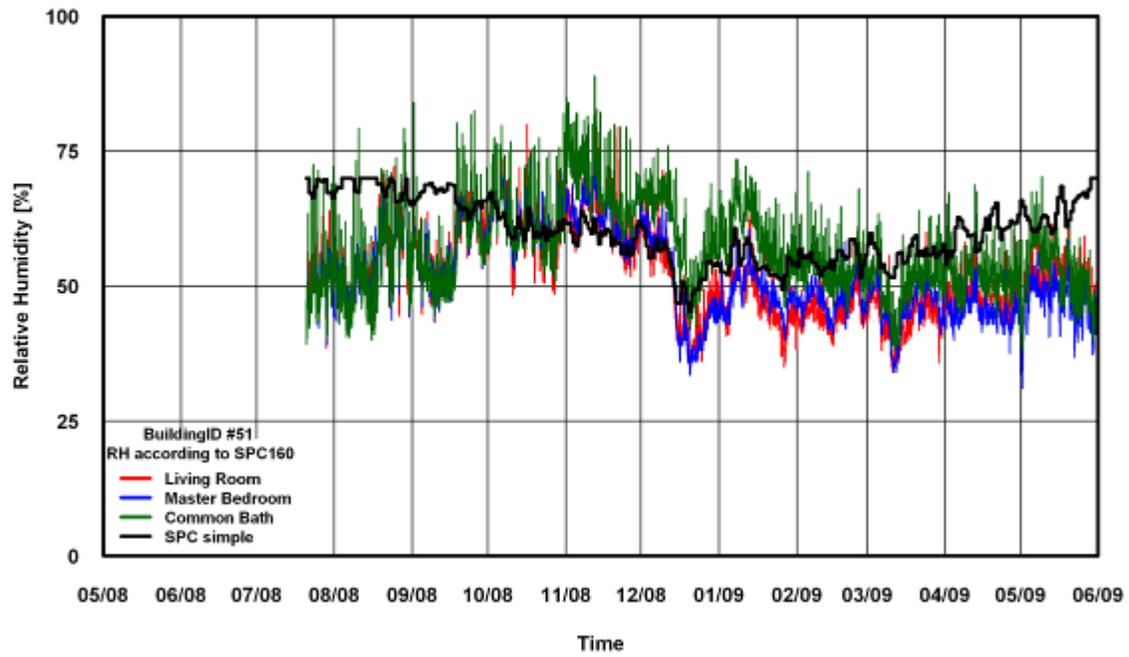
Figure 124: RH Comparison of SPC 160 Simple Method for Building # 51
