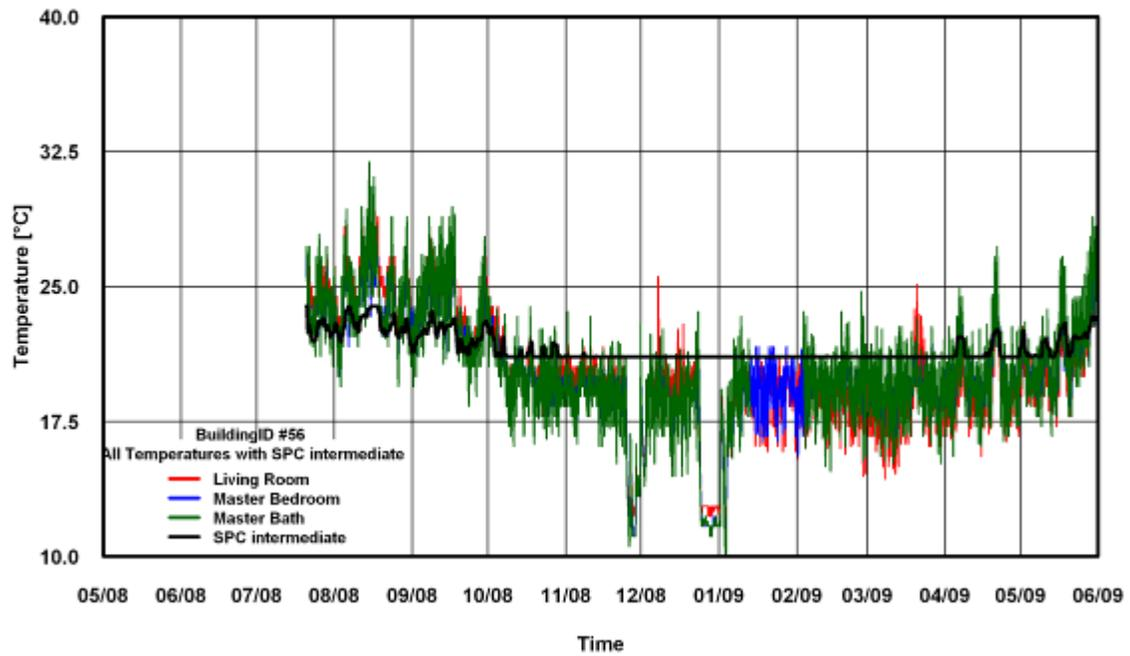
Figure 255: Temperature of SPC 160 Intermediate Method for Building # 56
