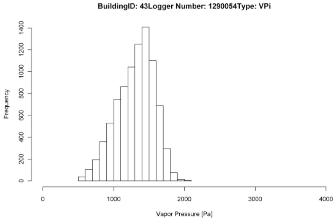
Figure 20: Frequency Plot for the Interior Vapor Pressure (Pa) for House 43
