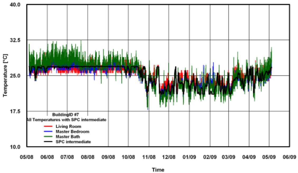
Figure 279: Temperature of SPC 160 Intermediate ANK Modified Method for Building # 7
