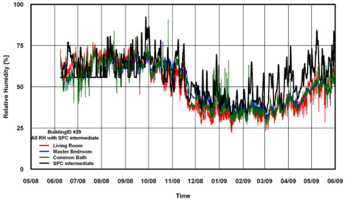
Figure 202: RH Comparison of SPC 160 Intermediate Method for Building # 29
