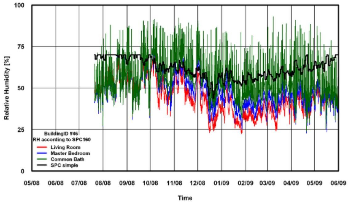
Figure 114: RH Comparison of SPC 160 Simple Method for Building # 46
