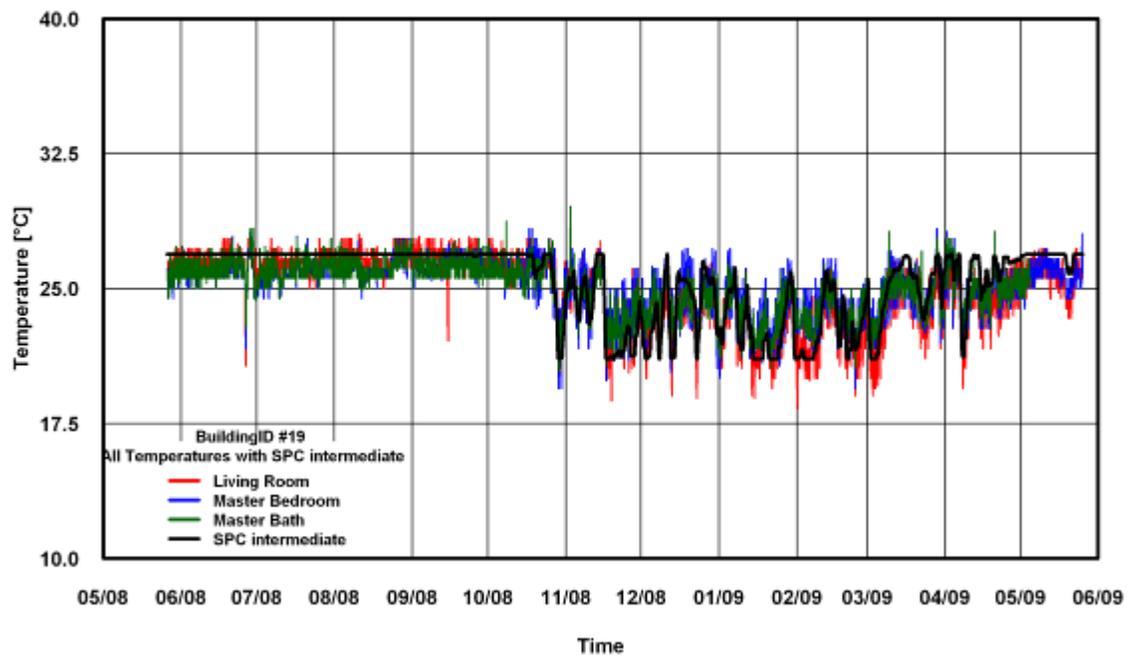
Figure 303: Temperature of SPC 160 Intermediate ANK Modified Method for Building # 19
