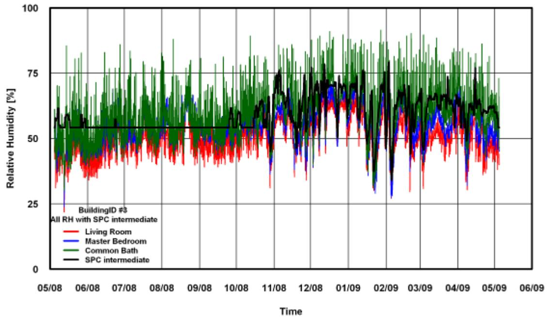
Figure 270: RH Comparison of SPC 160 Intermediate ANK Modified Method for Building # 3
