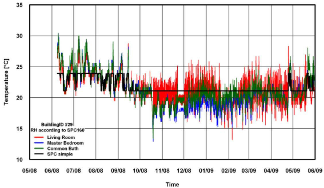
Figure 83: Temperature Comparison of SPC 160 Simple Method for Building # 29
