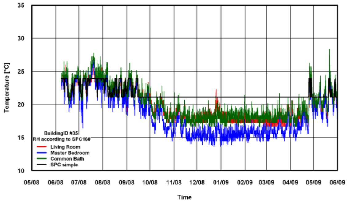
Figure 95: Temperature Comparison of SPC 160 Simple Method for Building # 35
