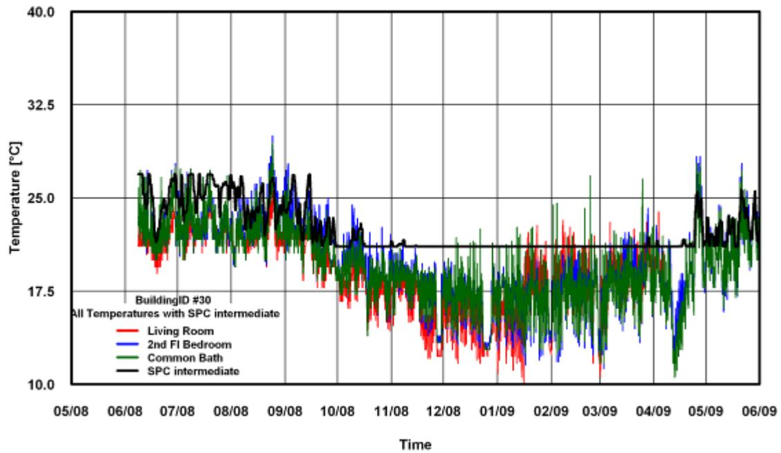
Figure 325: Temperature of SPC 160 Intermediate ANK Modified Method for Building # 30
