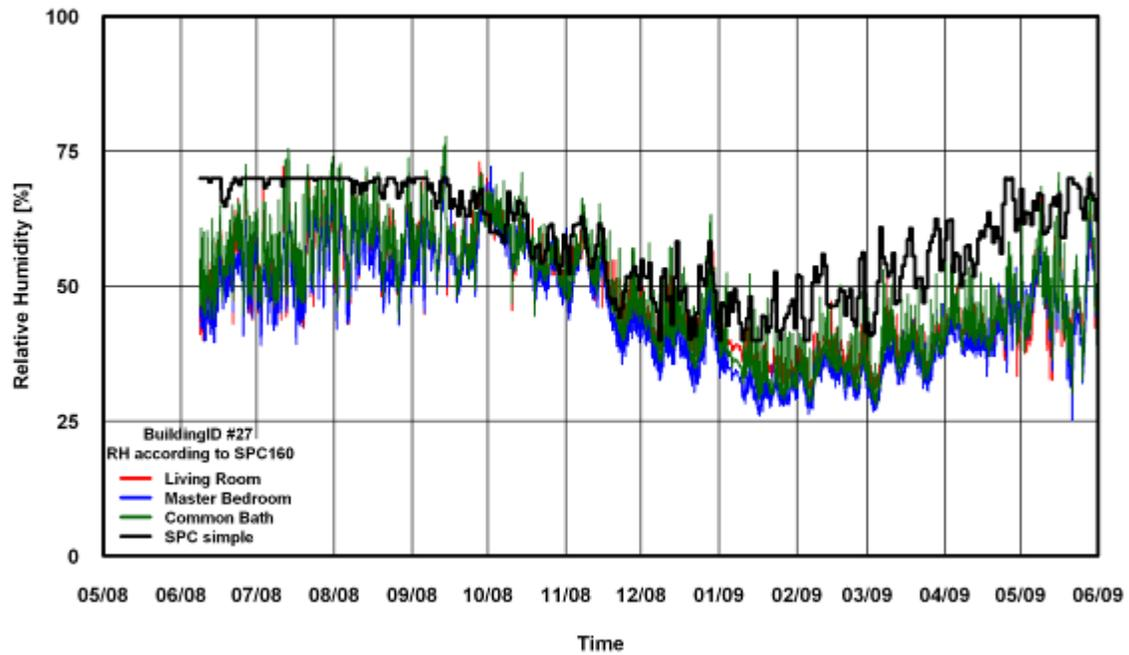
Figure 78: RH Comparison of SPC 160 Simple Method for Building # 27
