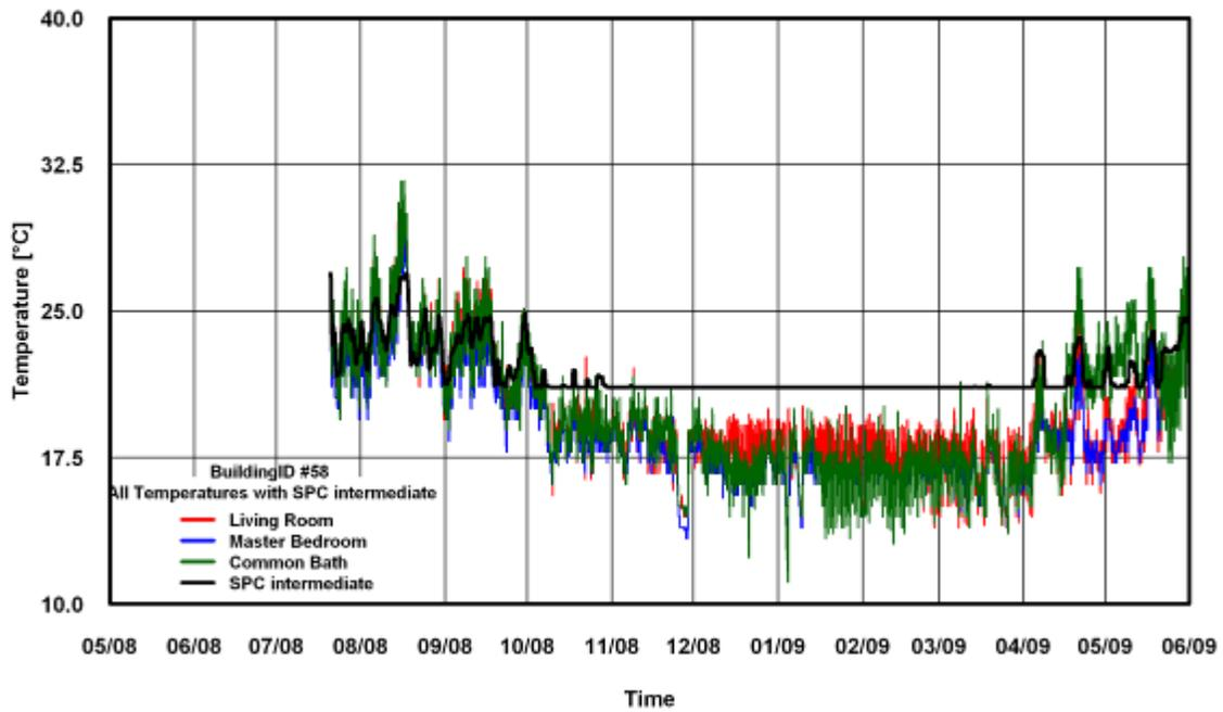
Figure 379: Temperature of SPC 160 Intermediate ANK Modified Method for Building # 58
