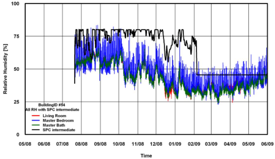
Figure 370: RH Comparison of SPC 160 Intermediate ANK Modified Method for Building # 54
