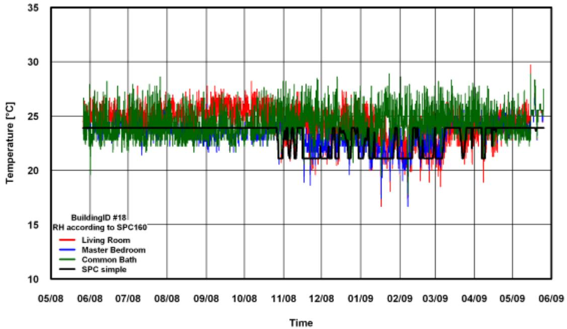
Figure 61: Temperature Comparison of SPC 160 Simple Method for Building # 18
