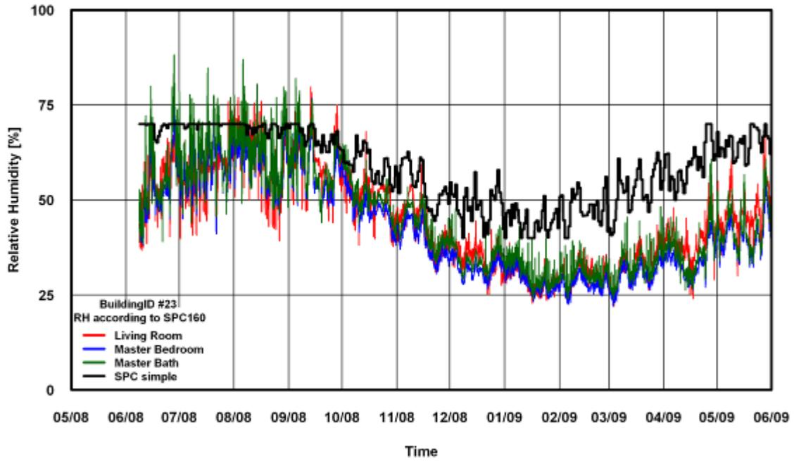
Figure 70: RH Comparison of SPC 160 Simple Method for Building # 23
