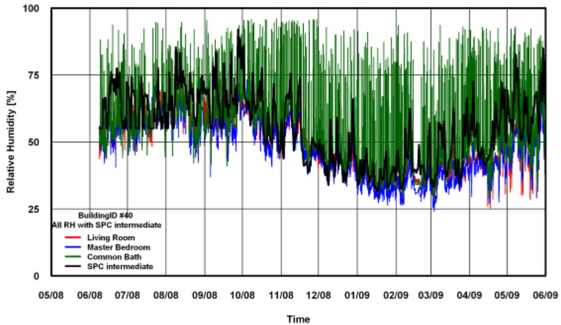
Figure 224: RH Comparison of SPC 160 Intermediate Method for Building # 40
