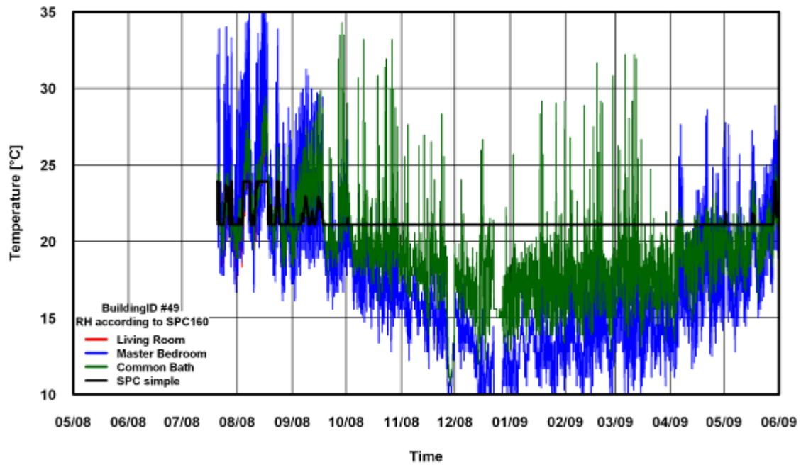
Figure 121: Temperature Comparison of SPC 160 Simple Method for Building # 49
