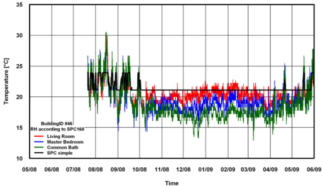
Figure 115: Temperature Comparison of SPC 160 Simple Method for Building # 46
