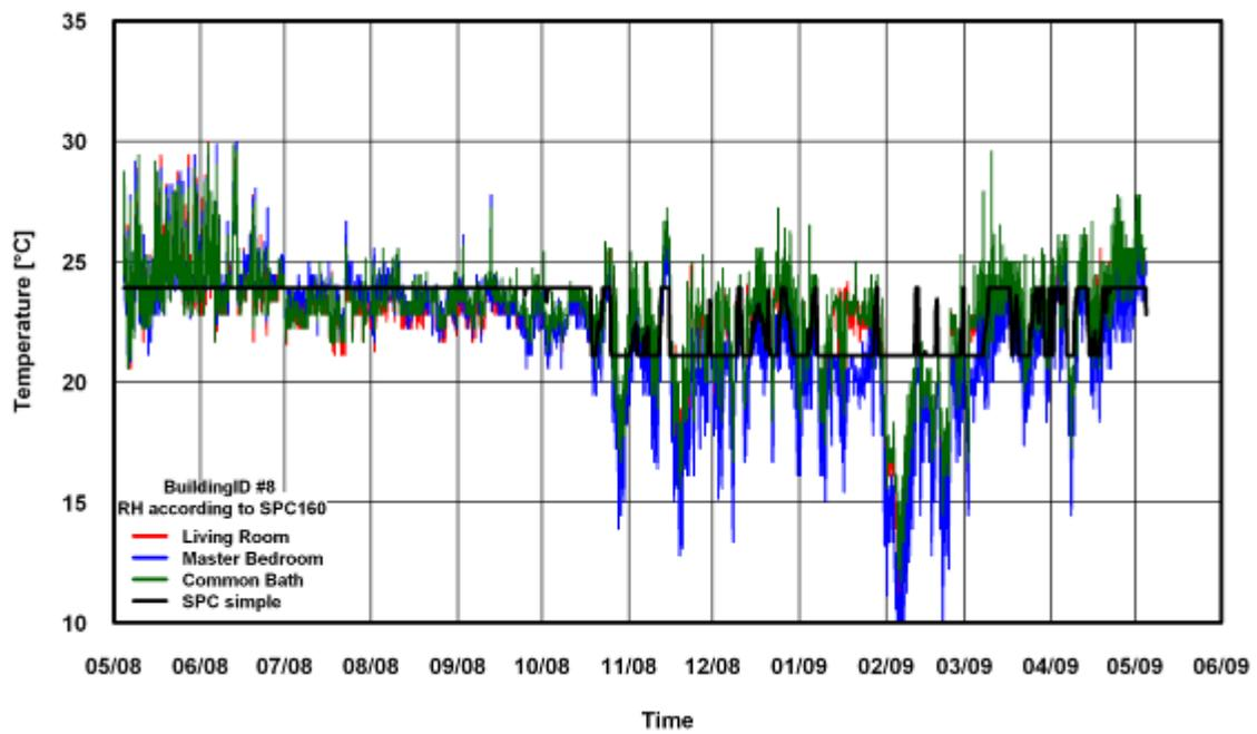
Figure 41: Temperature Comparison of SPC 160 Simple Method for Building # 8
