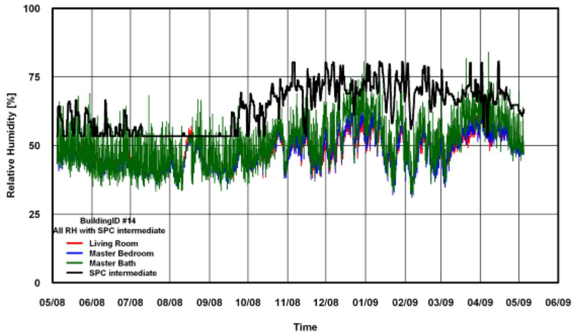
Figure 292: RH Comparison of SPC 160 Intermediate ANK Modified Method for Building # 14
