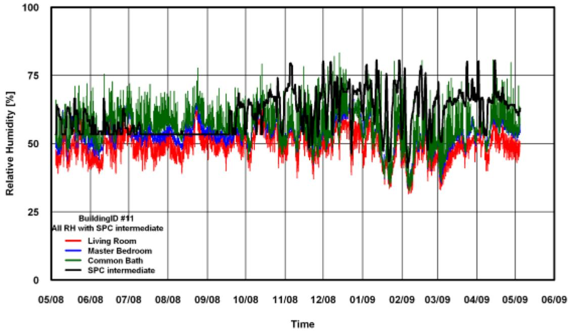
Figure 286: RH Comparison of SPC 160 Intermediate ANK Modified Method for Building # 11
