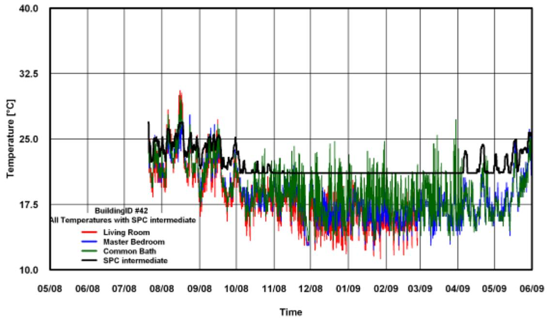
Figure 347: Temperature of SPC 160 Intermediate ANK Modified Method for Building # 42
