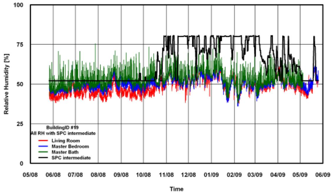
Figure 302: RH Comparison of SPC 160 Intermediate ANK Modified Method for Building # 19
