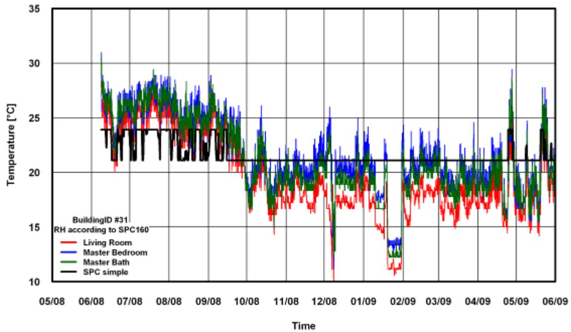
Figure 87: Temperature Comparison of SPC 160 Simple Method for Building # 31
