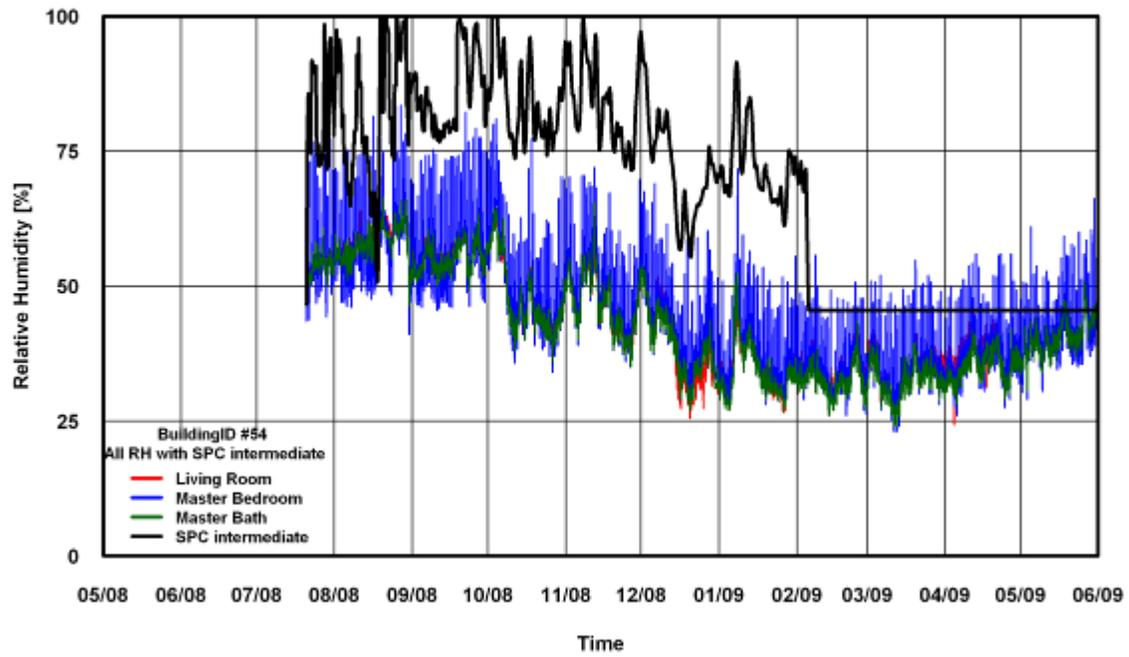
Figure 250: RH Comparison of SPC 160 Intermediate Method for Building # 54
