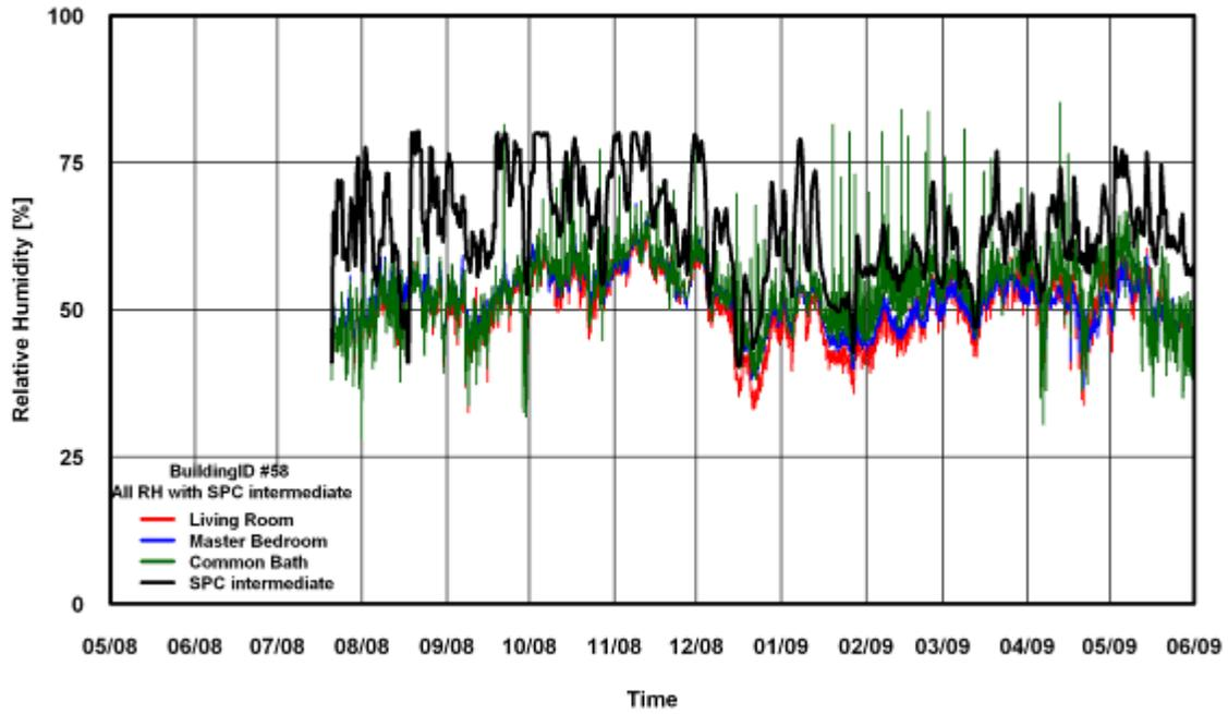
Figure 378: RH Comparison of SPC 160 Intermediate ANK Modified Method for Building # 58
