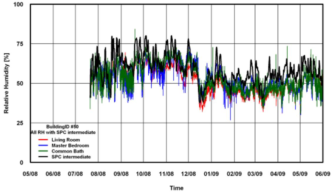
Figure 362: RH Comparison of SPC 160 Intermediate ANK Modified Method for Building # 50
