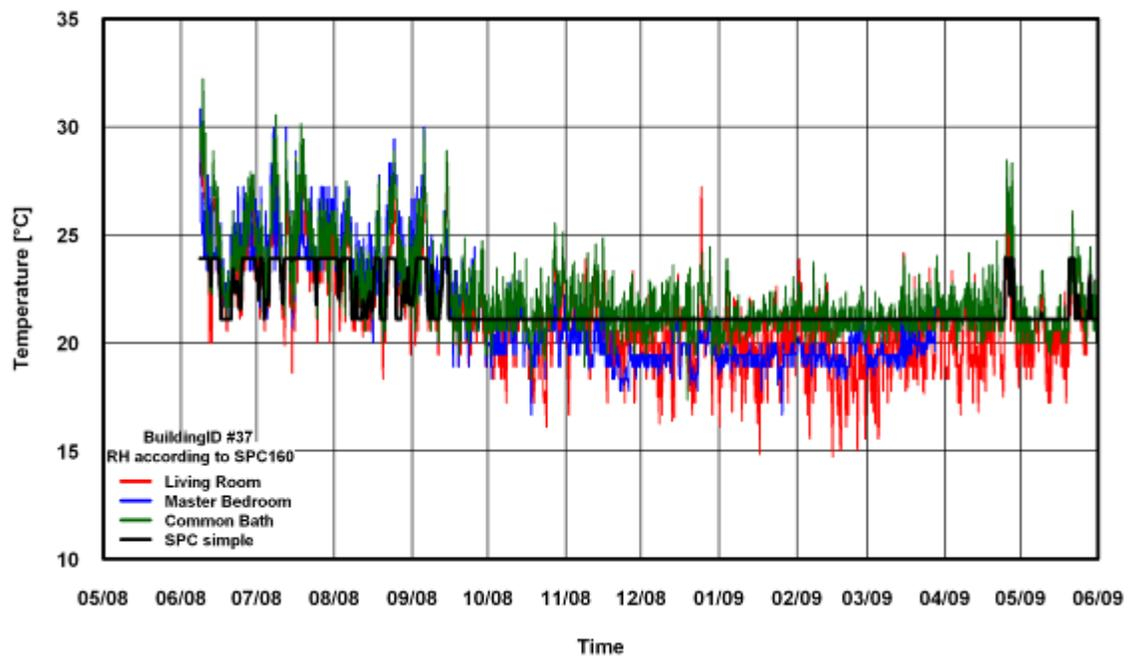
Figure 99: Temperature Comparison of SPC 160 Simple Method for Building # 37
