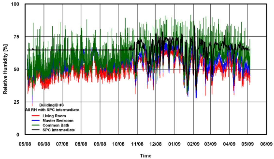
Figure 150: RH Comparison of SPC 160 Intermediate Method for Building # 3
