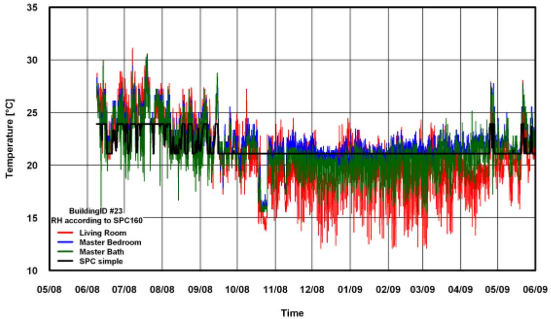
Figure 71: Temperature Comparison of SPC 160 Simple Method for Building # 23
