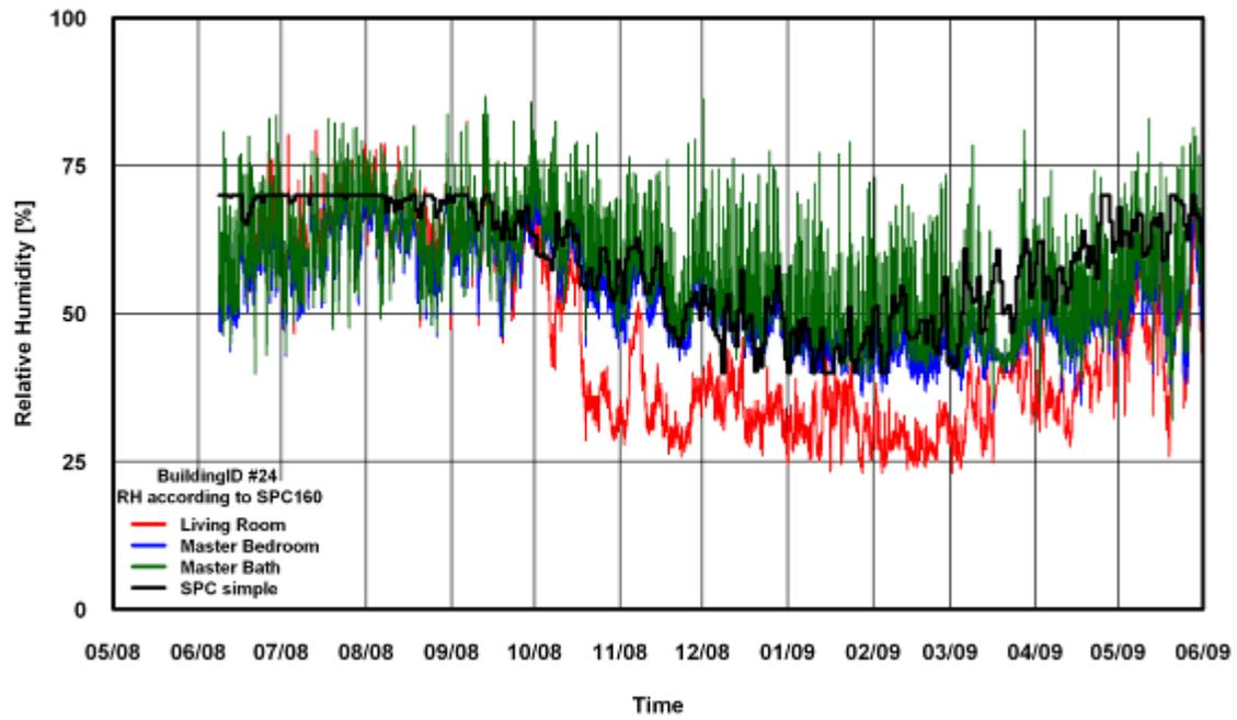
Figure 72: RH Comparison of SPC 160 Simple Method for Building # 24
