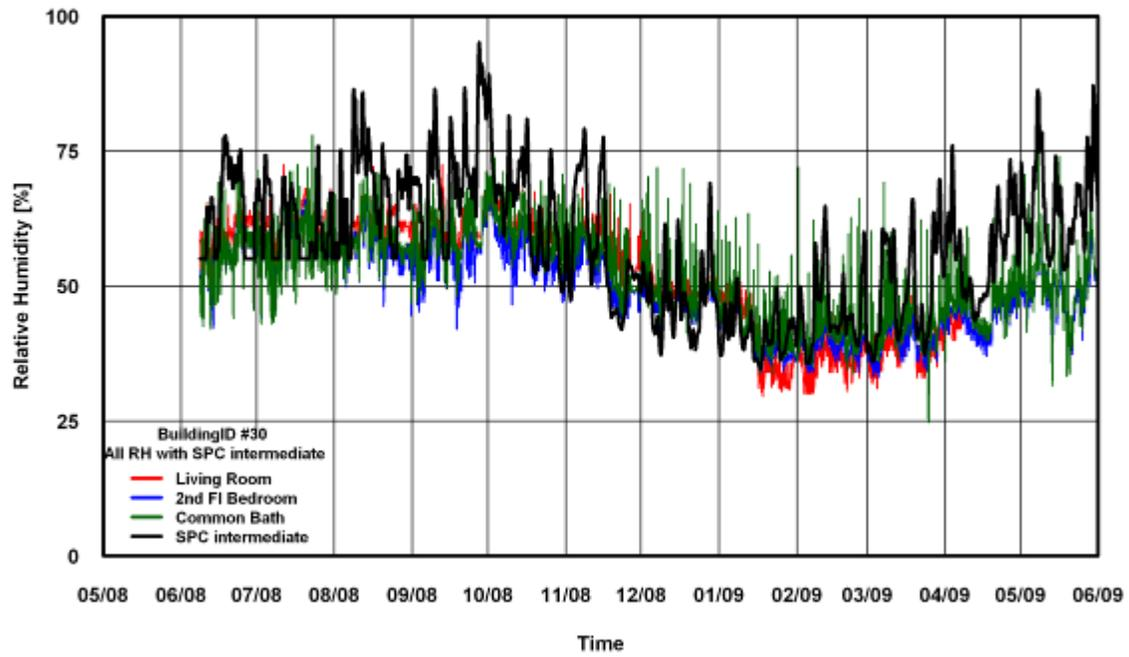
Figure 204: RH Comparison of SPC 160 Intermediate Method for Building # 30
