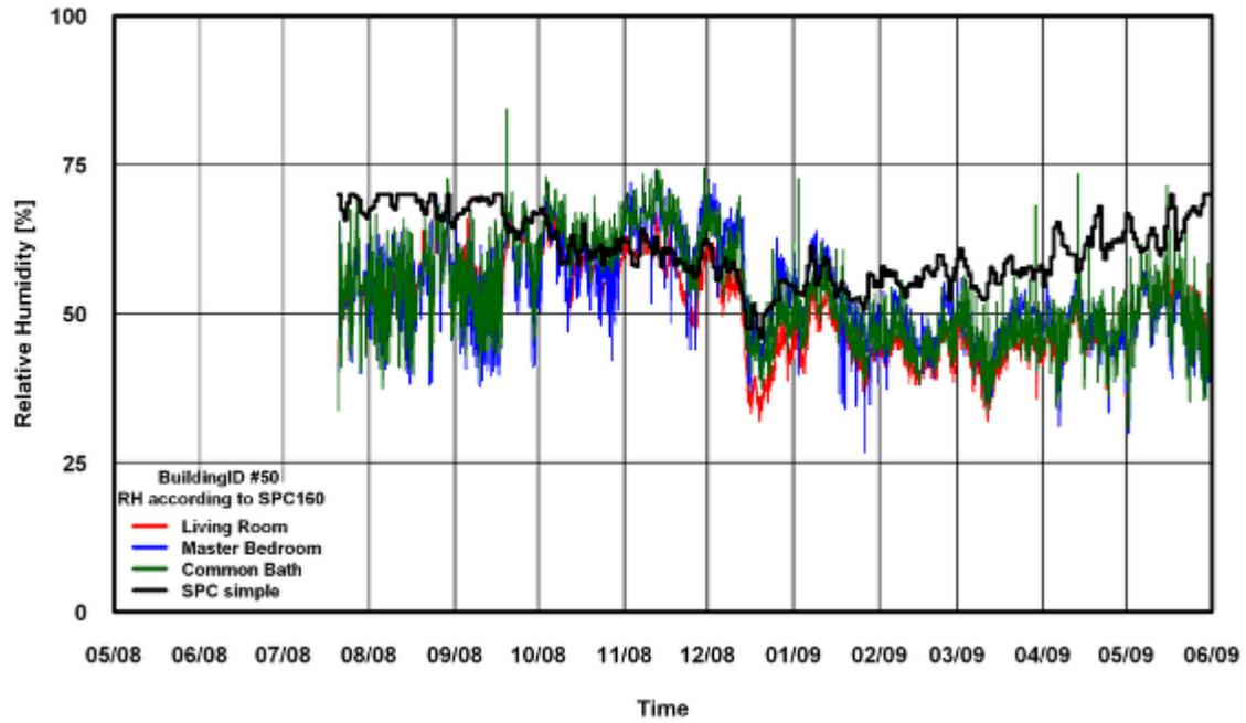
Figure 122: RH Comparison of SPC 160 Simple Method for Building # 50
