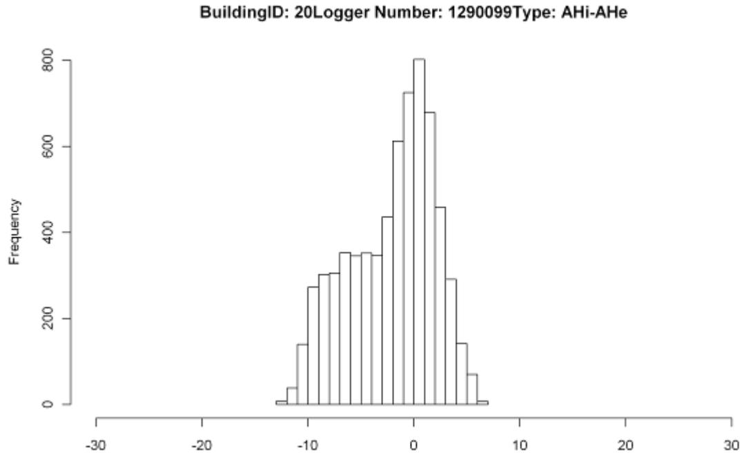
Figure 7: Frequency Plot for the difference in Moisture concentration (Inside -Outside)  $\text{g/m}^3$  for House 20
