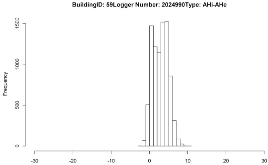
Figure 23: Frequency Plot for the difference in Moisture concentration (Inside -Outside)  $\text{g/m}^3$  for House 59
