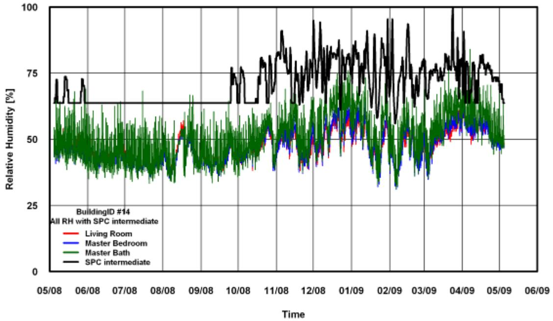
Figure 172: RH Comparison of SPC 160 Intermediate Method for Building # 14
