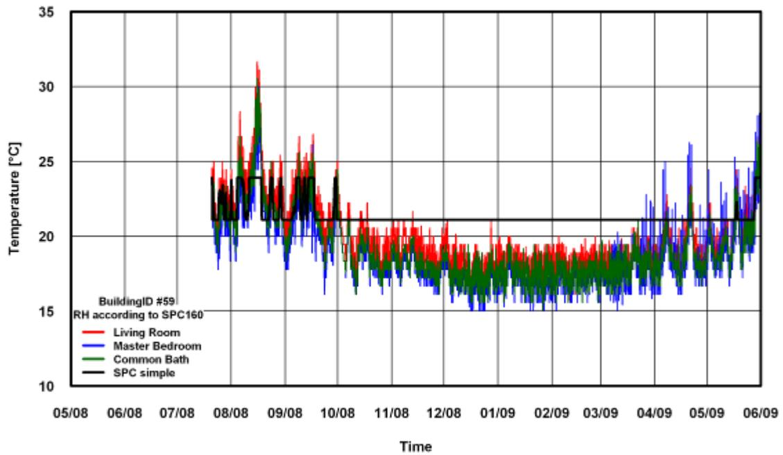
Figure 141: Temperature Comparison of SPC 160 Simple Method for Building # 59
