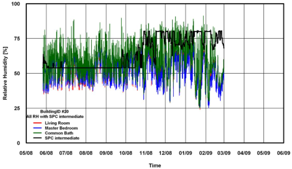
Figure 304: RH Comparison of SPC 160 Intermediate ANK Modified Method for Building # 20
