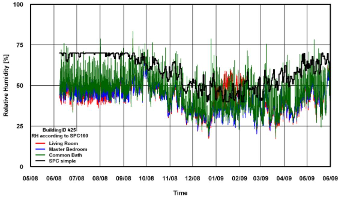
Figure 74: RH Comparison of SPC 160 Simple Method for Building # 25
