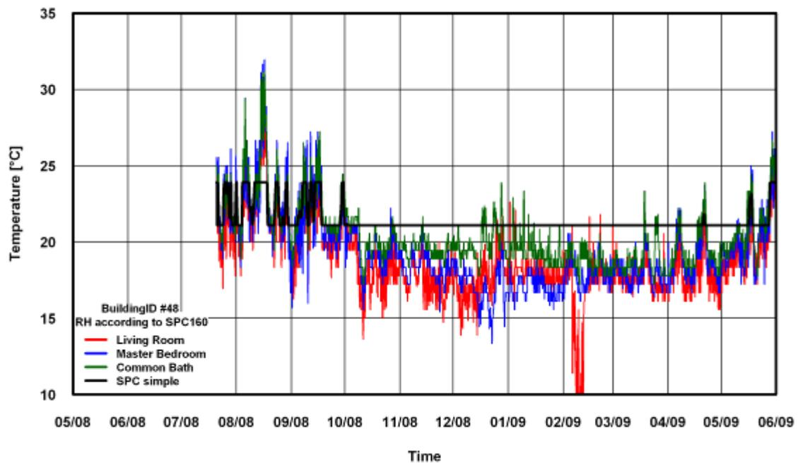
Figure 119: Temperature Comparison of SPC 160 Simple Method for Building # 48
