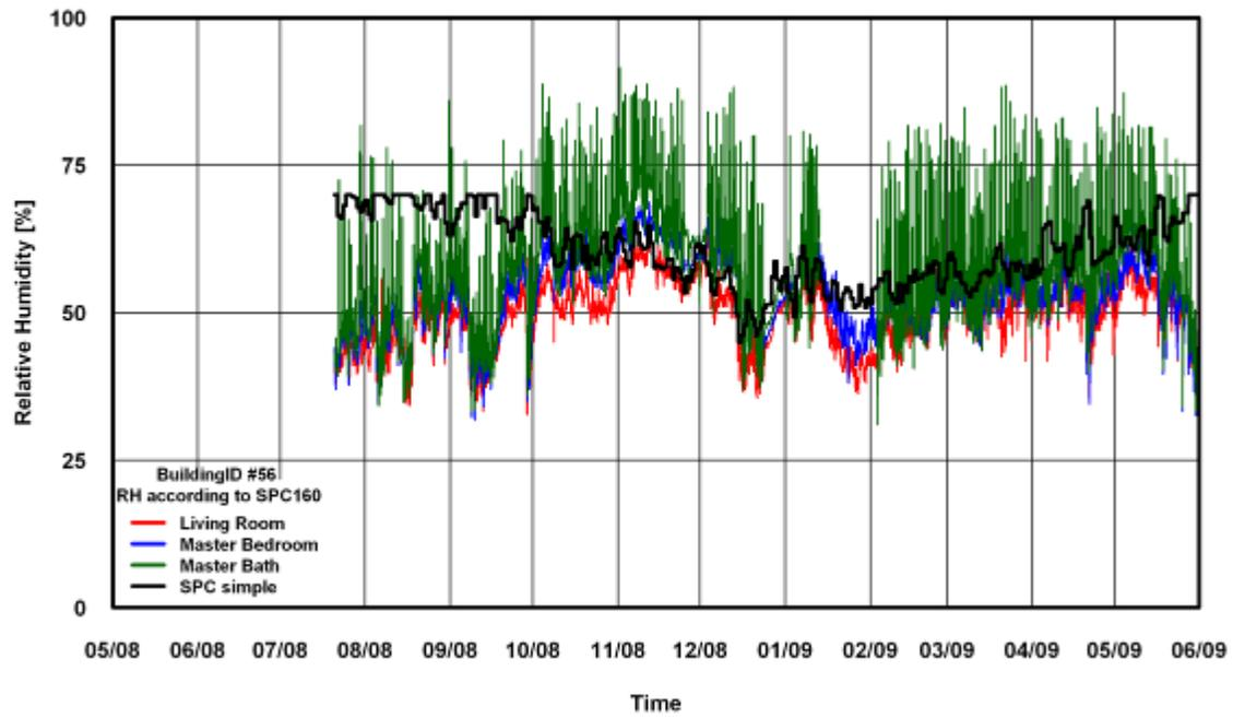
Figure 134: RH Comparison of SPC 160 Simple Method for Building # 56
