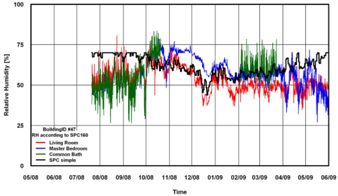
Figure 116: RH Comparison of SPC 160 Simple Method for Building # 47
