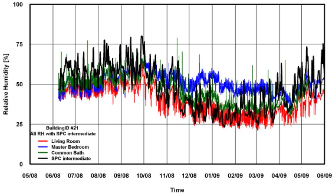
Figure 306: RH Comparison of SPC 160 Intermediate ANK Modified Method for Building # 21
