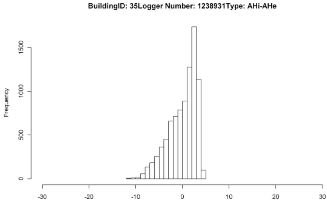
Figure 15: Frequency Plot for the difference in Moisture concentration (Inside -Outside)  $\text{g/m}^3$  for House 35
