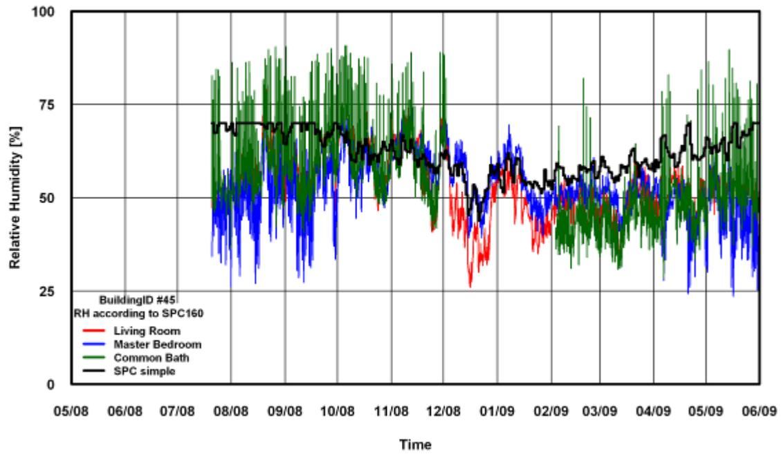
Figure 112: RH Comparison of SPC 160 Simple Method for Building # 45
