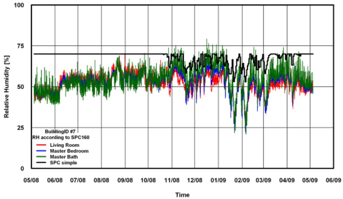
Figure 38: RH Comparison of SPC 160 Simple Method for Building # 7
