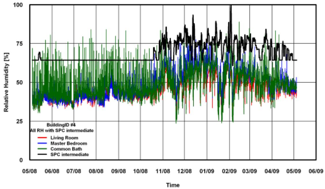
Figure 152: RH Comparison of SPC 160 Intermediate Method for Building # 4
