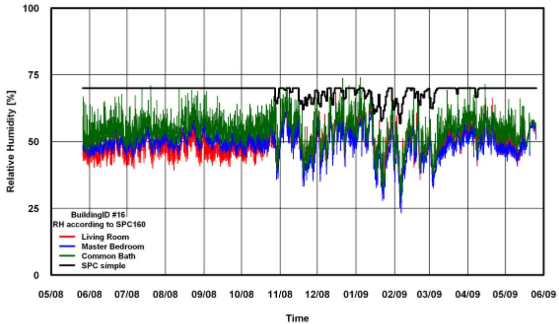
Figure 56: RH Comparison of SPC 160 Simple Method for Building # 16
