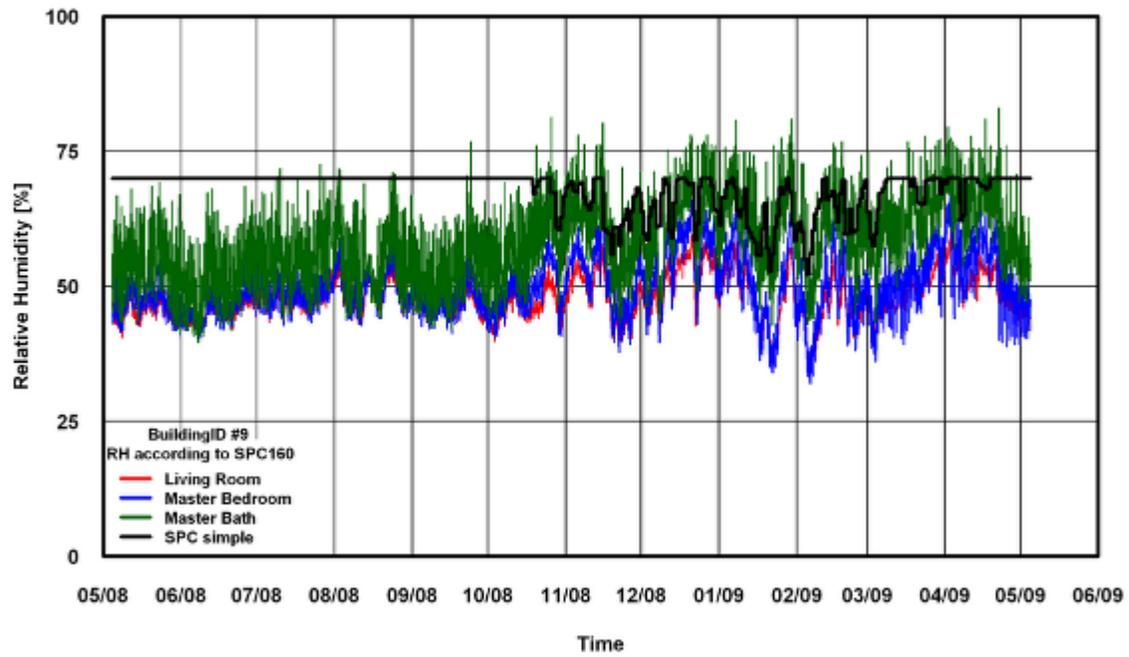
Figure 42: RH Comparison of SPC 160 Simple Method for Building #9
