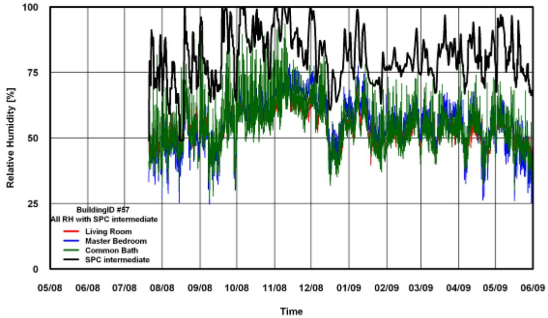
Figure 256: RH Comparison of SPC 160 Intermediate Method for Building # 57
