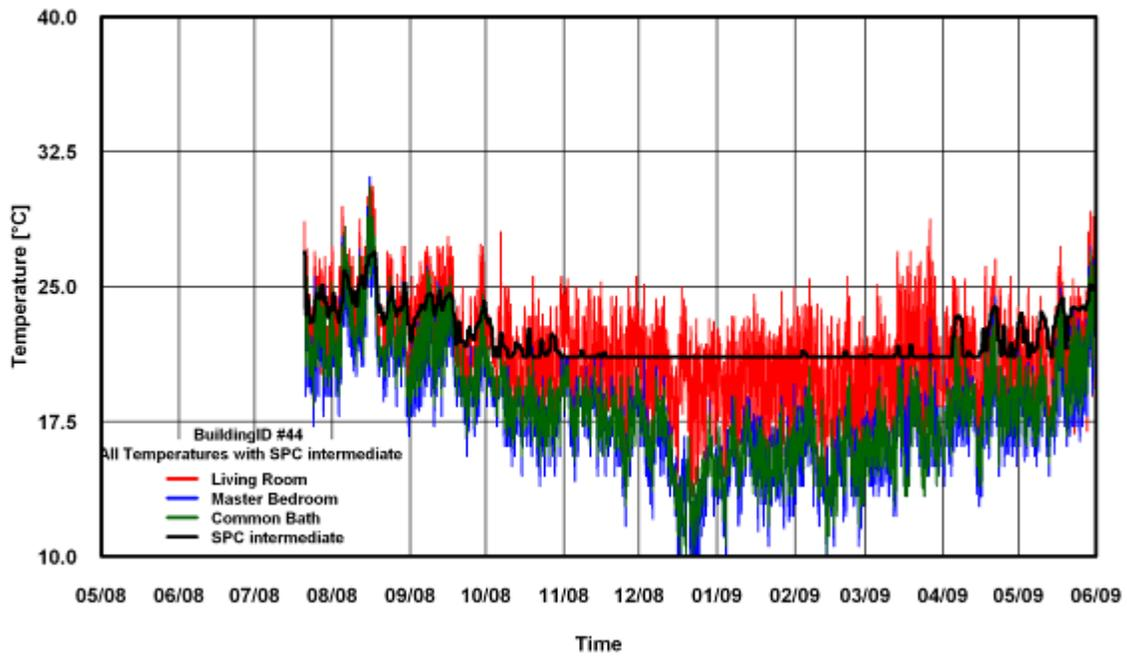
Figure 351: Temperature of SPC 160 Intermediate ANK Modified Method for Building # 44
