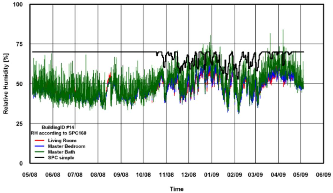
Figure 52: RH Comparison of SPC 160 Simple Method for Building # 14
