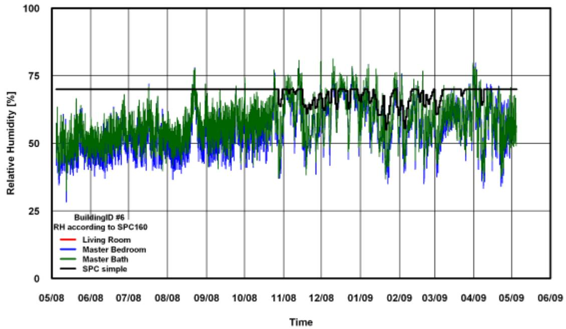
Figure 6: RH Comparison of SPC 160 Simple Method for Building # 6
