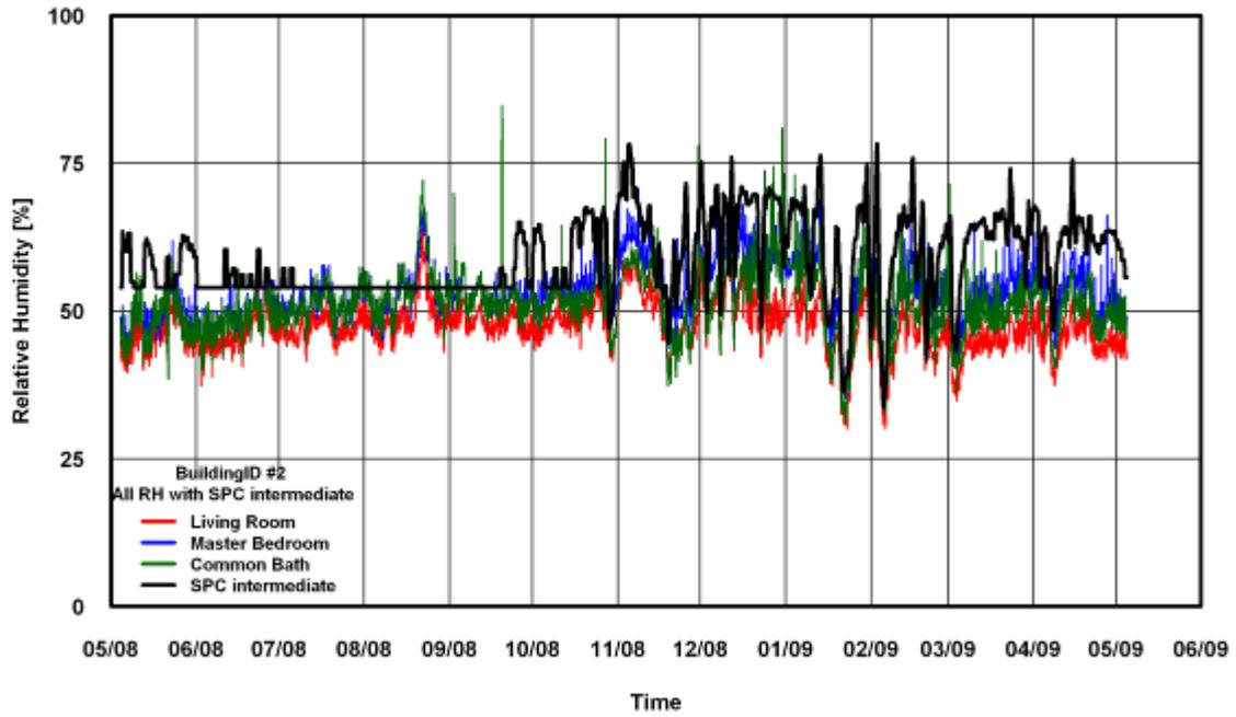
Figure 268: RH Comparison of SPC 160 Intermediate ANK Modified Method for Building # 2
