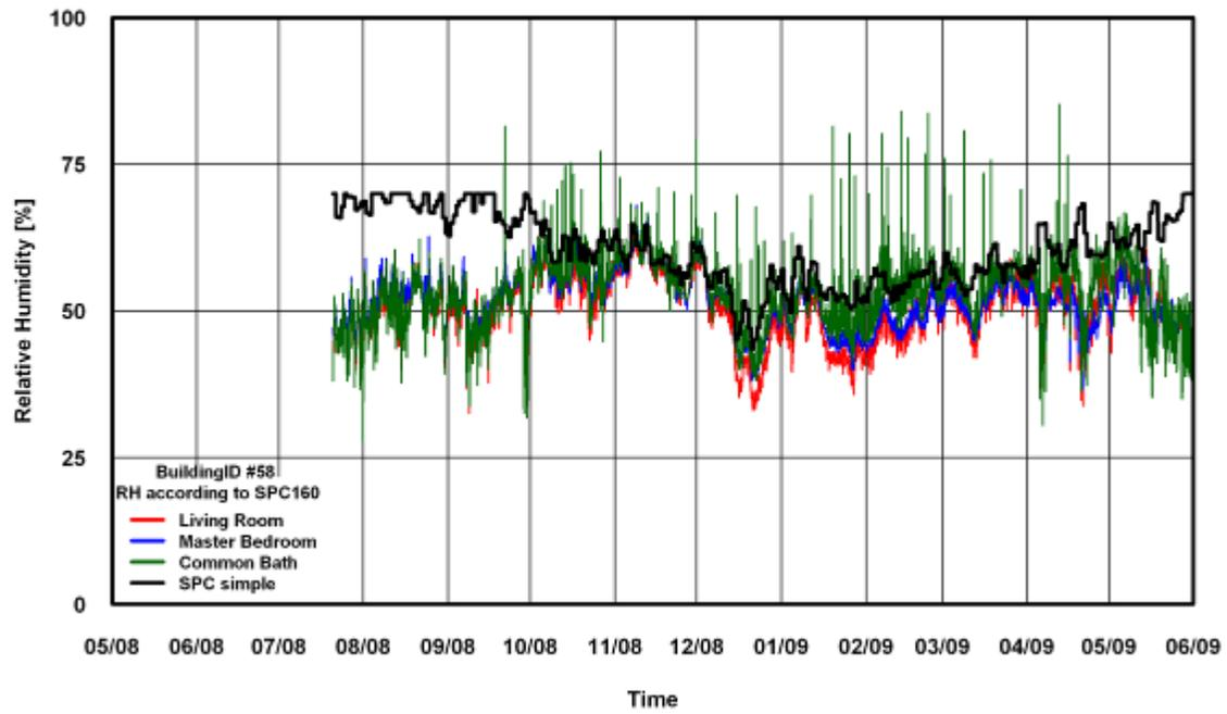
Figure 138: RH Comparison of SPC 160 Simple Method for Building # 58
