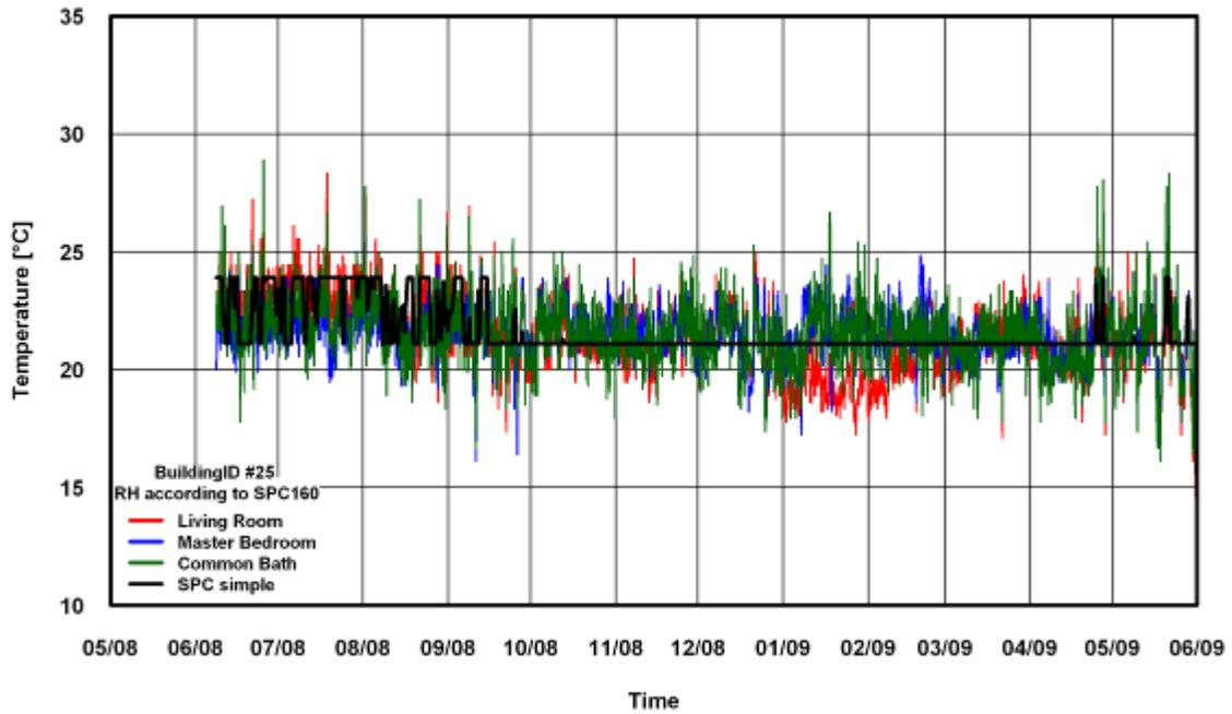
Figure 75: Temperature Comparison of SPC 160 Simple Method for Building # 25
