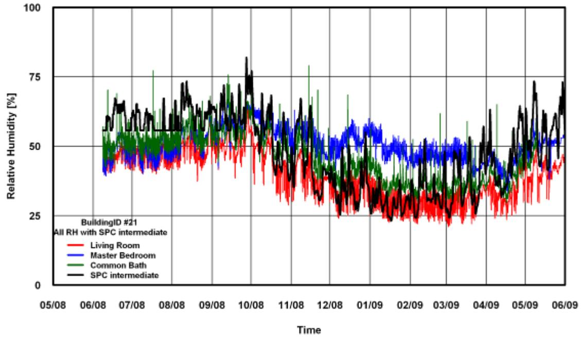
Figure 186: RH Comparison of SPC 160 Intermediate Method for Building # 21
