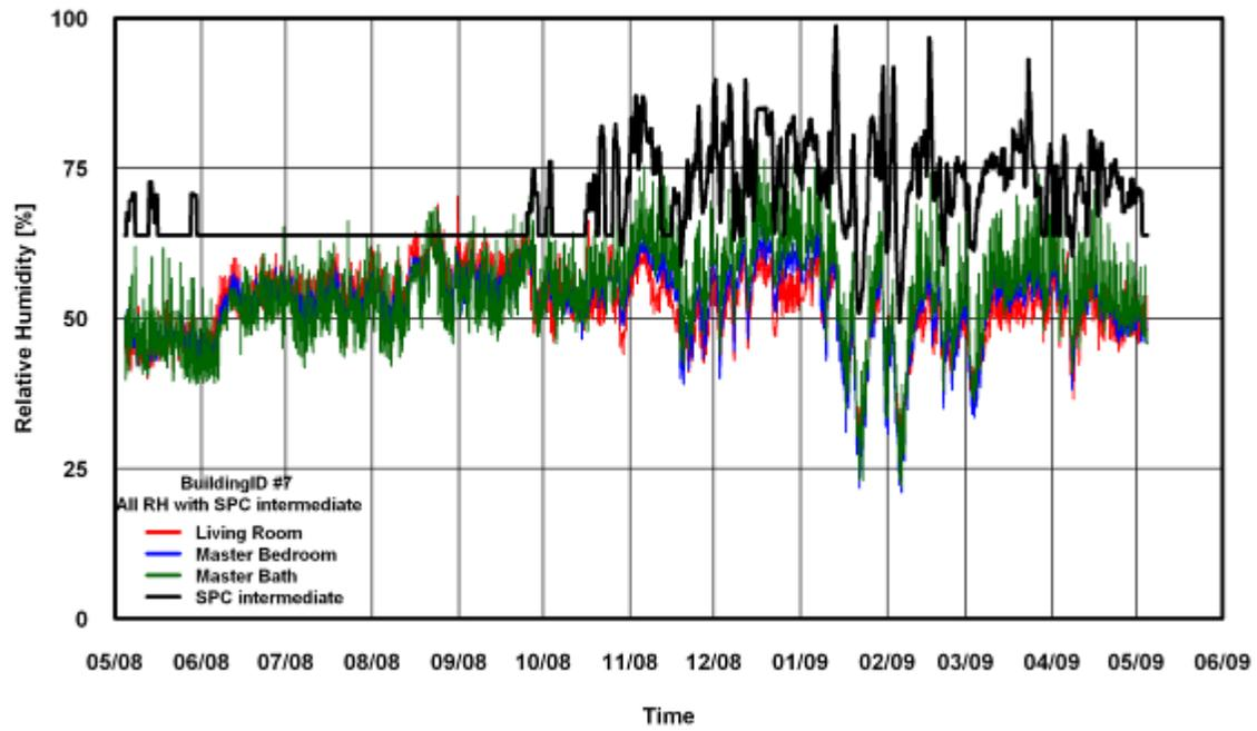
Figure 158: RH Comparison of SPC 160 Intermediate Method for Building # 7
