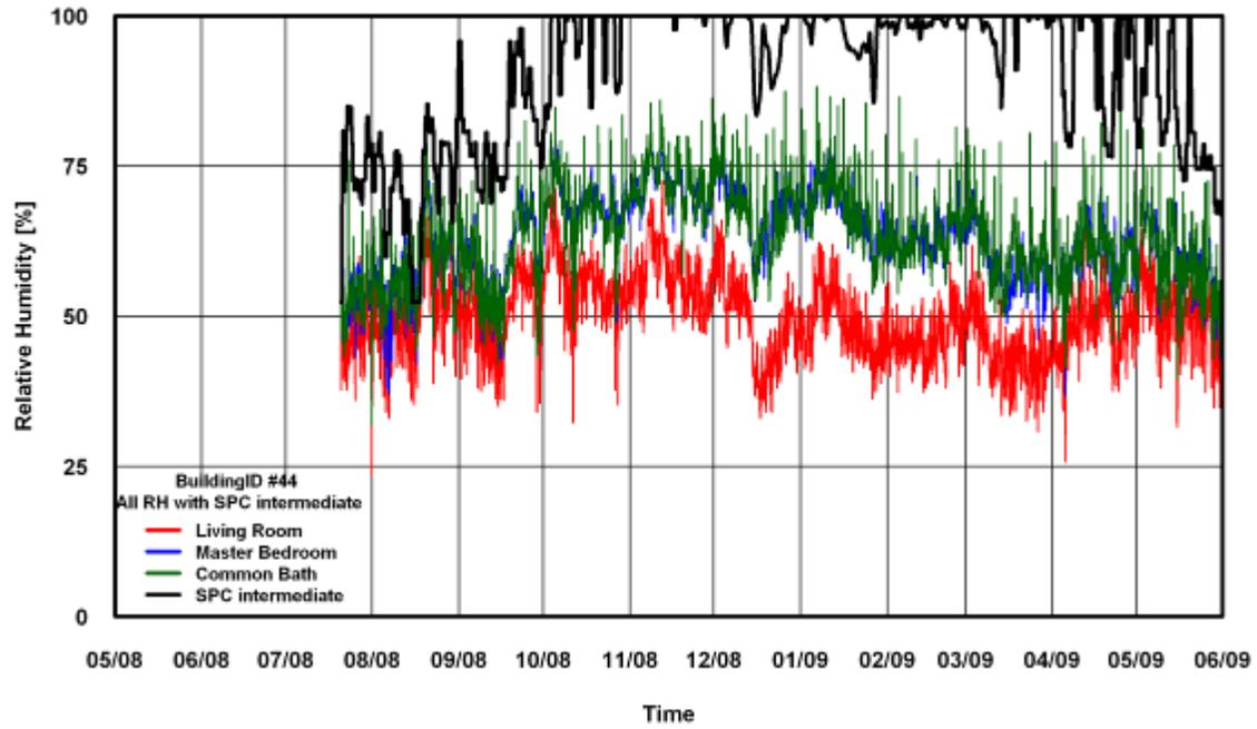
Figure 230: RH Comparison of SPC 160 Intermediate Method for Building # 44
