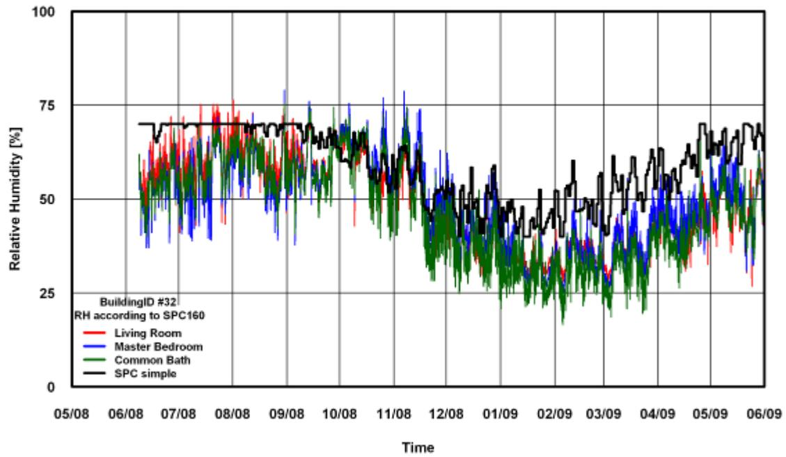
Figure 88: RH Comparison of SPC 160 Simple Method for Building # 32
