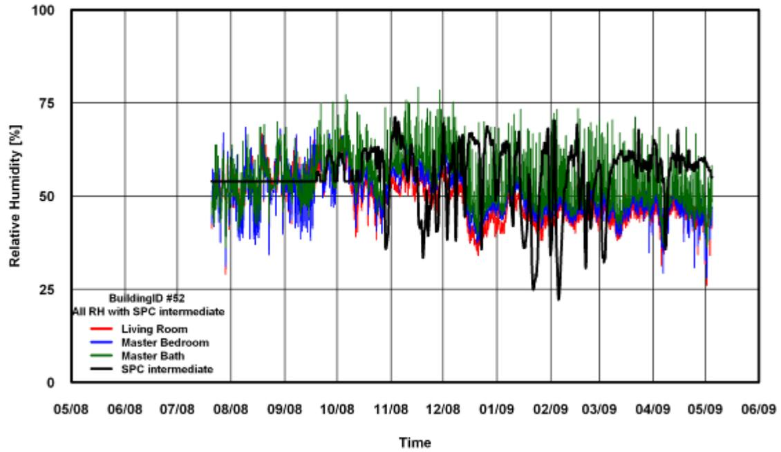
Figure 366: RH Comparison of SPC 160 Intermediate ANK Modified Method for Building # 52
