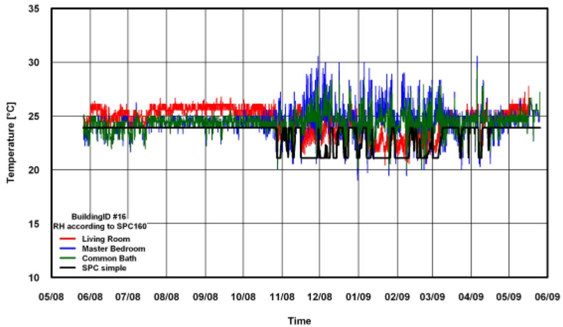
Figure 57: Temperature Comparison of SPC 160 Simple Method for Building # 16
