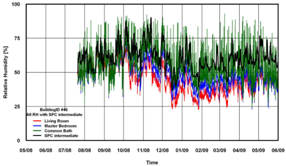
Figure 234: RH Comparison of SPC 160 Intermediate Method for Building # 46
