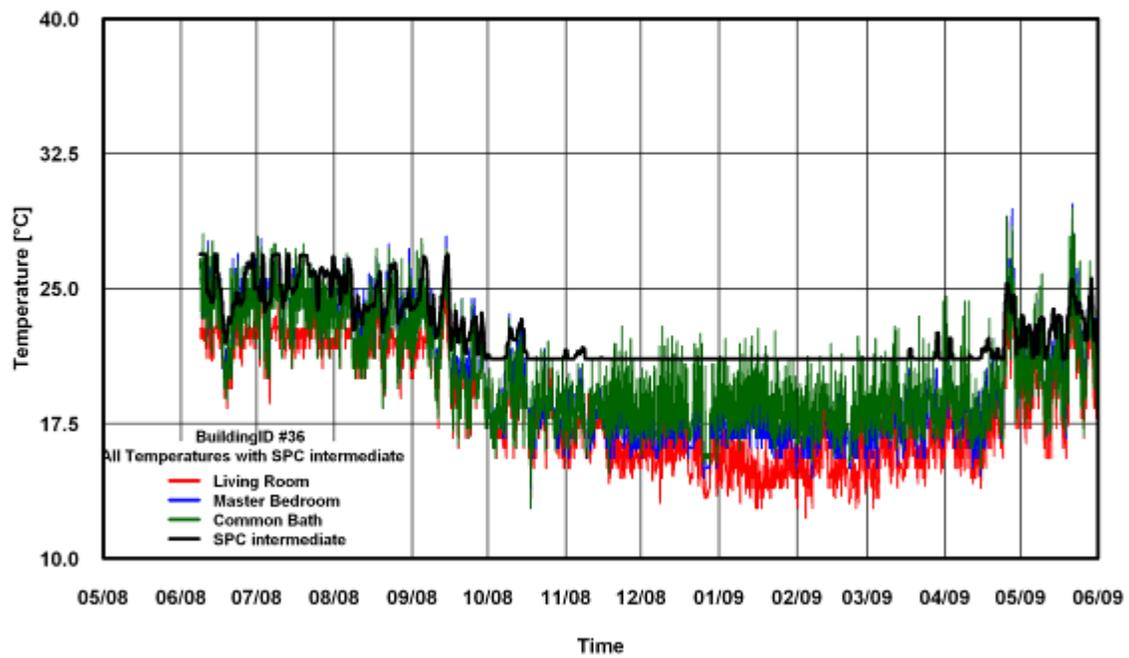
Figure 337: Temperature of SPC 160 Intermediate ANK Modified Method for Building # 36
