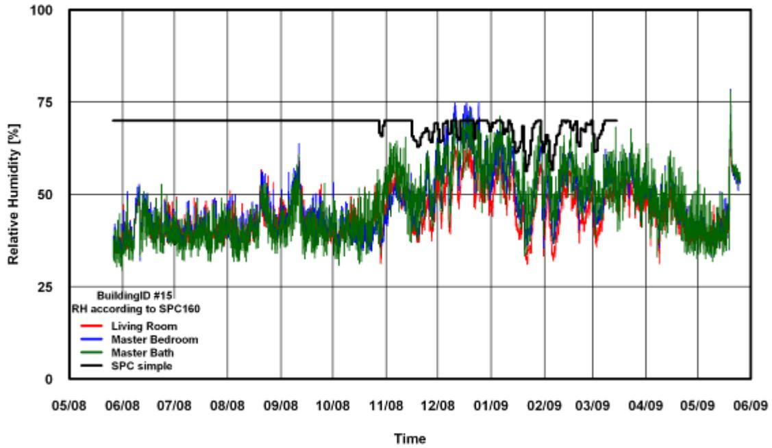
Figure 54: RH Comparison of SPC 160 Simple Method for Building # 15
