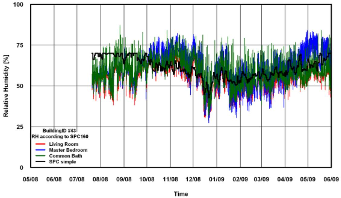
Figure 108: RH Comparison of SPC 160 Simple Method for Building # 43
