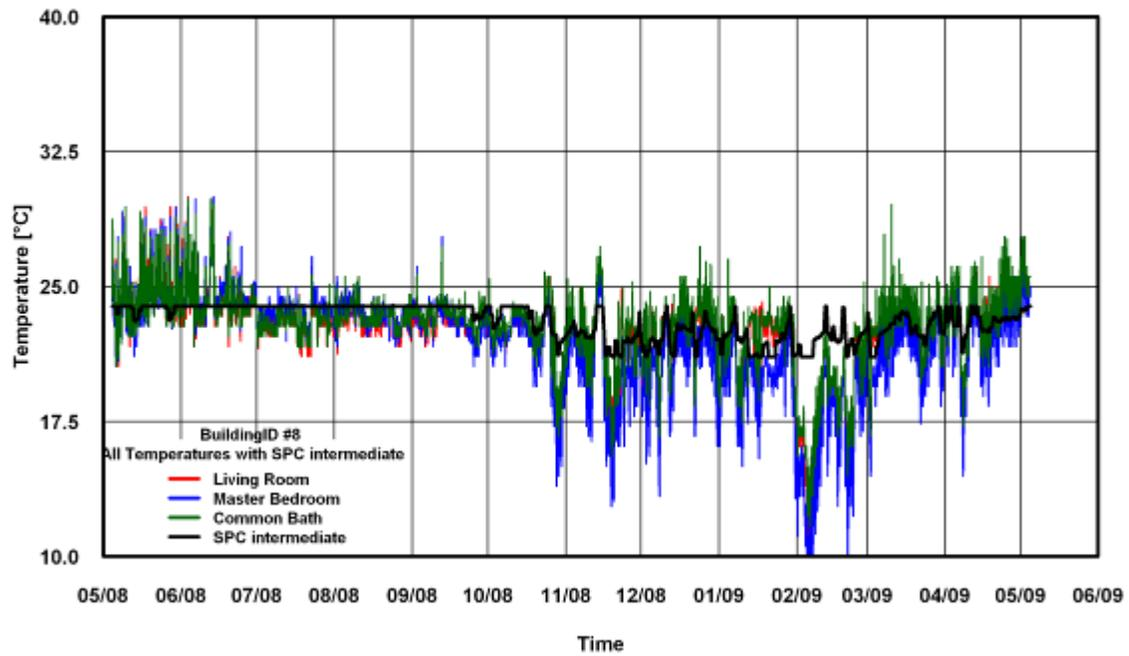
Figure 161: Temperature of SPC 160 Intermediate Method for Building # 8
