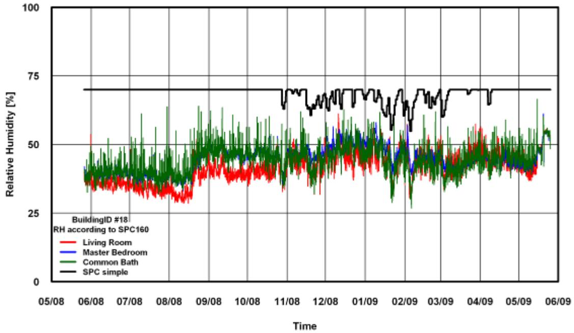
Figure 60: RH Comparison of SPC 160 Simple Method for Building # 18
