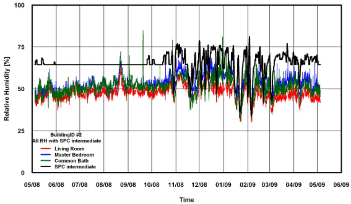
Figure 148: RH Comparison of SPC 160 Intermediate Method for Building # 2
