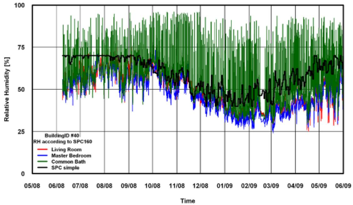
Figure 104: RH Comparison of SPC 160 Simple Method for Building # 40
