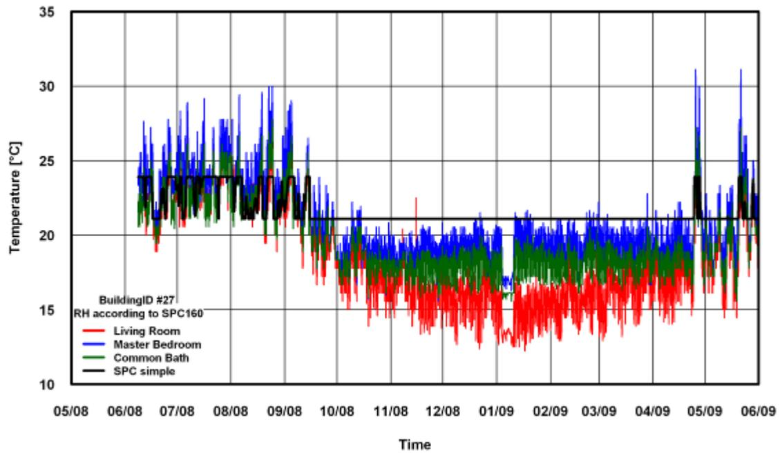
Figure 79: Temperature Comparison of SPC 160 Simple Method for Building # 27
