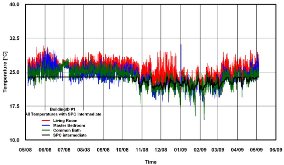
Figure 147: Temperature of SPC 160 Intermediate Method for Building # 1
