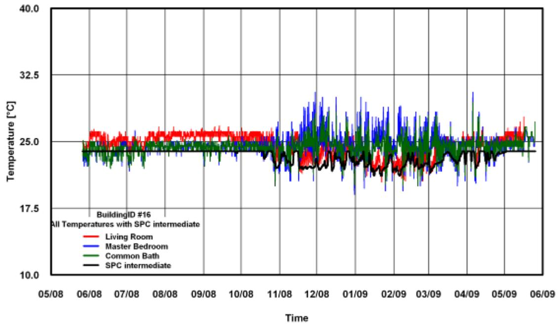
Figure 177: Temperature of SPC 160 Intermediate Method for Building # 16
