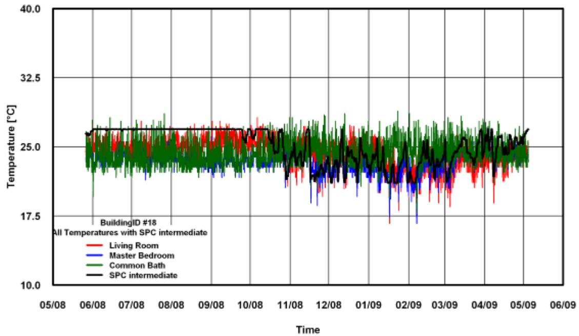
Figure 301: Temperature of SPC 160 Intermediate ANK Modified Method for Building # 18
