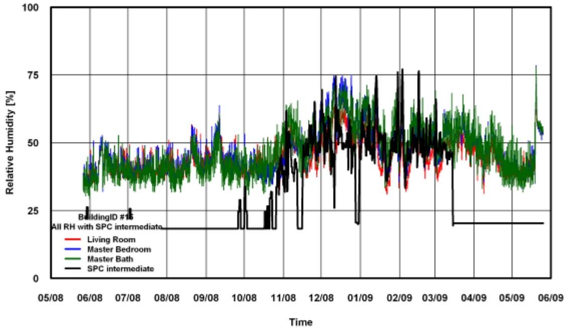
Figure 294: RH Comparison of SPC 160 Intermediate ANK Modified Method for Building # 15
