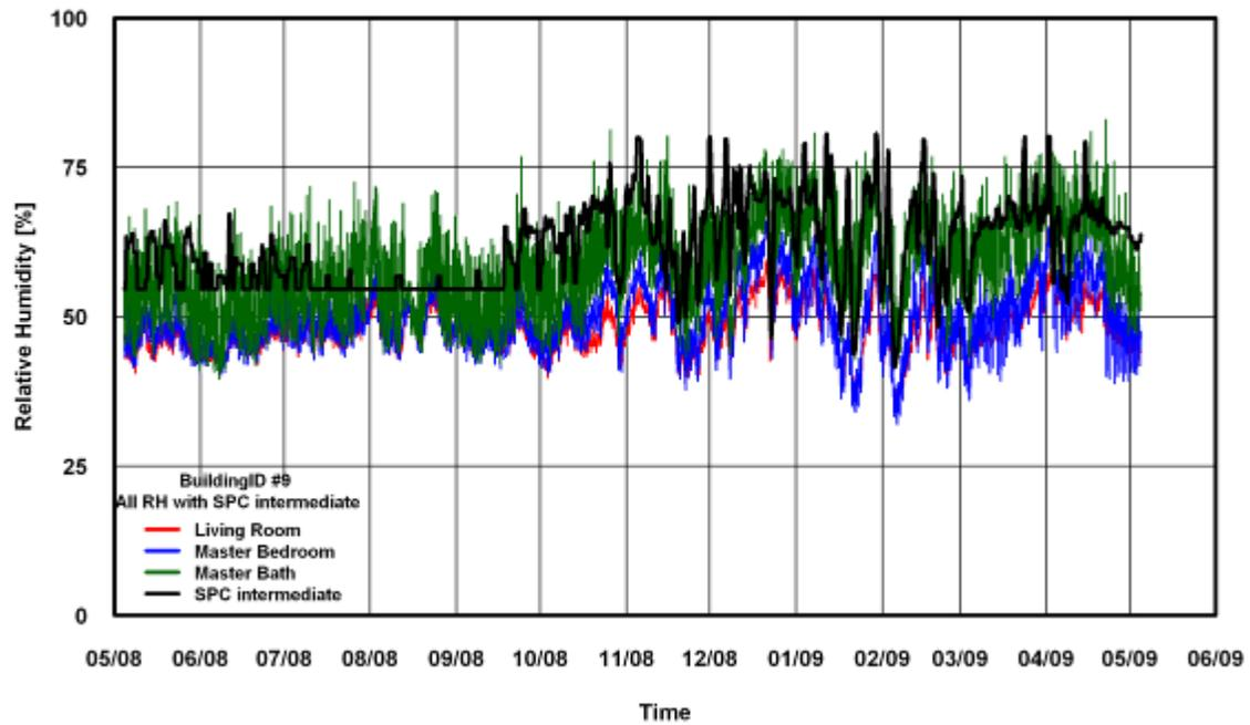
Figure 282: RH Comparison of SPC 160 Intermediate ANK Modified Method for Building # 9
