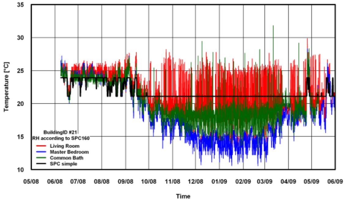
Figure 67: Temperature Comparison of SPC 160 Simple Method for Building # 21
