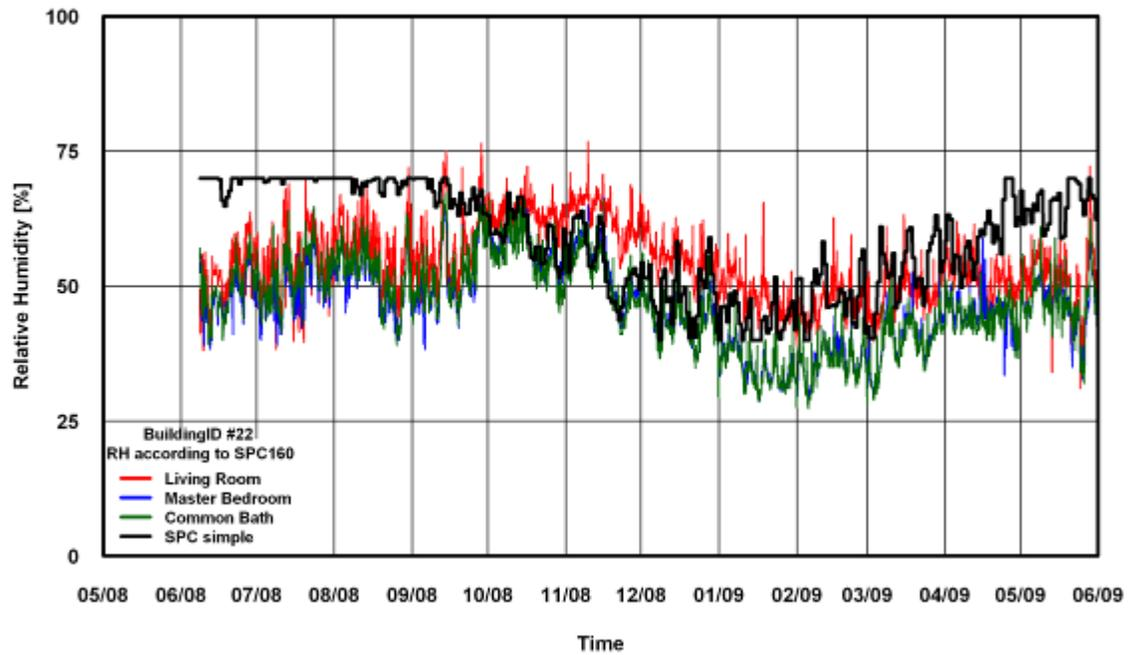
Figure 68: RH Comparison of SPC 160 Simple Method for Building # 22
