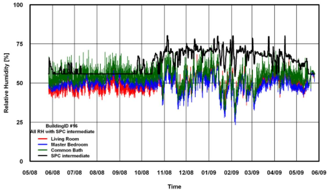
Figure 296: RH Comparison of SPC 160 Intermediate ANK Modified Method for Building # 16
