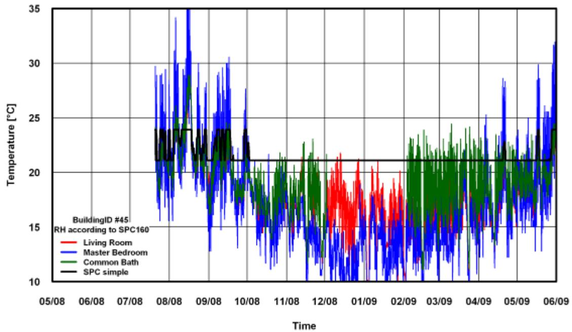
Figure 113: Temperature Comparison of SPC 160 Simple Method for Building # 45
