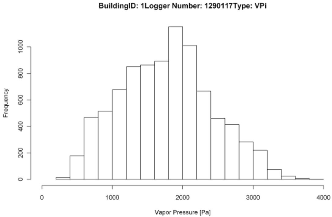
Figure 4: Frequency Plot for the Interior Vapor Pressure (Pa) for House 1
