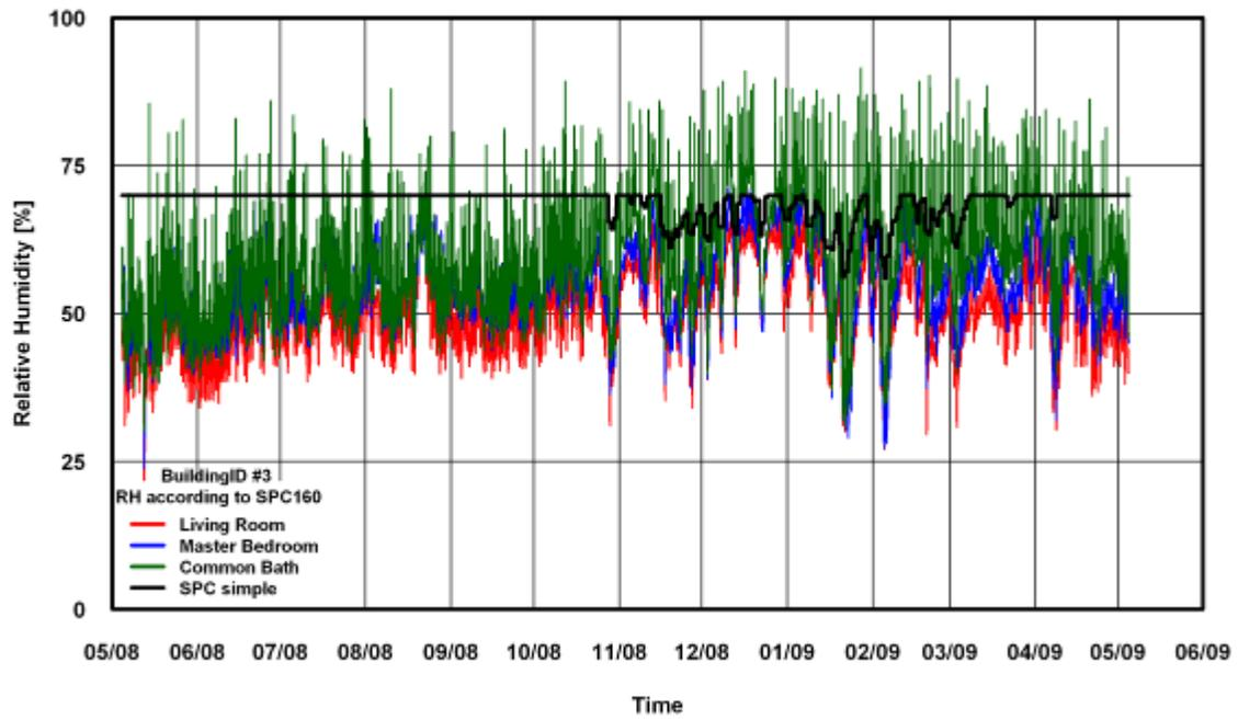
Figure 31: RH Comparison of SPC 160 Simple Method for Building # 3
