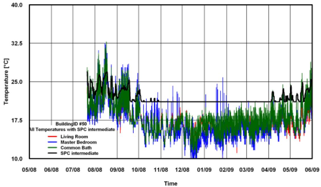
Figure 363: Temperature of SPC 160 Intermediate ANK Modified Method for Building # 50
