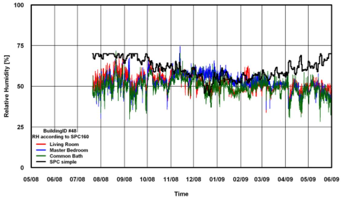
Figure 118: RH Comparison of SPC 160 Simple Method for Building # 48
