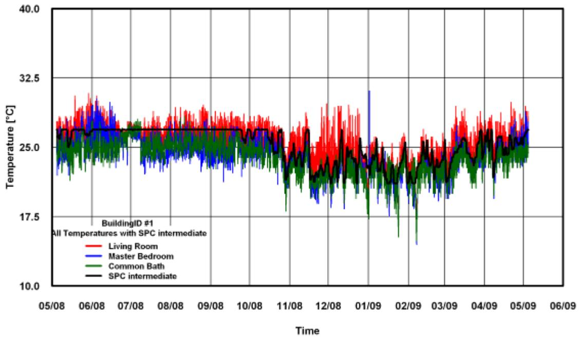
Figure 267: Temperature of SPC 160 Intermediate ANK Modified Method for Building # 1
