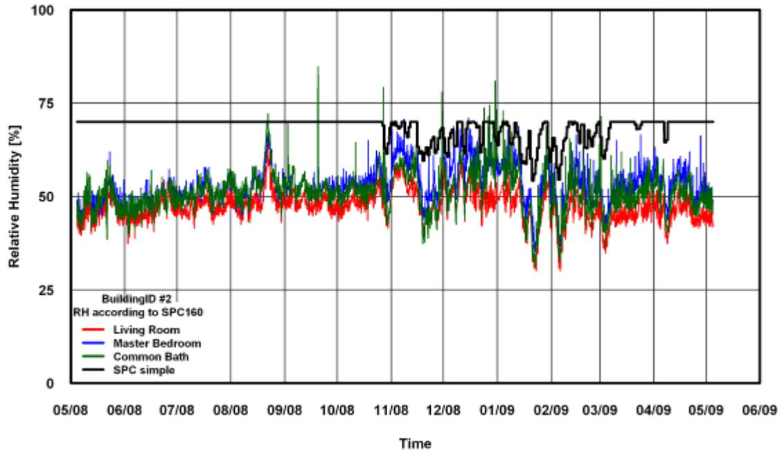
Figure 29: RH Comparison of SPC 160 Simple Method for Building # 2
