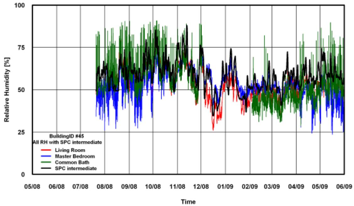
Figure 232: RH Comparison of SPC 160 Intermediate Method for Building # 45
