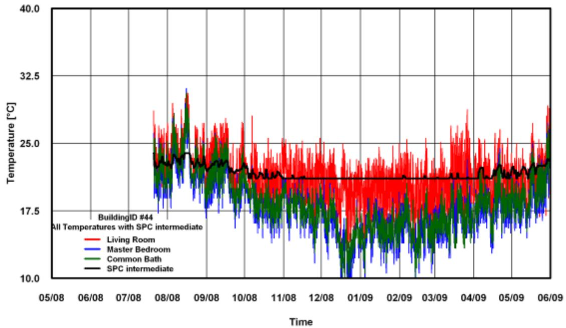
Figure 231: Temperature of SPC 160 Intermediate Method for Building # 44
