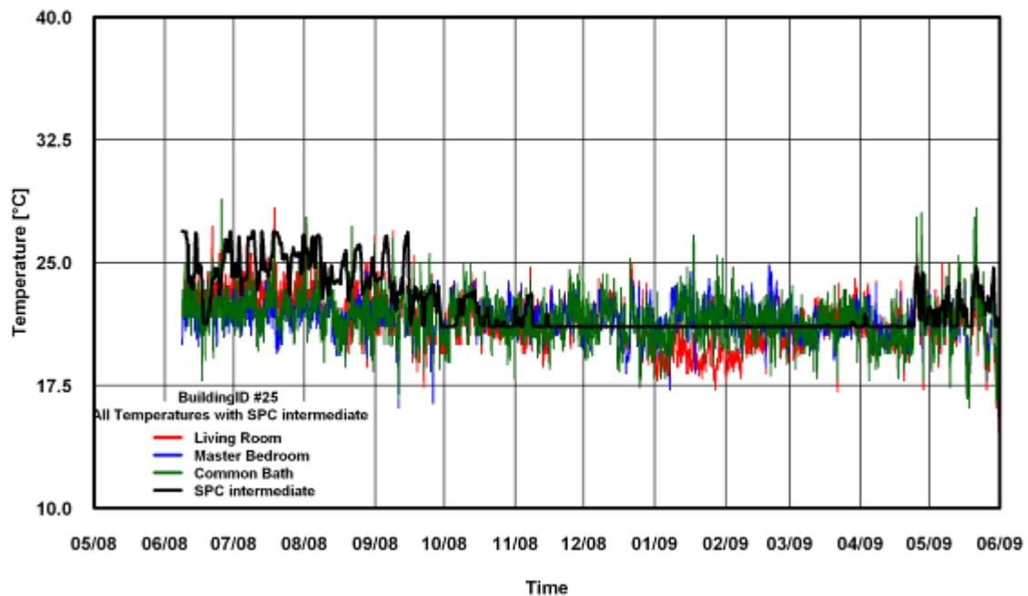
Figure 315: Temperature of SPC 160 Intermediate ANK Modified Method for Building # 25
