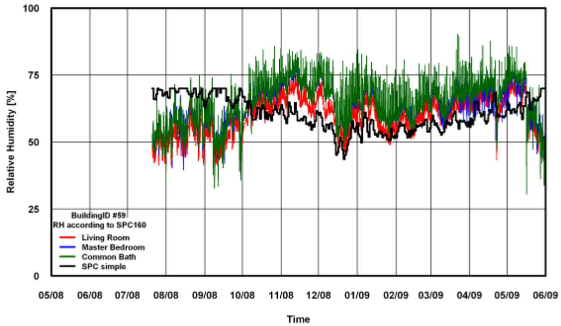
Figure 140: RH Comparison of SPC 160 Simple Method for Building # 59
