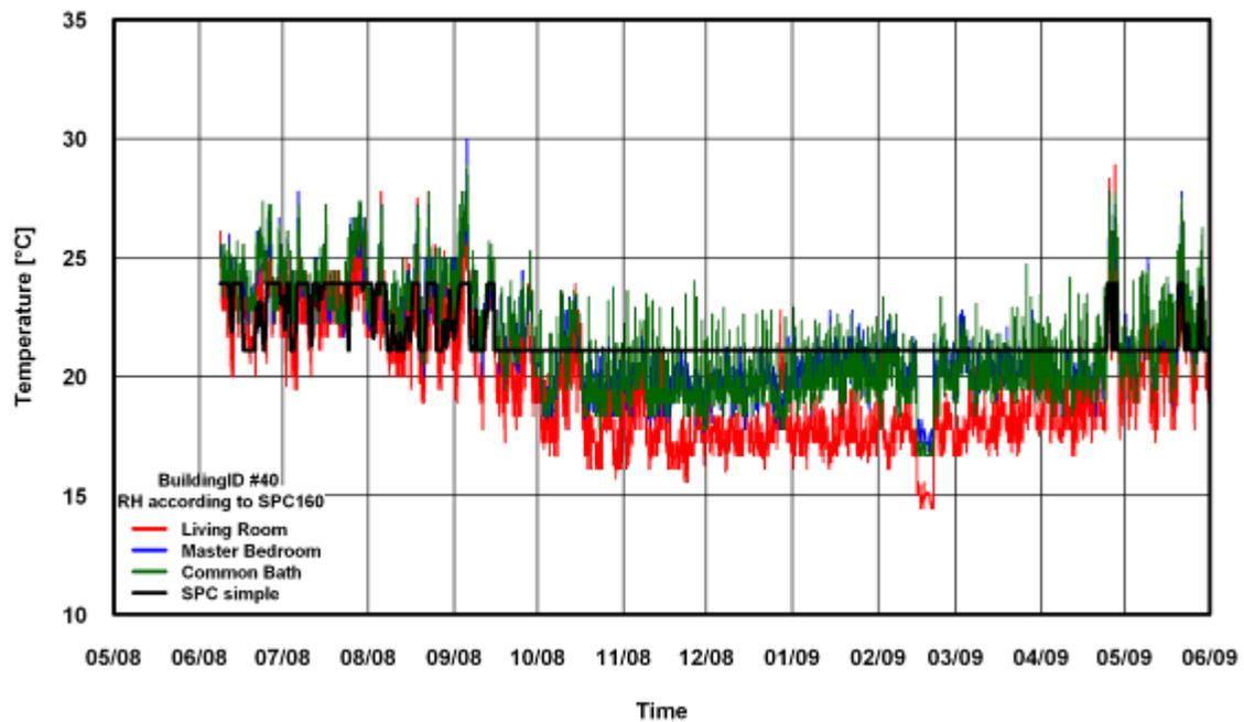
Figure 105: Temperature Comparison of SPC 160 Simple Method for Building # 40
