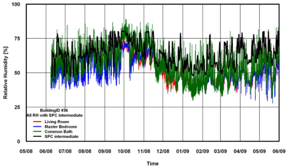
Figure 336: RH Comparison of SPC 160 Intermediate ANK Modified Method for Building # 36
