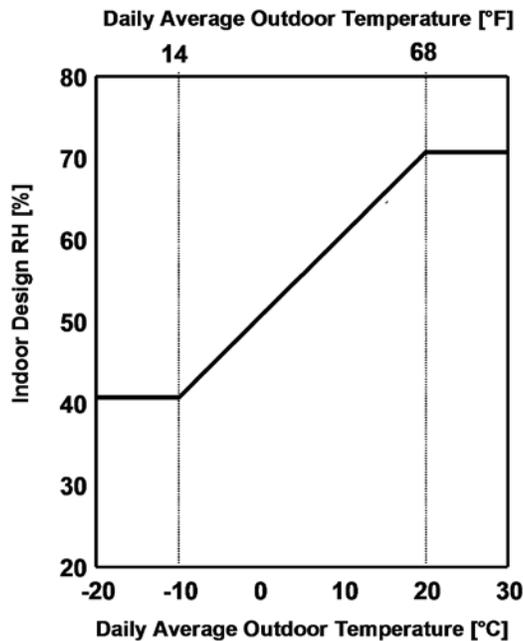
Figure 1: Design Indoor RH, Simplified Method
