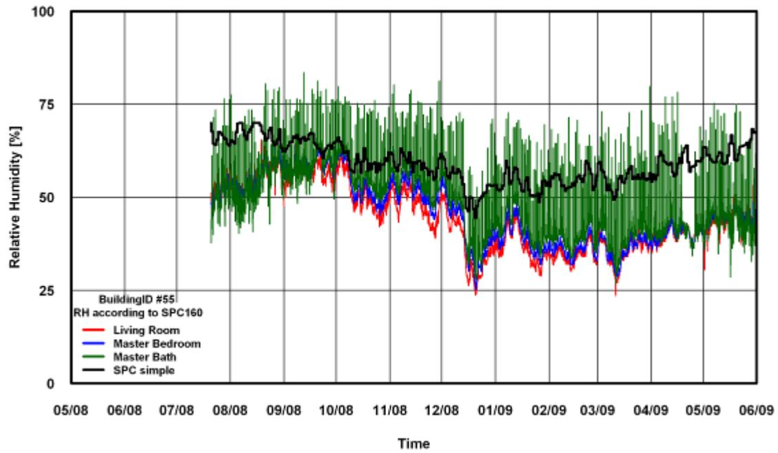
Figure 132: RH Comparison of SPC 160 Simple Method for Building # 55
