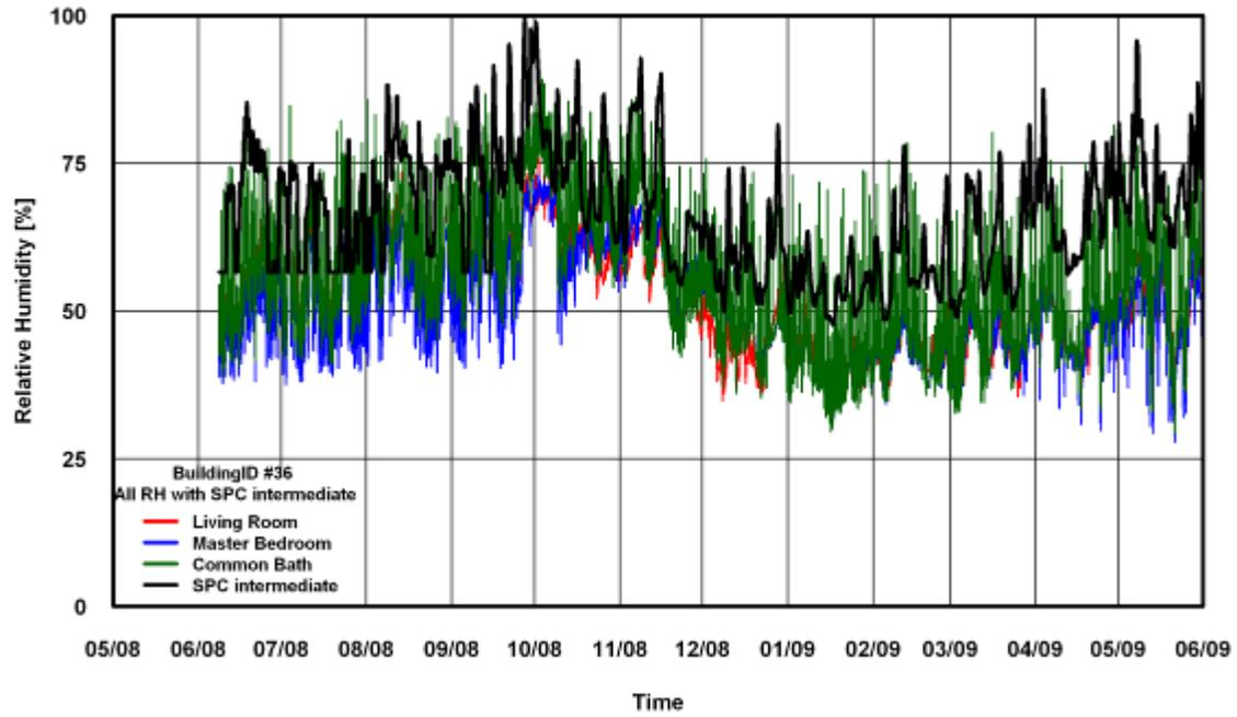
Figure 216: RH Comparison of SPC 160 Intermediate Method for Building # 36
