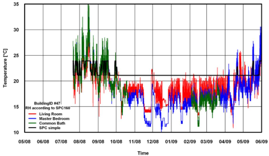
Figure 117: Temperature Comparison of SPC 160 Simple Method for Building # 47
