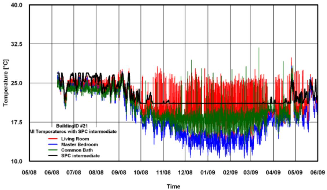
Figure 307: Temperature of SPC 160 Intermediate ANK Modified Method for Building # 21
