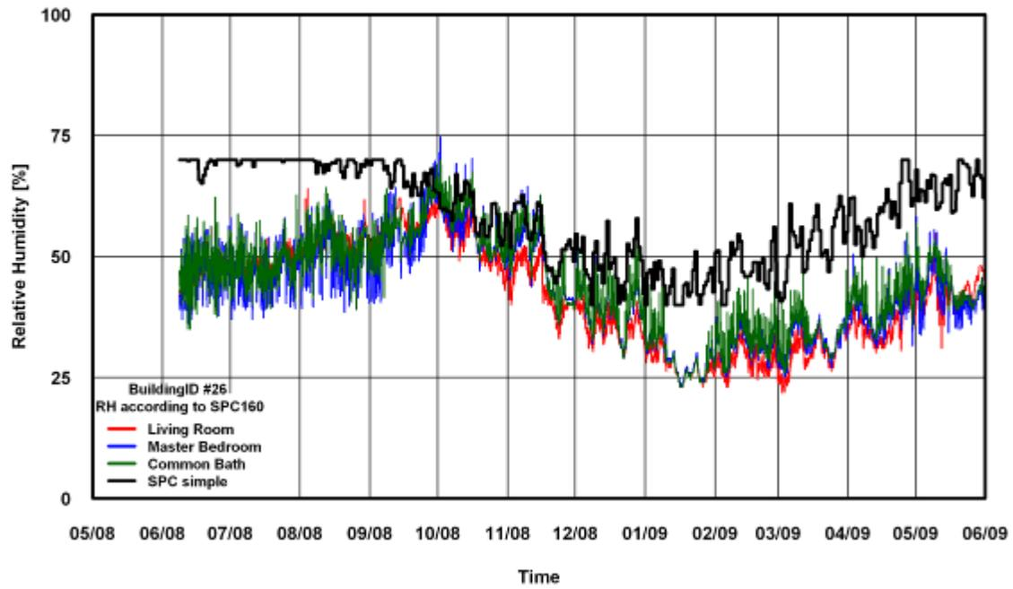
Figure 76: RH Comparison of SPC 160 Simple Method for Building # 26
