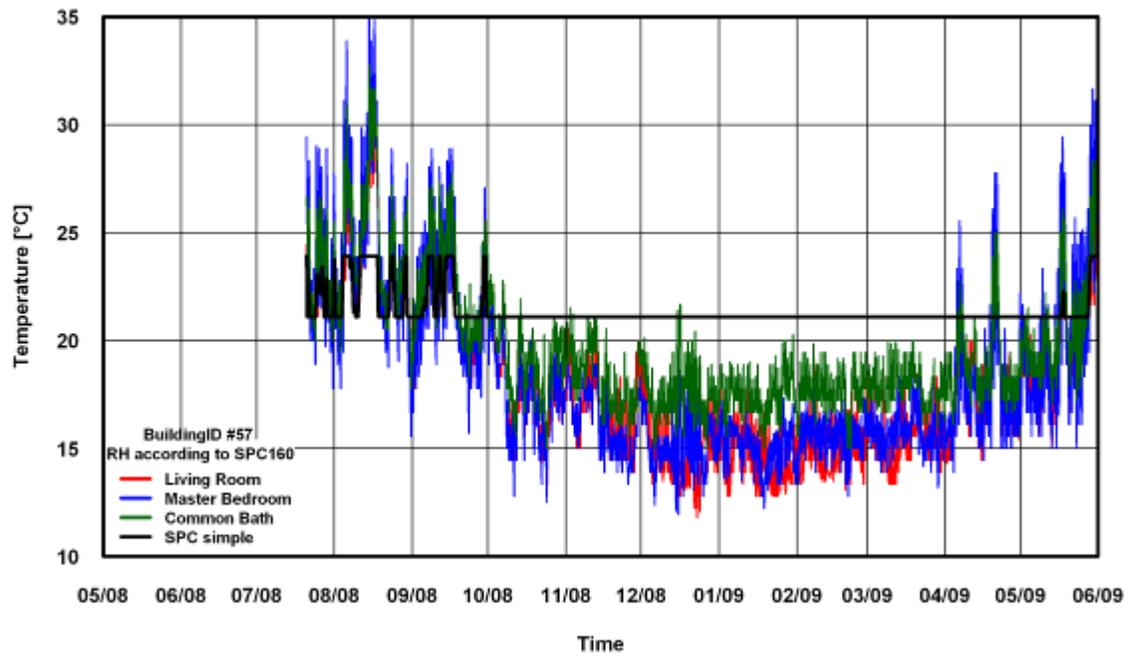
Figure 137: Temperature Comparison of SPC 160 Simple Method for Building # 57
