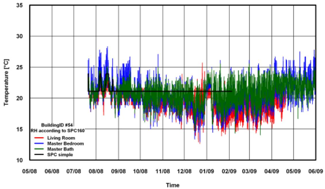
Figure 131: Temperature Comparison of SPC 160 Simple Method for Building # 54
