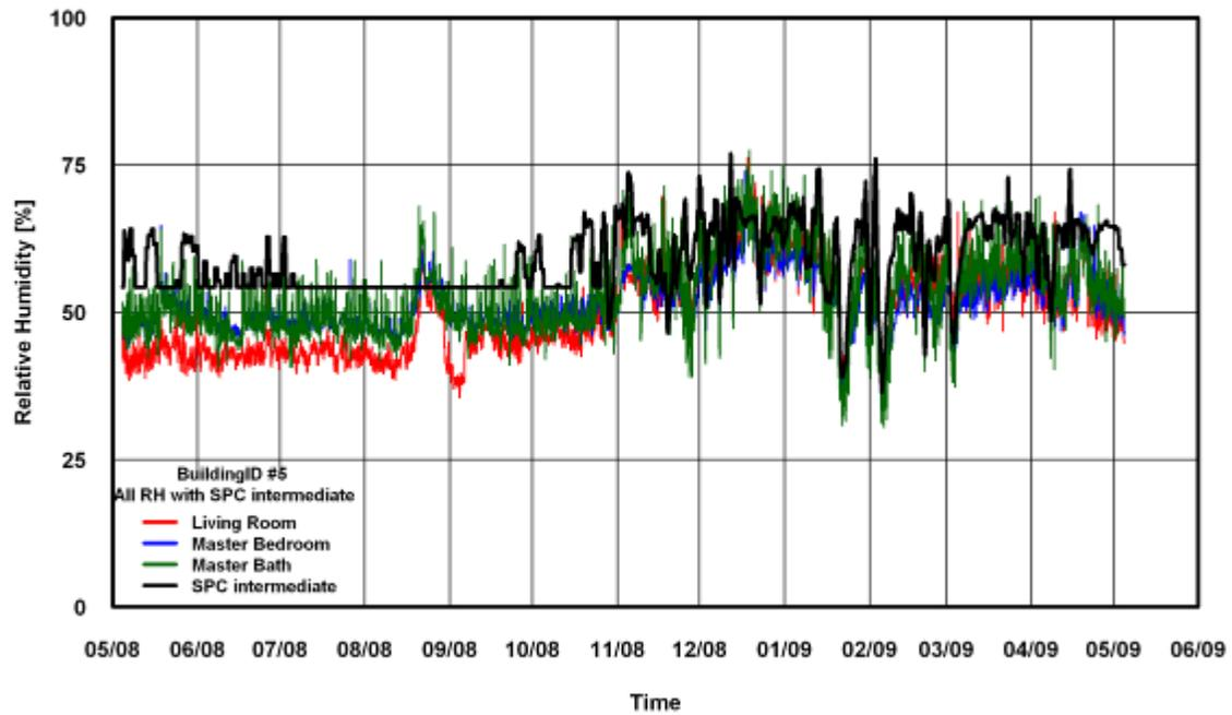
Figure 274: RH Comparison of SPC 160 Intermediate ANK Modified Method for Building # 5
