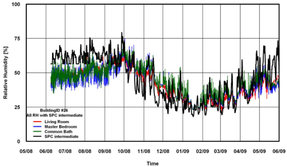
Figure 196: RH Comparison of SPC 160 Intermediate Method for Building # 26
