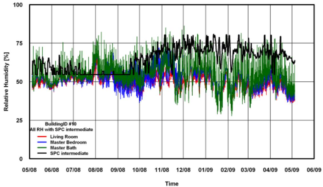
Figure 284: RH Comparison of SPC 160 Intermediate ANK Modified Method for Building # 10
