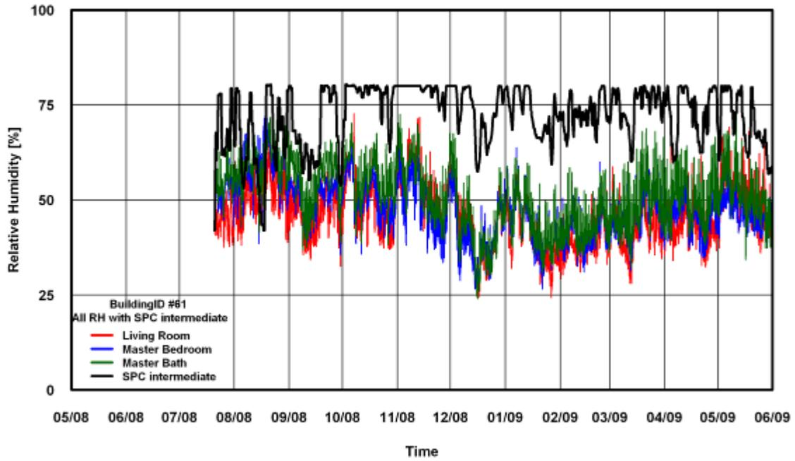
Figure 384: RH Comparison of SPC 160 Intermediate ANK Modified Method for Building # 61
