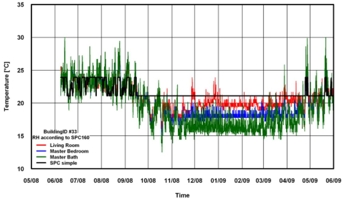
Figure 91: Temperature Comparison of SPC 160 Simple Method for Building # 33
