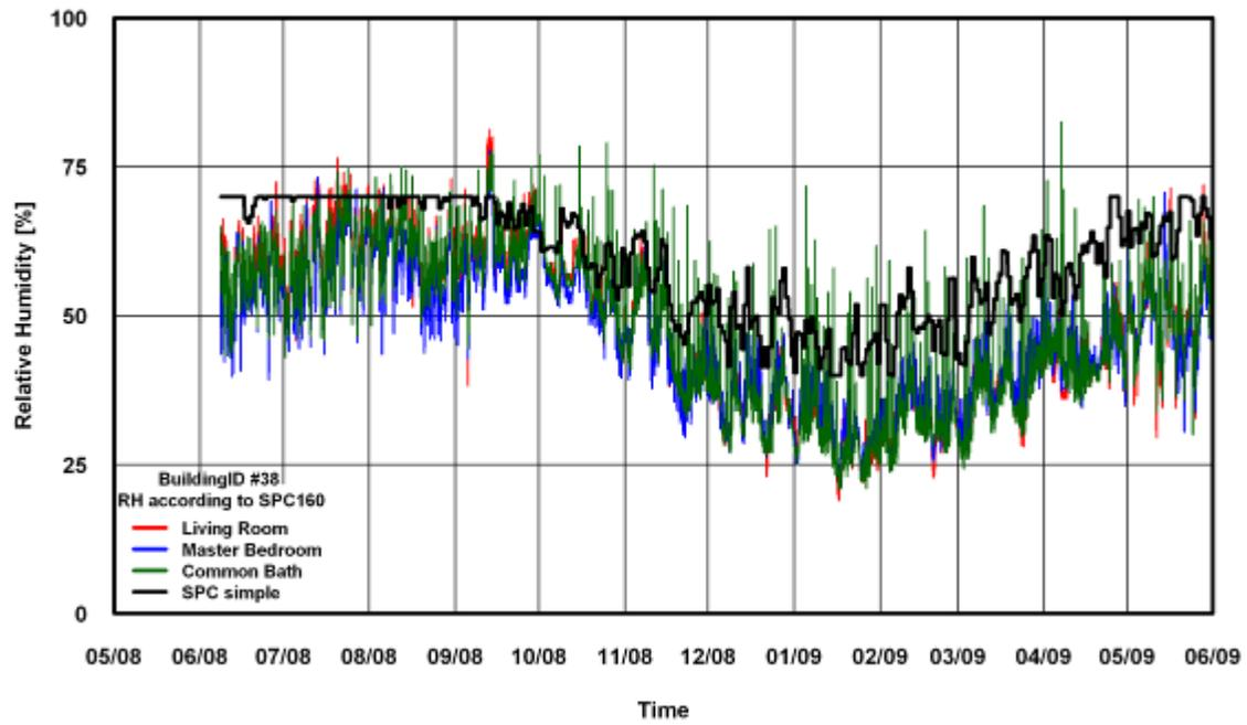
Figure 100: RH Comparison of SPC 160 Simple Method for Building # 38
