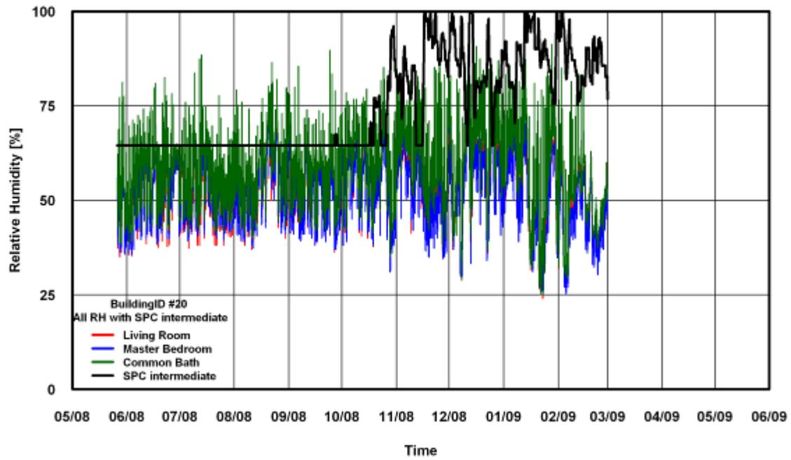
Figure 184: RH Comparison of SPC 160 Intermediate Method for Building # 20
