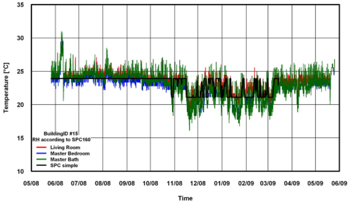
Figure 55: Temperature Comparison of SPC 160 Simple Method for Building # 15
