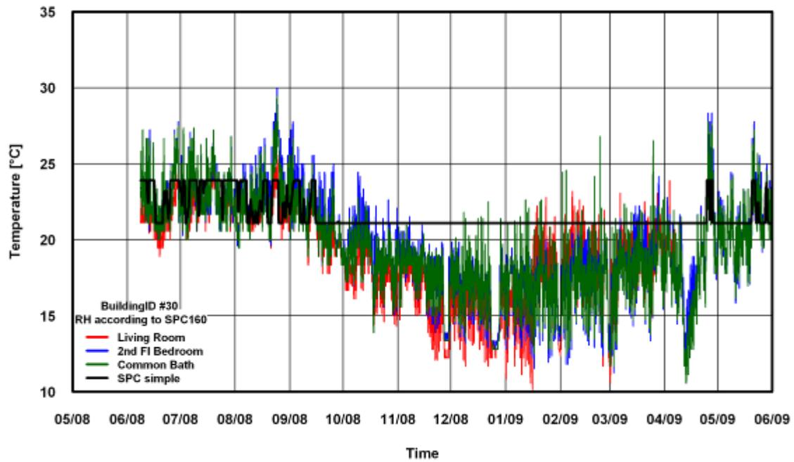
Figure 85: Temperature Comparison of SPC 160 Simple Method for Building # 30
