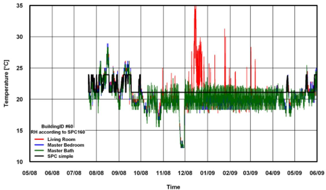
Figure 143: Temperature Comparison of SPC 160 Simple Method for Building # 60
