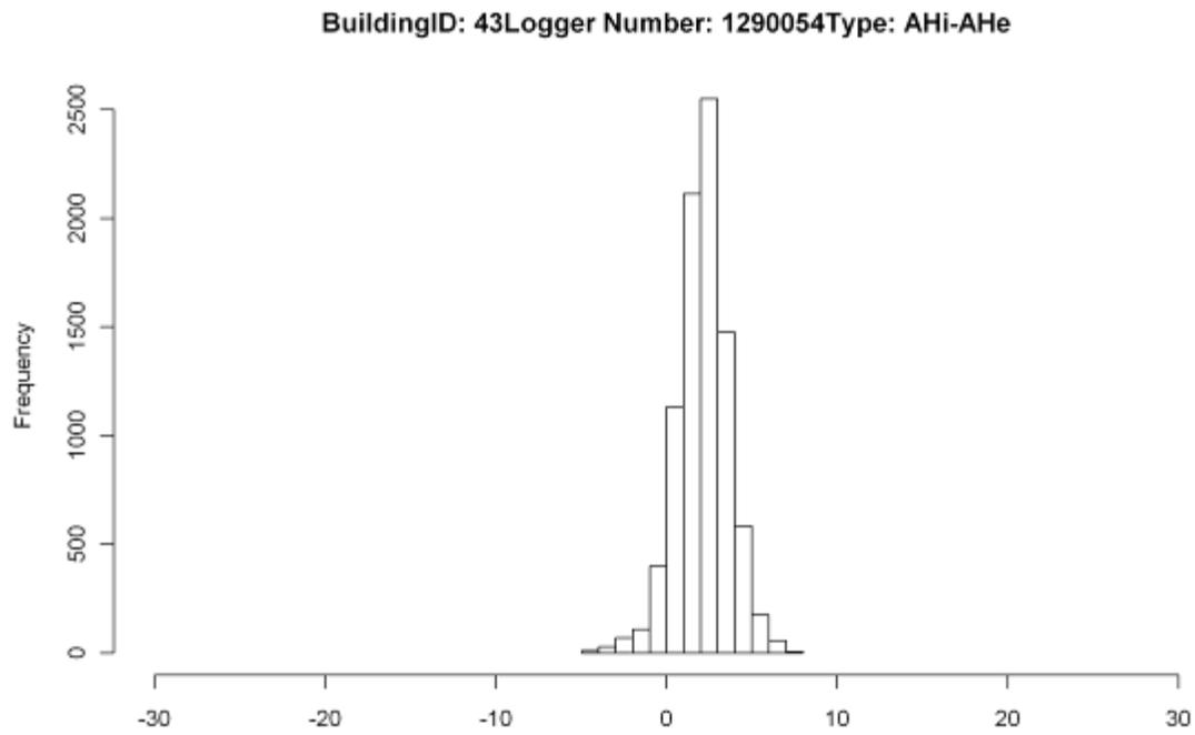
Figure 19: Frequency Plot for the difference in Moisture concentration (Inside –Outside)  $\text{g/m}^3$  for House 43
