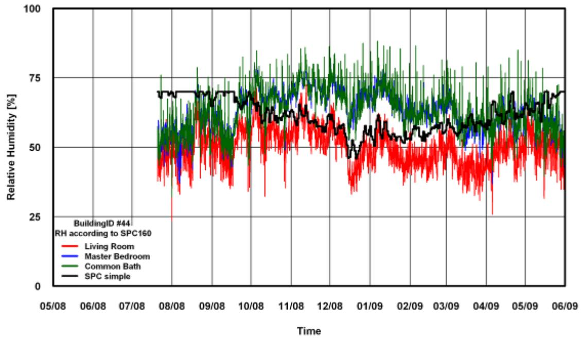
Figure 110: RH Comparison of SPC 160 Simple Method for Building # 44
