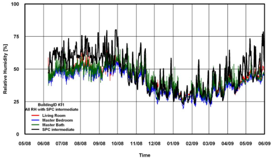
Figure 326: RH Comparison of SPC 160 Intermediate ANK Modified Method for Building # 31
