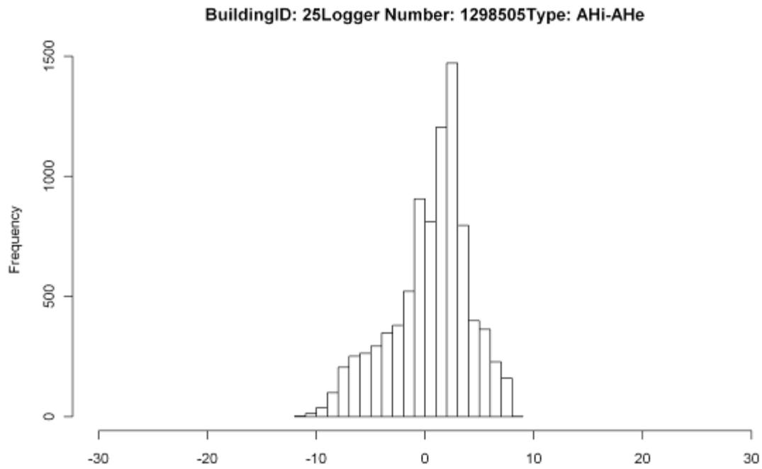
Figure 11: Frequency Plot for the difference in Moisture concentration (Inside –Outside)  $\text{g/m}^3$  for House 25
