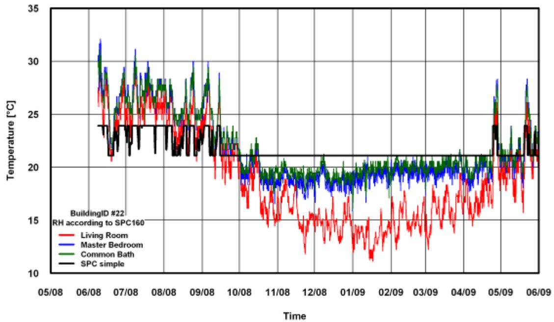
Figure 69: Temperature Comparison of SPC 160 Simple Method for Building # 22
