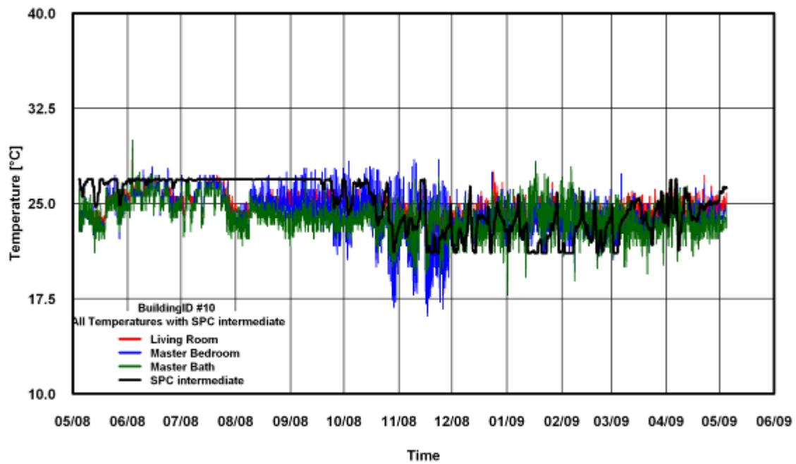
Figure 285: Temperature of SPC 160 Intermediate ANK Modified Method for Building # 10
