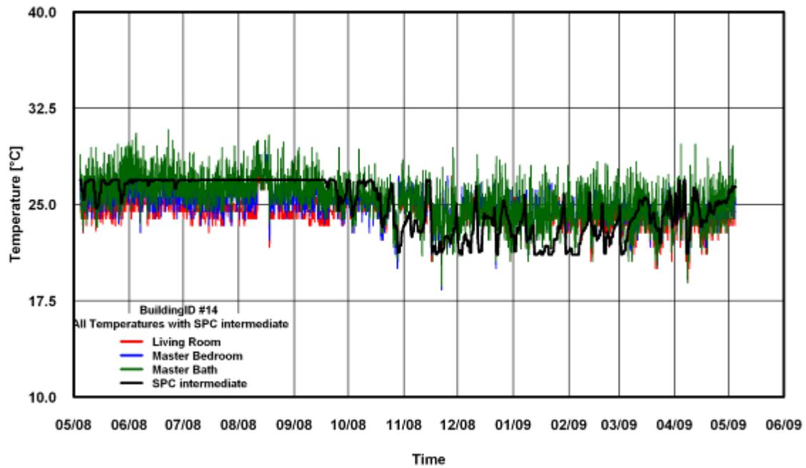
Figure 293: Temperature of SPC 160 Intermediate ANK Modified Method for Building # 14
