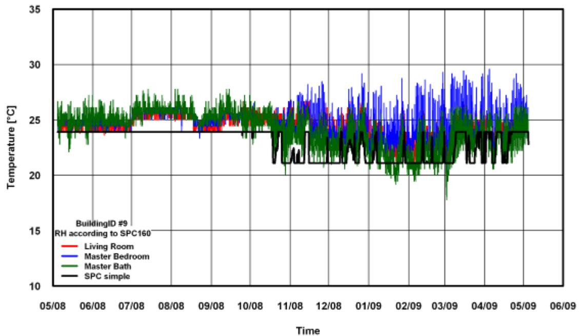
Figure 43: Temperature Comparison of SPC 160 Simple Method for Building #9
