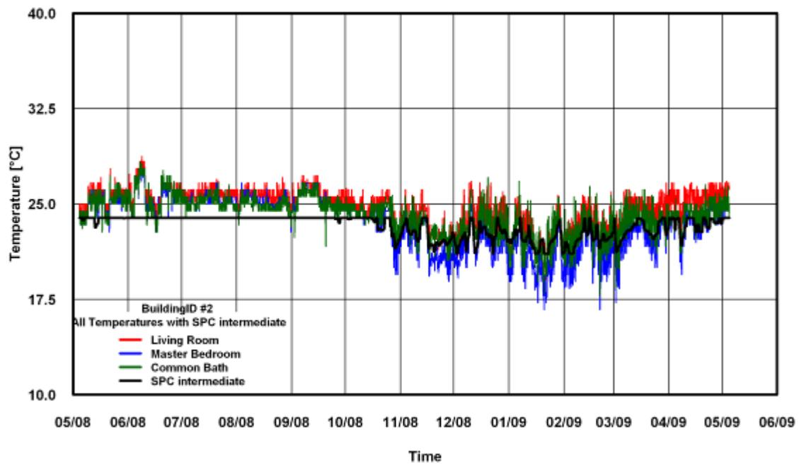
Figure 149: Temperature of SPC 160 Intermediate Method for Building # 2
