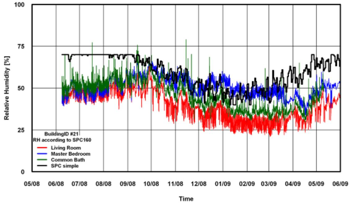
Figure 66: RH Comparison of SPC 160 Simple Method for Building # 21
