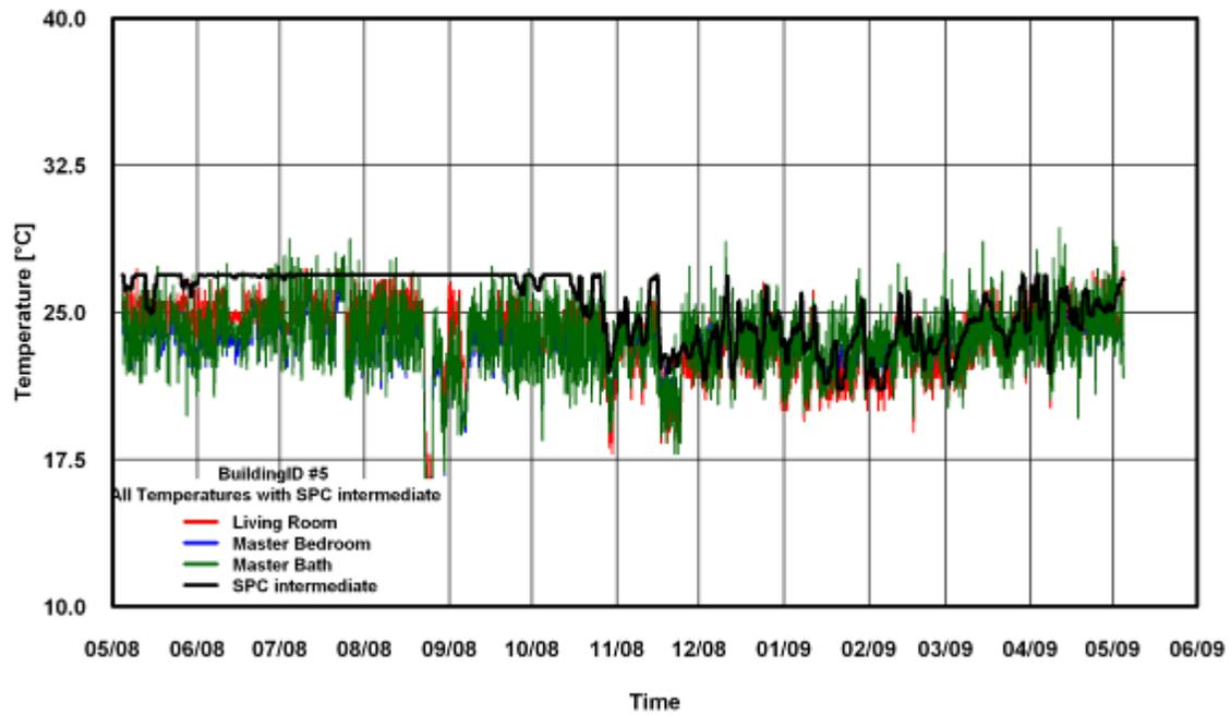
Figure 275: Temperature of SPC 160 Intermediate ANK Modified Method for Building # 5
