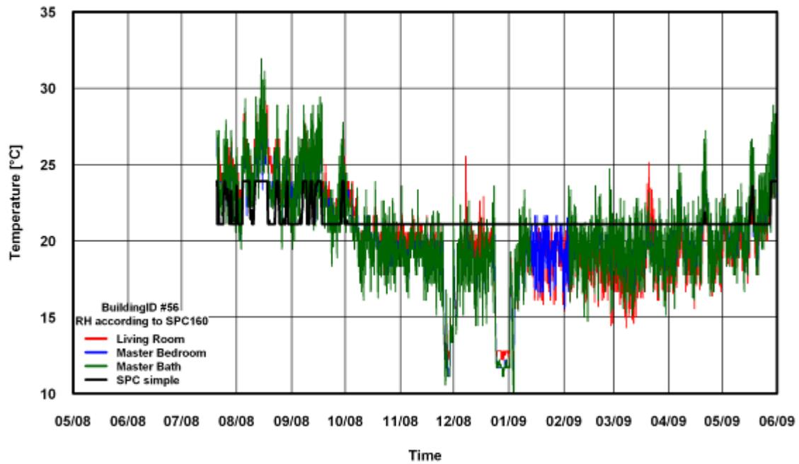
Figure 135: Temperature Comparison of SPC 160 Simple Method for Building # 56
