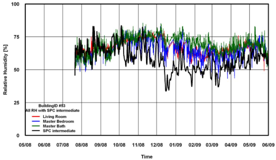
Figure 248: RH Comparison of SPC 160 Intermediate Method for Building # 53
