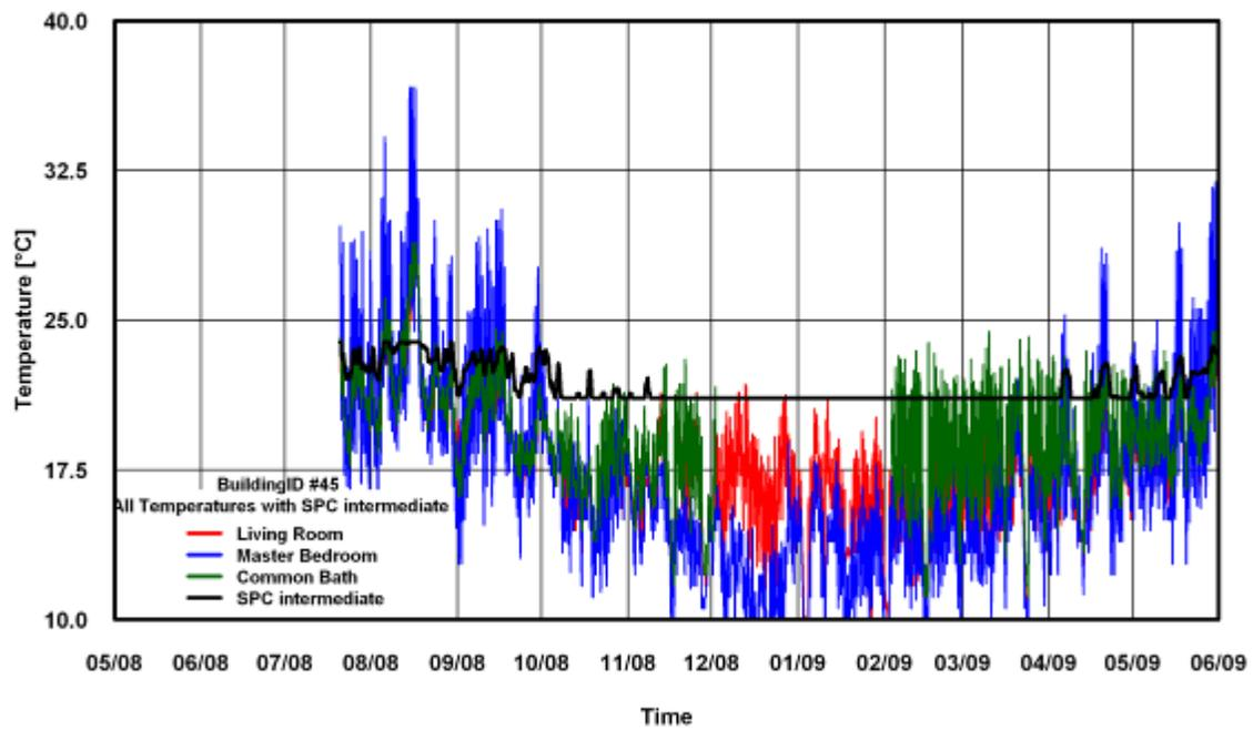
Figure 233: Temperature of SPC 160 Intermediate Method for Building # 45
