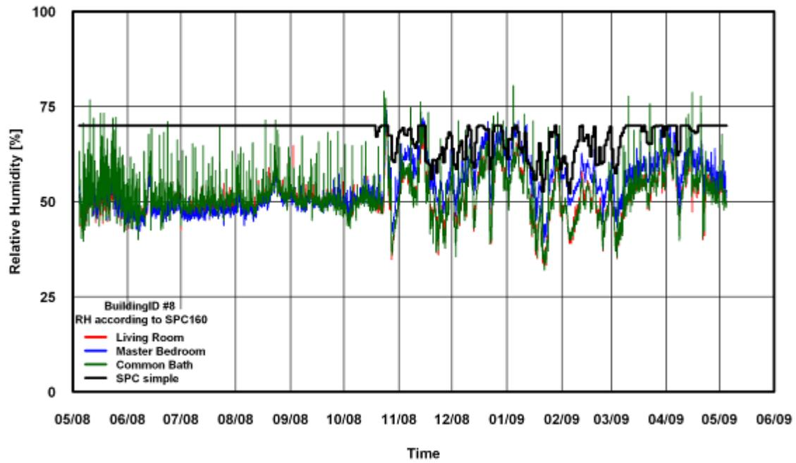
Figure 40: RH Comparison of SPC 160 Simple Method for Building # 8
