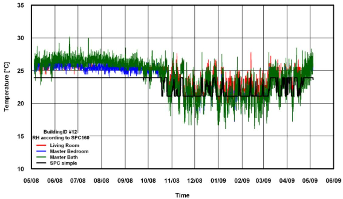
Figure 49: Temperature Comparison of SPC 160 Simple Method for Building # 12
