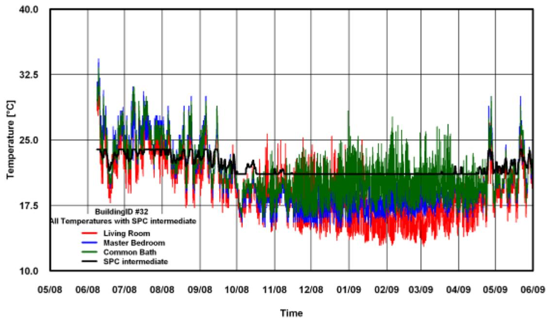
Figure 209: Temperature of SPC 160 Intermediate Method for Building # 32
