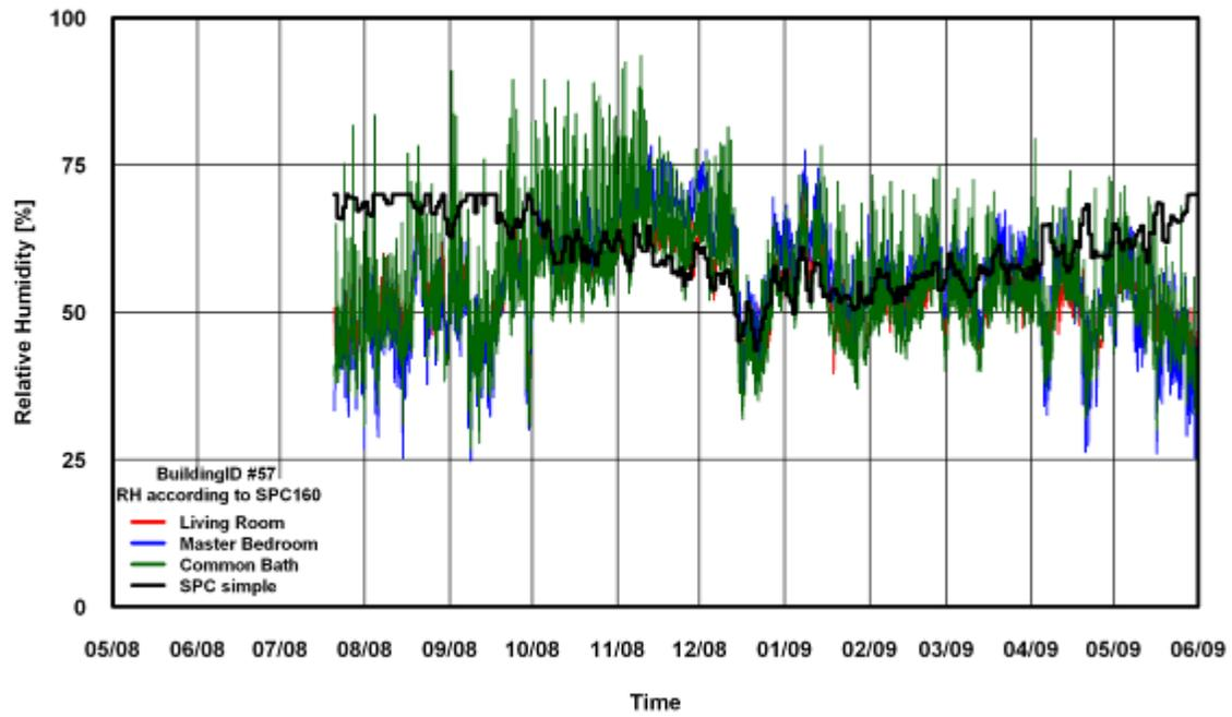
Figure 136: RH Comparison of SPC 160 Simple Method for Building # 57
