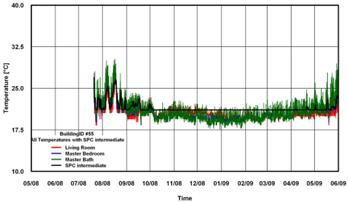
Figure 373: Temperature of SPC 160 Intermediate ANK Modified Method for Building # 55
