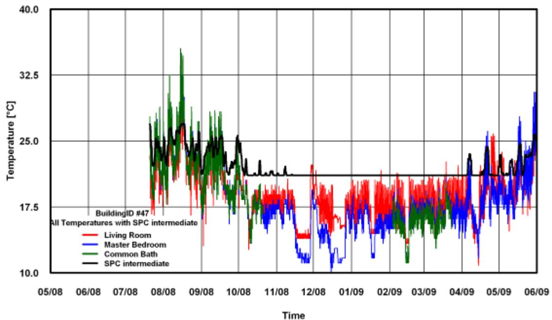
Figure 357: Temperature of SPC 160 Intermediate ANK Modified Method for Building # 47
