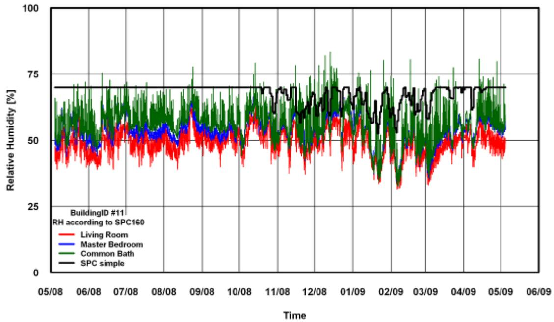
Figure 46: RH Comparison of SPC 160 Simple Method for Building # 11
