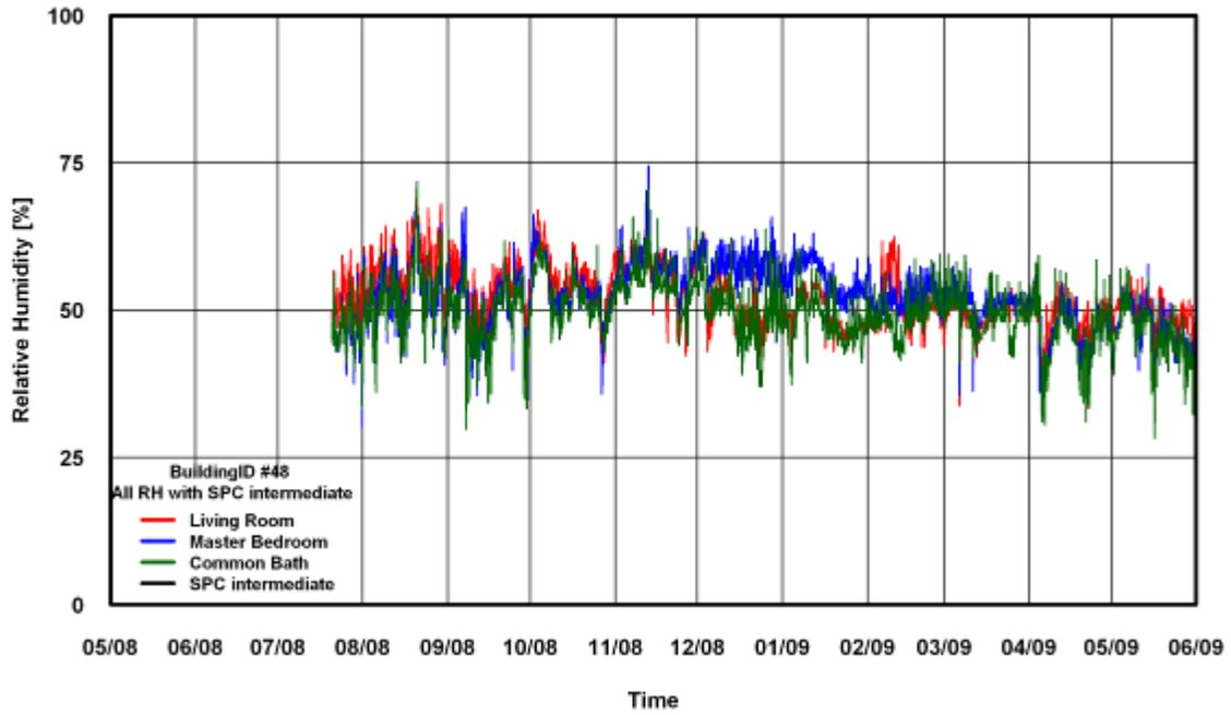
Figure 238: RH Comparison of SPC 160 Intermediate Method for Building # 48
