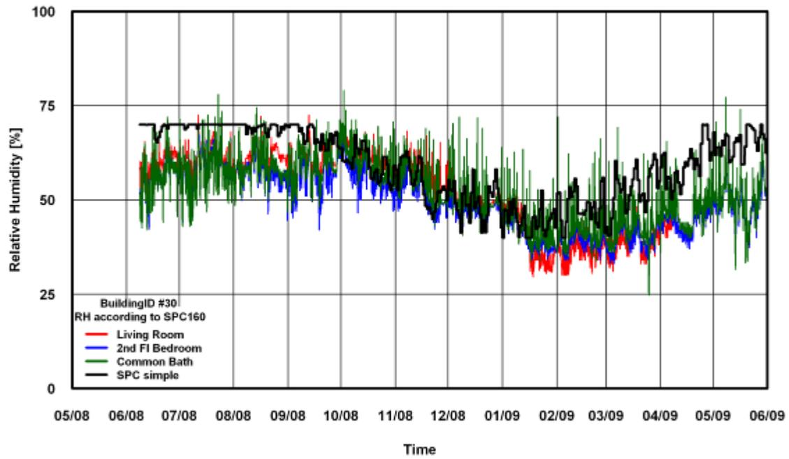
Figure 84: RH Comparison of SPC 160 Simple Method for Building # 30
