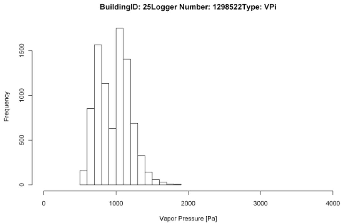
Figure 12: Frequency Plot for the Interior Vapor Pressure (Pa) for House 25
