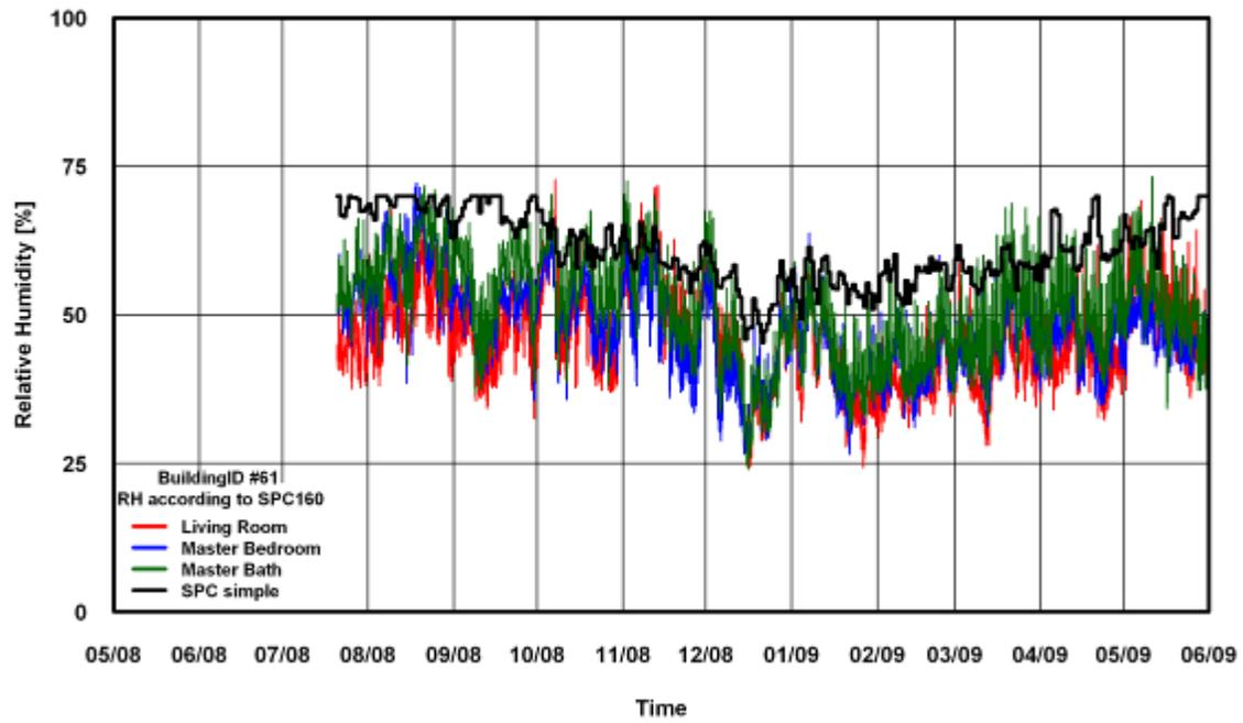
Figure 144: RH Comparison of SPC 160 Simple Method for Building # 61
