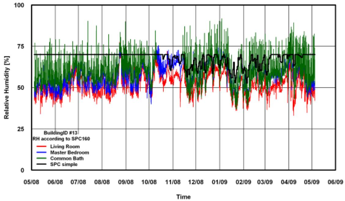
Figure 50: RH Comparison of SPC 160 Simple Method for Building # 13
