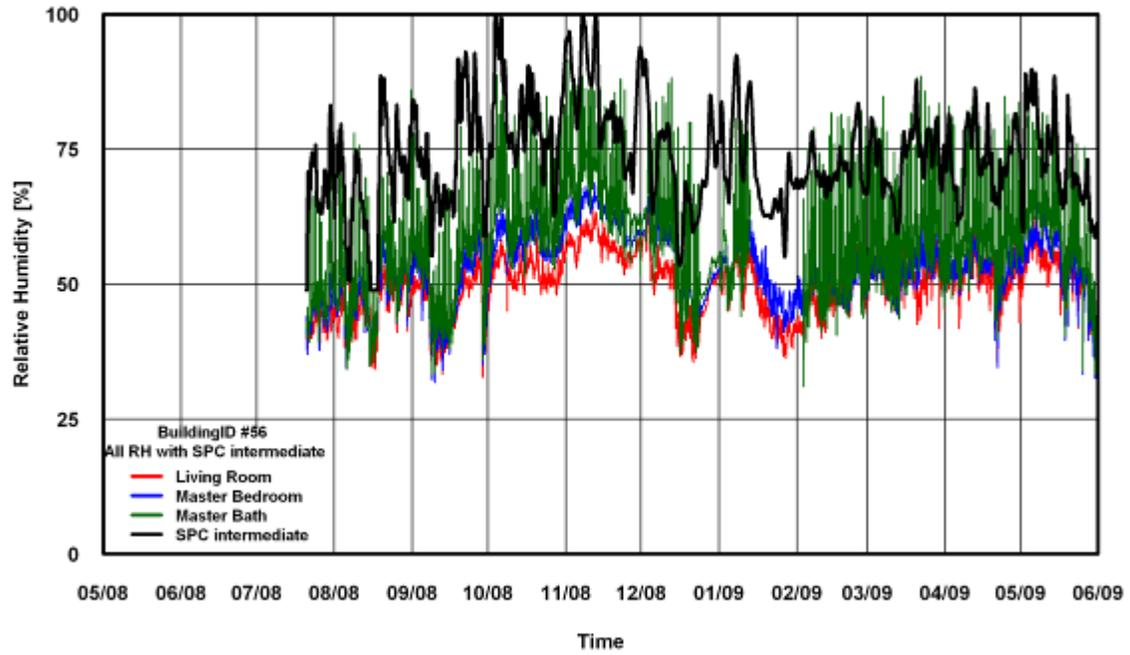
Figure 254: RH Comparison of SPC 160 Intermediate Method for Building # 56
