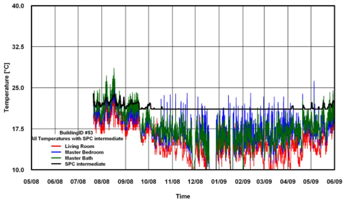
Figure 249: Temperature of SPC 160 Intermediate Method for Building # 53
