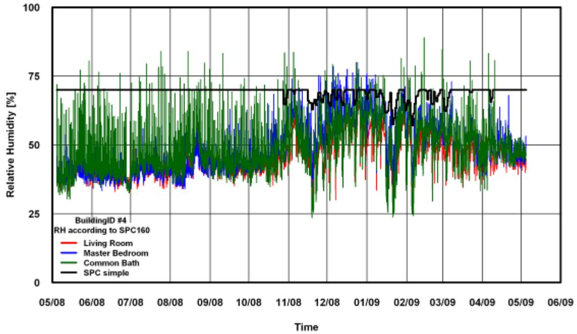
Figure 33: RH Comparison of SPC 160 Simple Method for Building # 4
