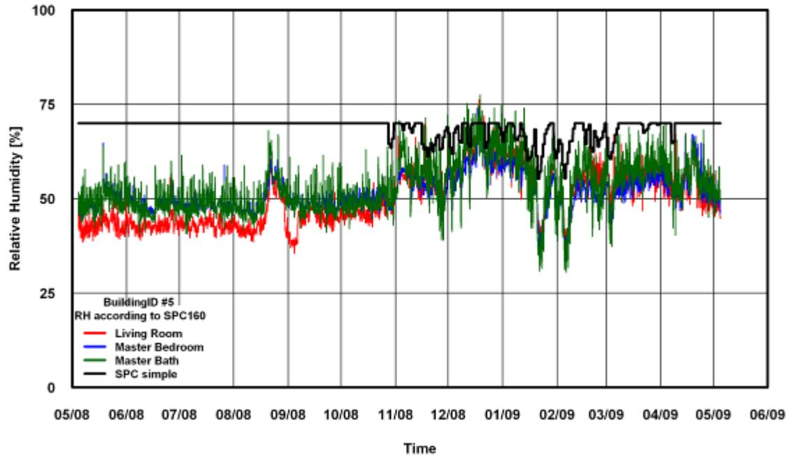
Figure 35: RH Comparison of SPC 160 Simple Method for Building # 5
