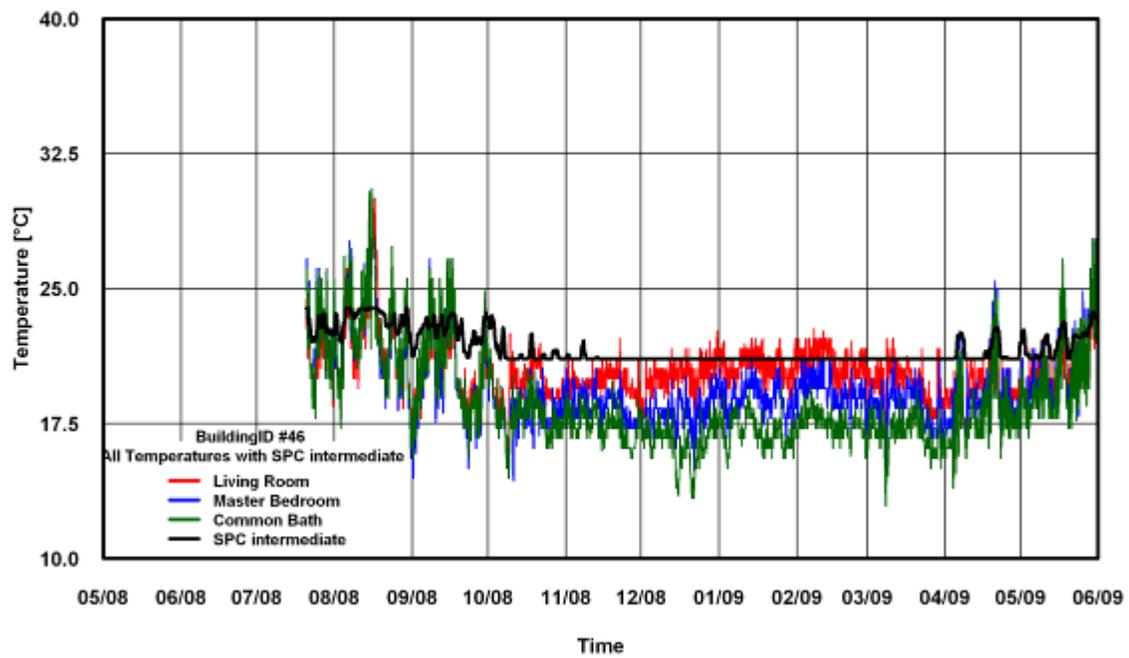
Figure 235: Temperature of SPC 160 Intermediate Method for Building # 46
