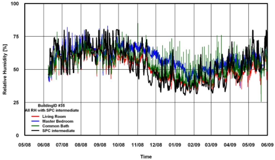
Figure 334: RH Comparison of SPC 160 Intermediate ANK Modified Method for Building # 35
