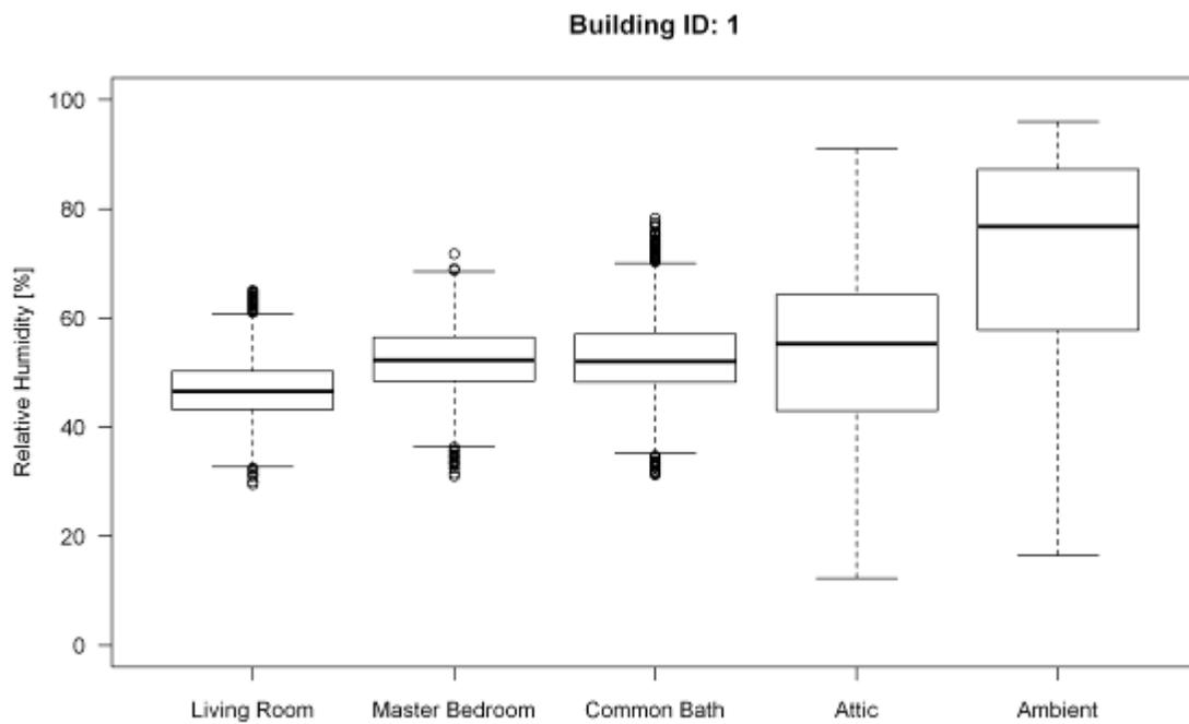
Figure 6: Box Plot for the Interior Relative Humidity (-) for House 1
