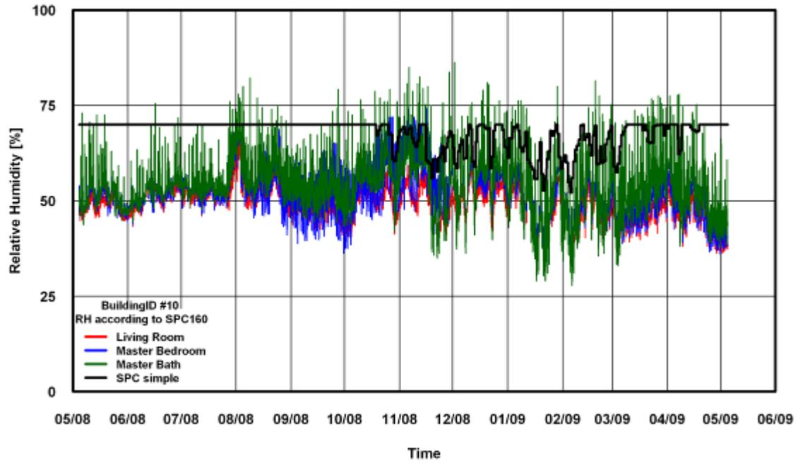
Figure 44: RH Comparison of SPC 160 Simple Method for Building # 10
