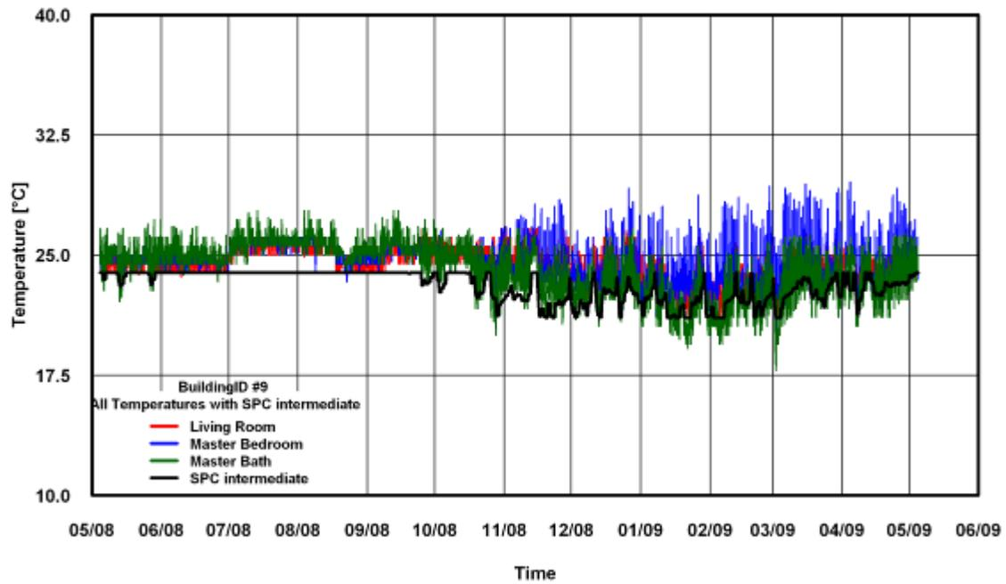
Figure 163: Temperature of SPC 160 Intermediate Method for Building # 9
