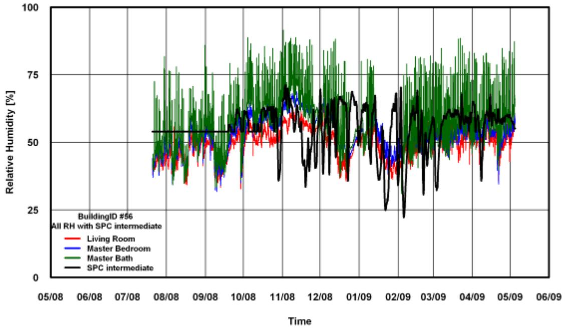
Figure 374: RH Comparison of SPC 160 Intermediate ANK Modified Method for Building # 56
