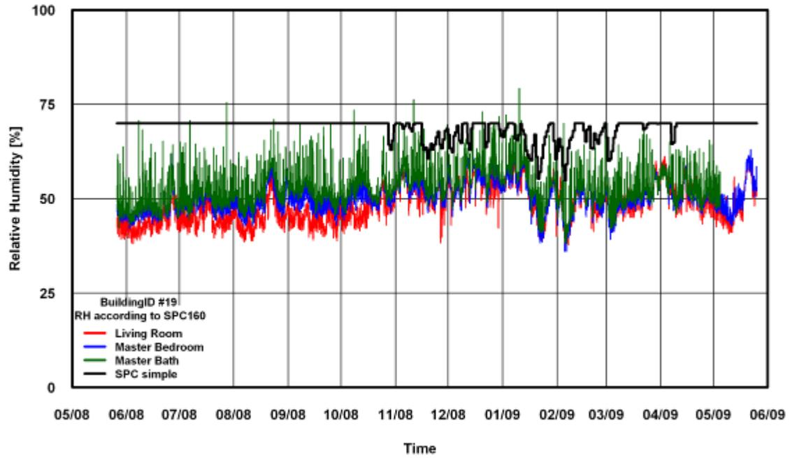
Figure 62: RH Comparison of SPC 160 Simple Method for Building # 19
