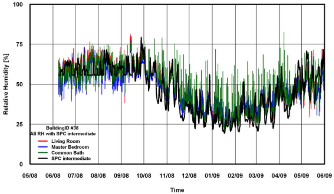
Figure 220: RH Comparison of SPC 160 Intermediate Method for Building # 38
