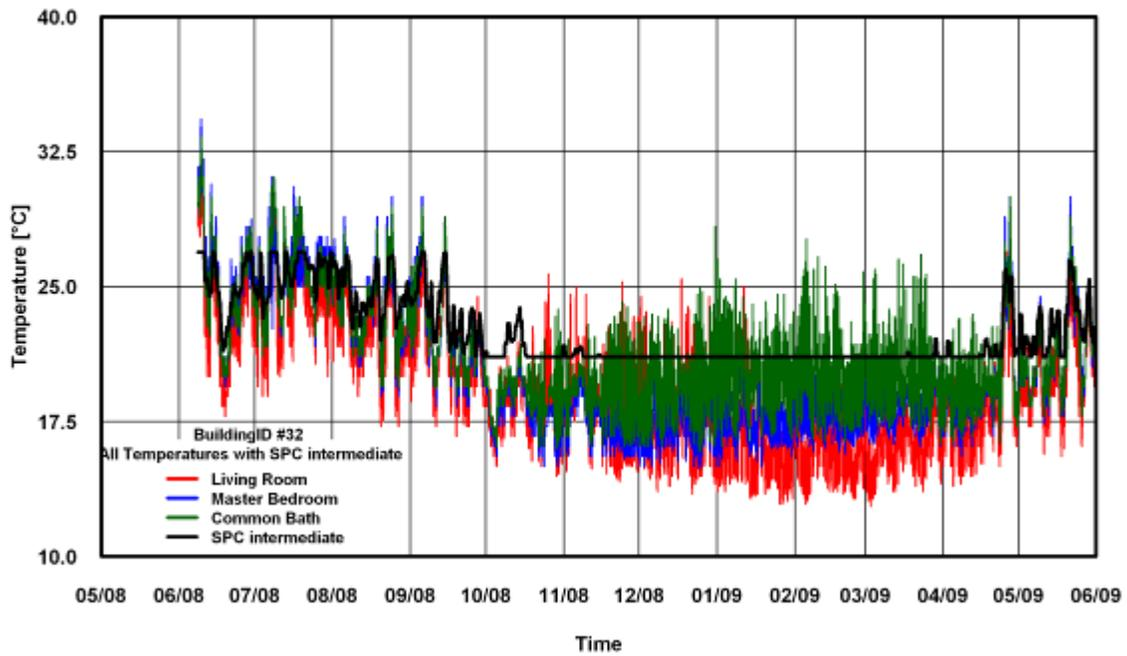
Figure 329: Temperature of SPC 160 Intermediate ANK Modified Method for Building # 32
