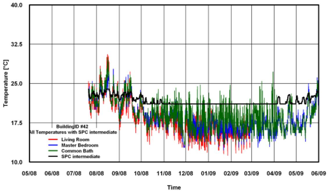
Figure 227: Temperature of SPC 160 Intermediate Method for Building # 42
