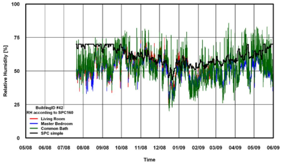
Figure 106: RH Comparison of SPC 160 Simple Method for Building # 42
