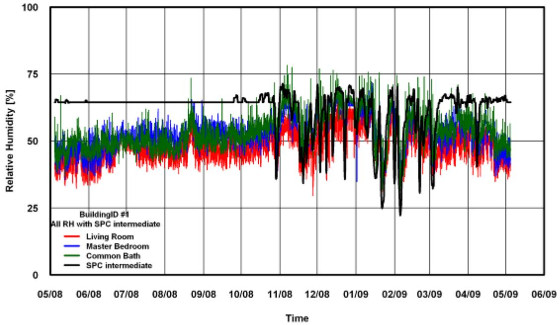
Figure 146: RH Comparison of SPC 160 Intermediate Method for Building # 1
