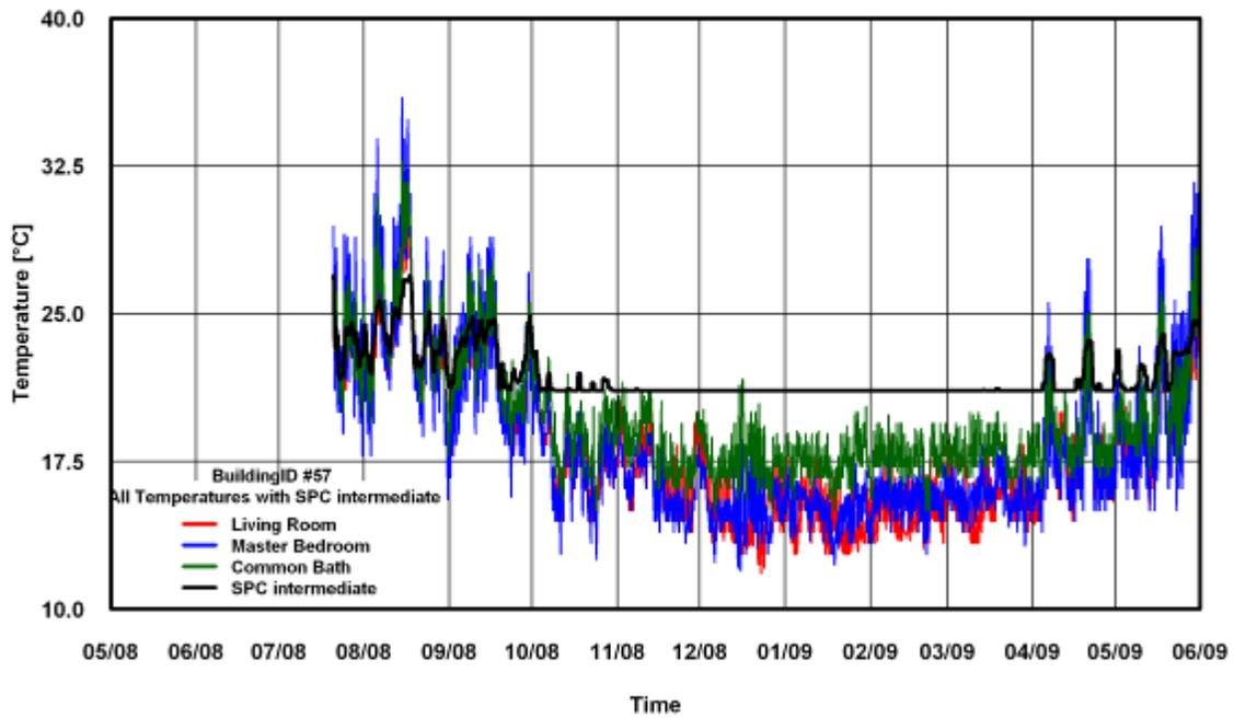
Figure 377: Temperature of SPC 160 Intermediate ANK Modified Method for Building # 57
