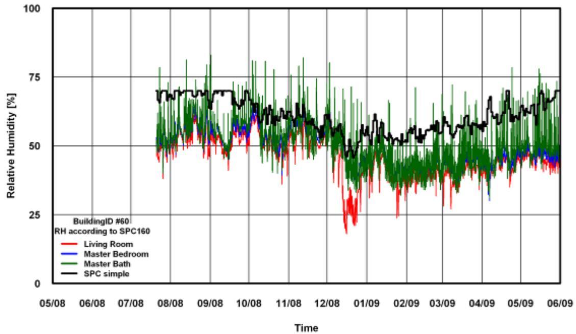
Figure 142: RH Comparison of SPC 160 Simple Method for Building # 60
