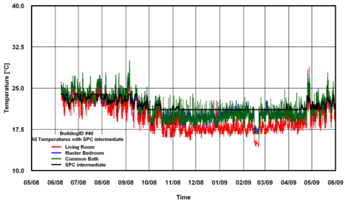
Figure 225: Temperature of SPC 160 Intermediate Method for Building # 40
