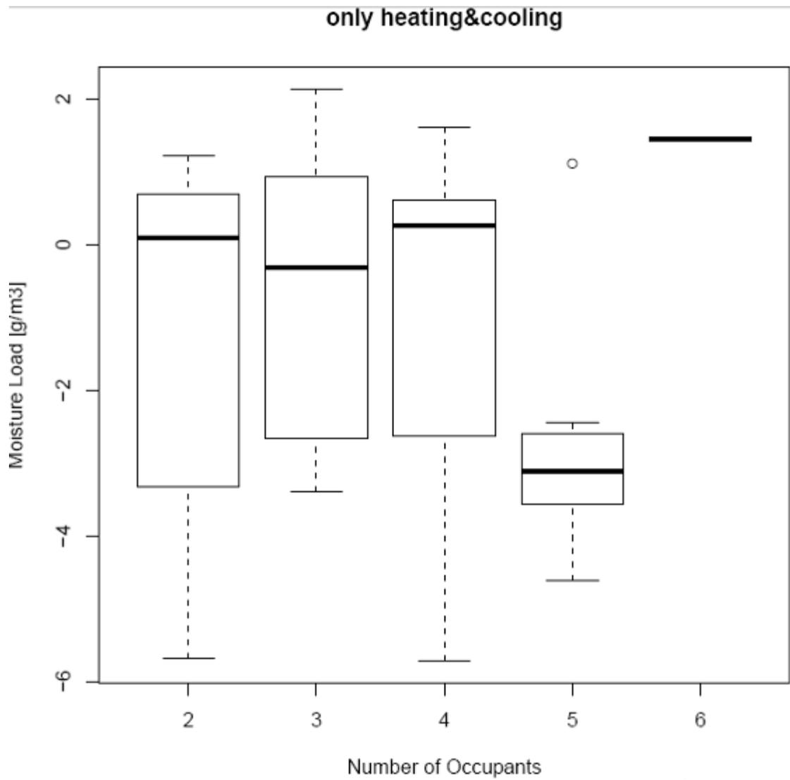
**Figure 391: Impact of Number of Occupants on Moisture Load ( $\text{g}/\text{m}^3$ )**
