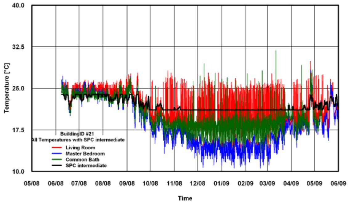
Figure 187: Temperature of SPC 160 Intermediate Method for Building # 21
