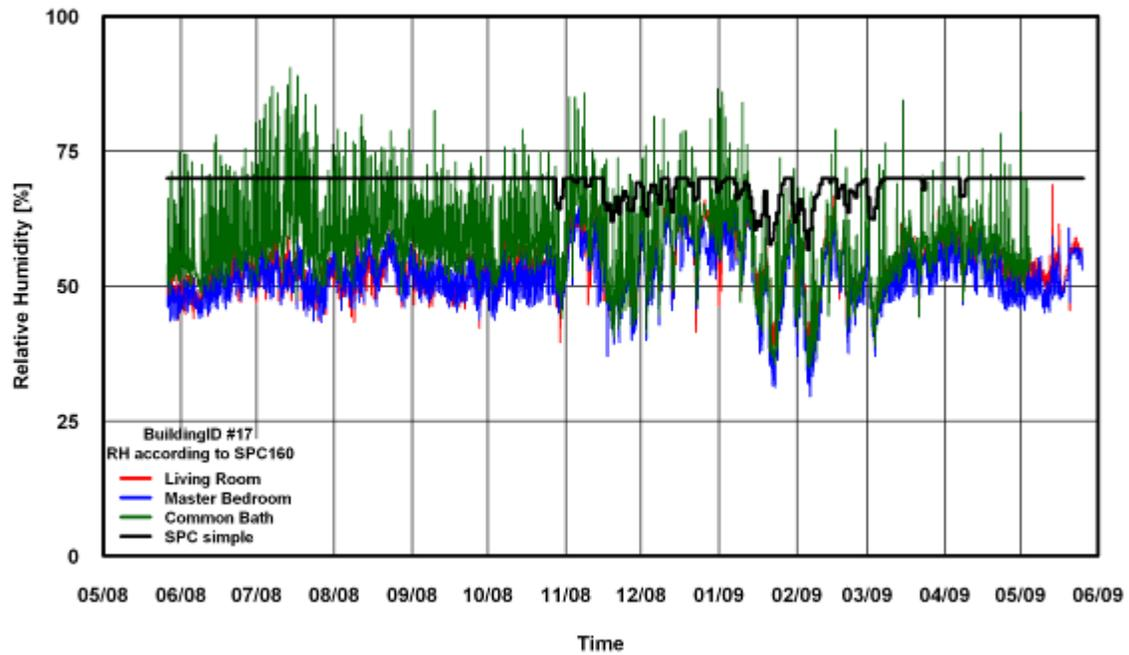
Figure 58: RH Comparison of SPC 160 Simple Method for Building # 17
