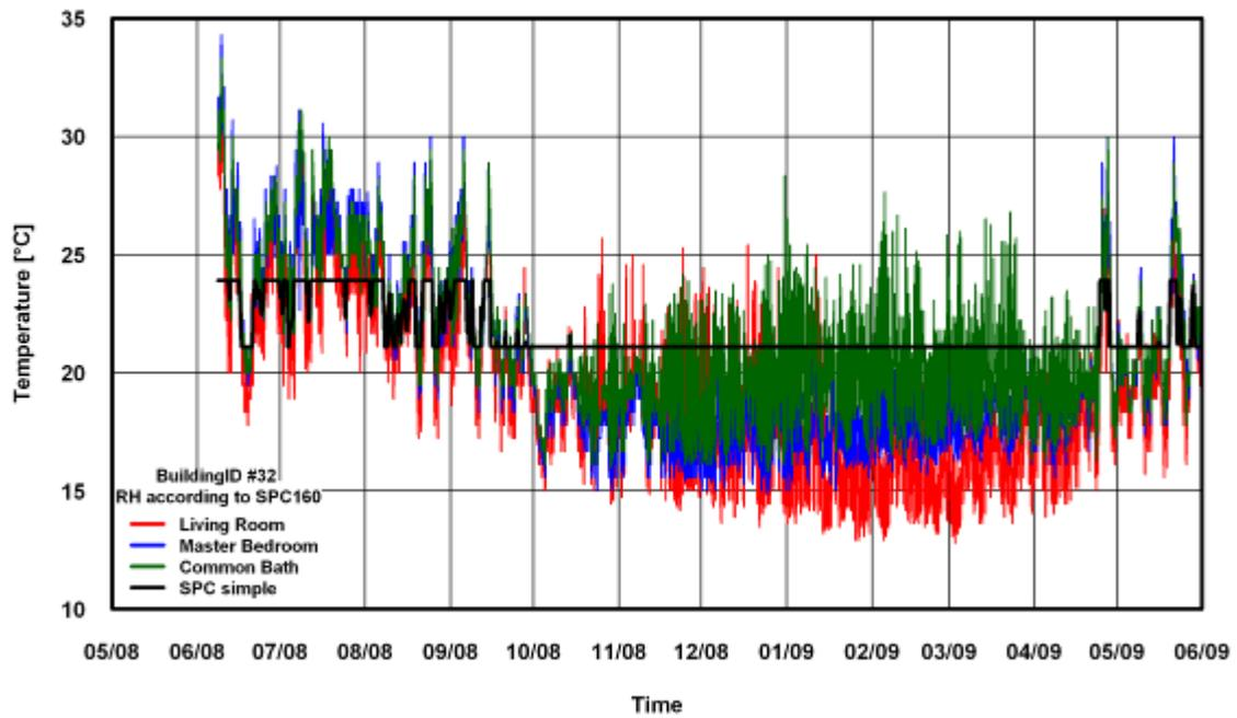
Figure 89: Temperature Comparison of SPC 160 Simple Method for Building # 32
