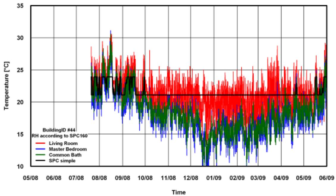
Figure 111: Temperature Comparison of SPC 160 Simple Method for Building # 44
