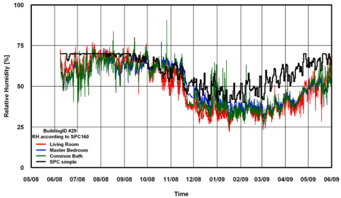
Figure 82: RH Comparison of SPC 160 Simple Method for Building # 29
