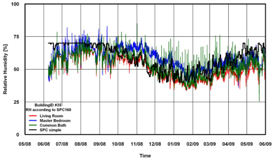
Figure 94: RH Comparison of SPC 160 Simple Method for Building # 35
