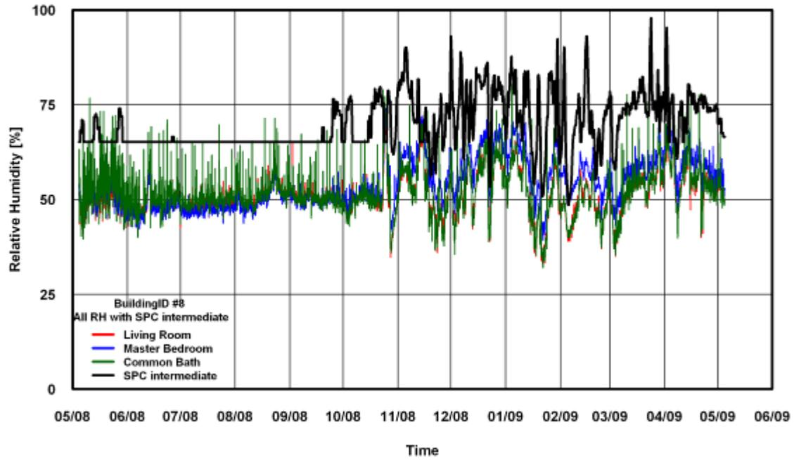
Figure 160: RH Comparison of SPC 160 Intermediate Method for Building # 8
