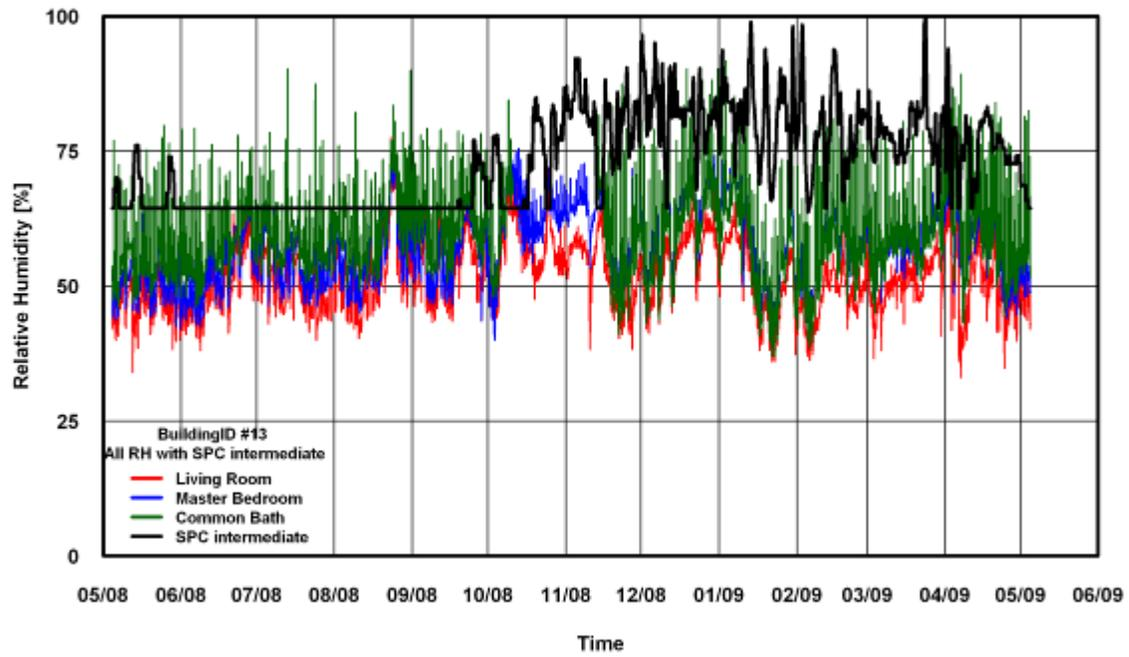
Figure 170: RH Comparison of SPC 160 Intermediate Method for Building # 13
