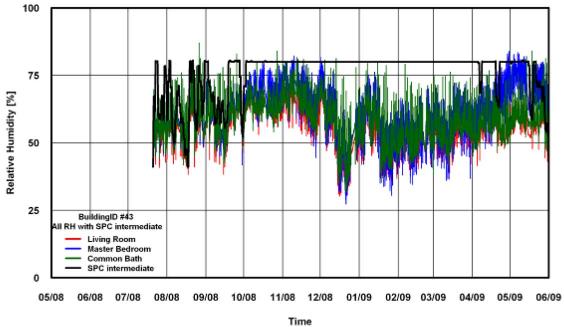
Figure 348: RH Comparison of SPC 160 Intermediate ANK Modified Method for Building # 43
