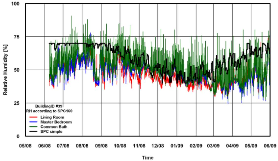
Figure 102: RH Comparison of SPC 160 Simple Method for Building # 39
