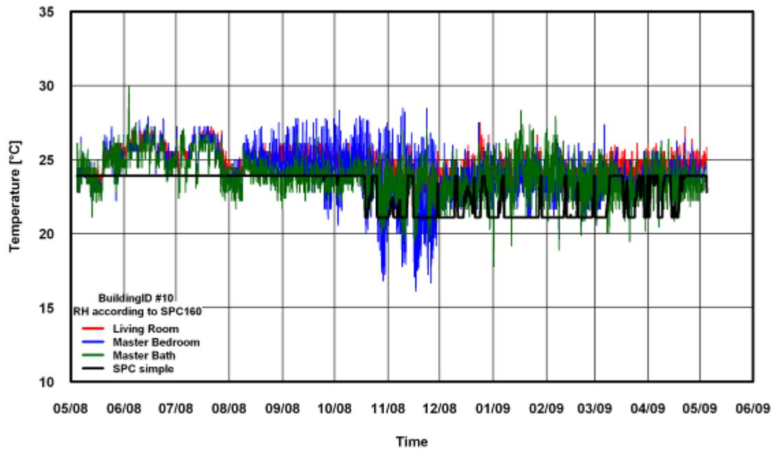
Figure 45: Temperature Comparison of SPC 160 Simple Method for Building # 10
