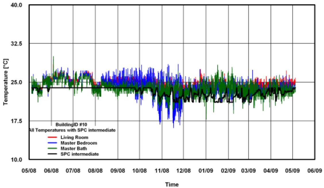
Figure 165: Temperature of SPC 160 Intermediate Method for Building # 10
