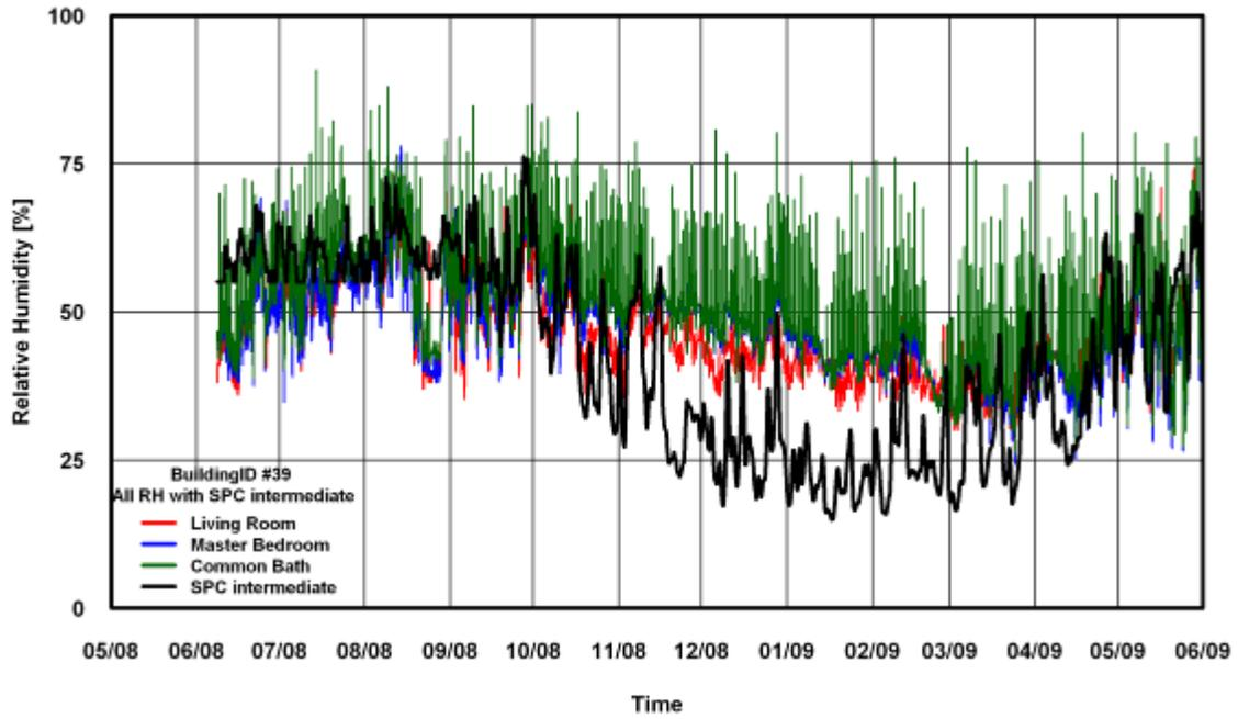
Figure 222: RH Comparison of SPC 160 Intermediate Method for Building # 39
