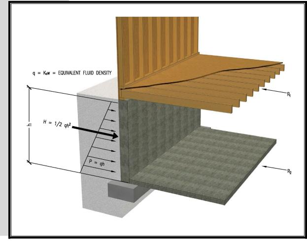
For the triangular pressure distribution shown in figure 3.1, the pressure, P in psf, at depth, h in feet, is determined by equation 3.5-2, and the resultant force, H in lbs, at depth, h in feet, is determined by equation 3.5-3. The factor q is the EFD as discussed above.
