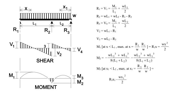
Figure A.17. Continuous Beam—Two Unequal Spans and Uniformly Distributed Load
