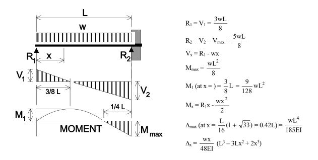
Figure A.9. Beam Fixed at One End, Supported at Other—Uniformly Distributed Load
