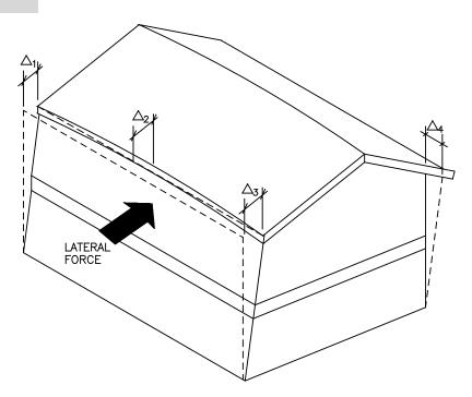
NOTE: IF STIFFNESS OR LOAD IS NONSYMMETRICAL, BUILDING ROTATION OCCURS ( $\Delta_1 \neq \Delta_3$ ) AND LOADS ARE DISTRIBUTED BY TORSION ( $\Delta_4 \neq 0$ ) AS WELL AS BY DIRECT SHEAR IN THE DIRECTION OF THE LATERAL FORCE. THIS CONDITION VARIES BUT IS A REALITY FOR MOST DESIGNS.  $\Delta_2$  IS THE BENDING DEFORMATION OF THE HORIZONTAL DIAPHRAGM (I.E., ROOF).
