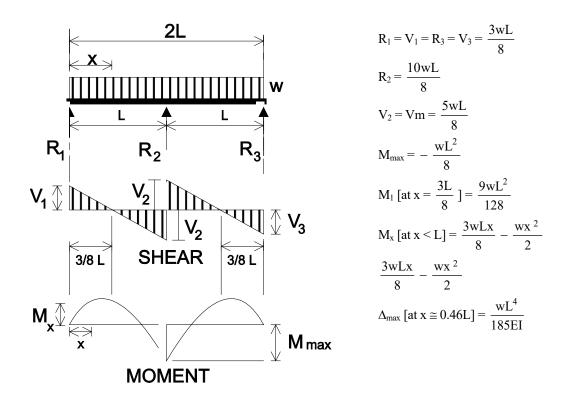
Figure A.15 Continuous Beam—Two Equal Spans and Uniformly Distributed Load
