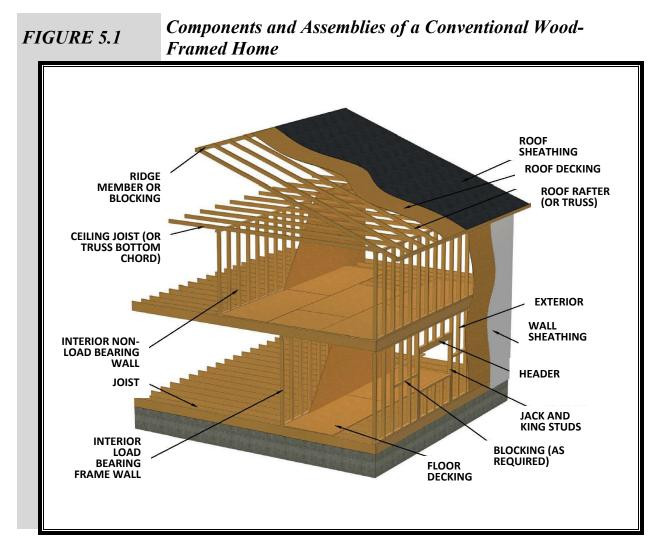
Each system can be complex to design as a whole; therefore, simple analysis usually focuses on the individual elements (subassemblies) that constitute the system. In some cases, "system effects" may be considered in simplified form and applied to the design of certain elements that constitute specifically defined systems. Structural elements that make up a residential structural system include—
