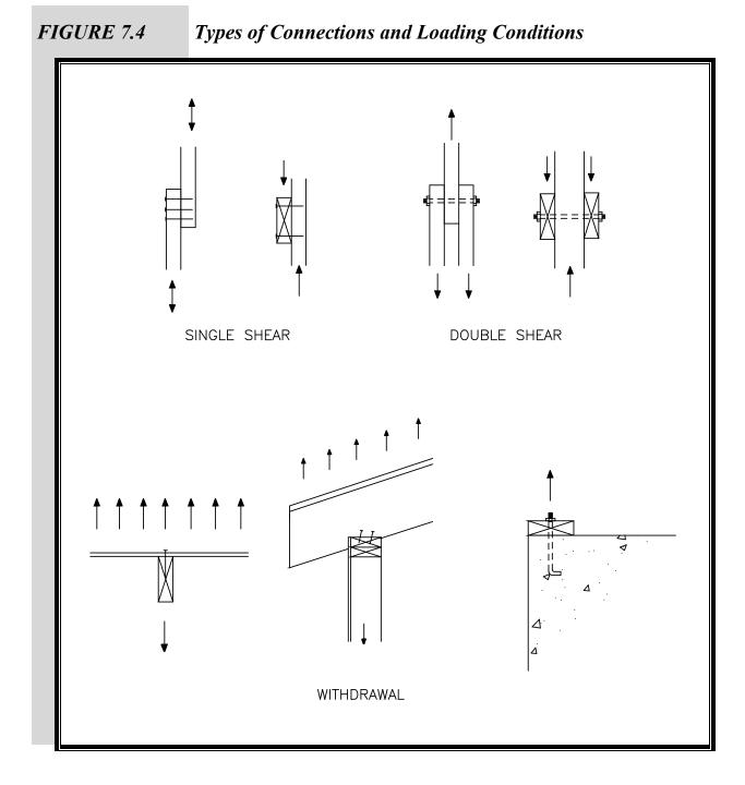
The NDS provides tabulated connection design values that use the following symbols for the three basic types of loading.
