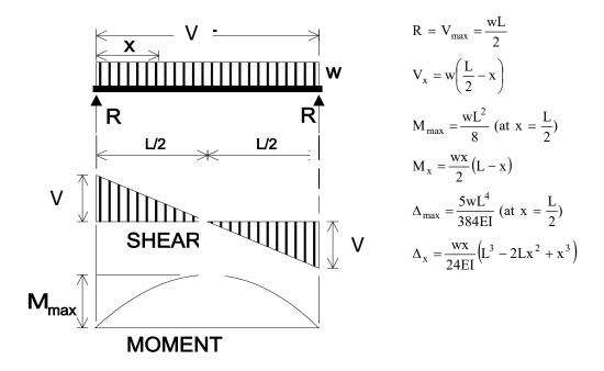
Figure A.3. Simple Beam—Uniformly Distributed Load
