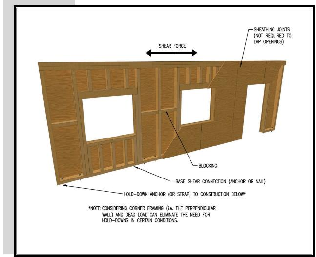
FIGURE 6.7 Basic Perforated Shear Wall
