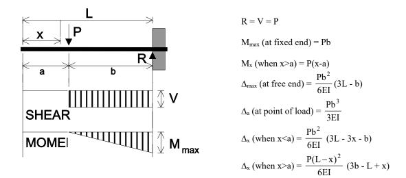
Figure A.8. Cantilever Beam—Concentrated Load at Any Point
