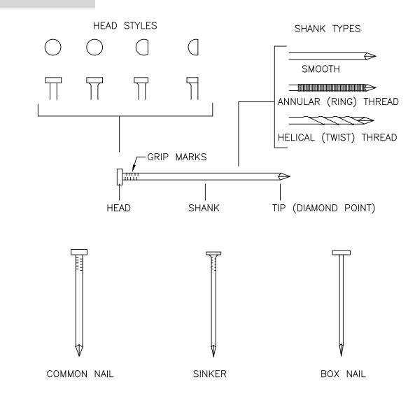
The following are the most common nail types used in residential wood construction.
