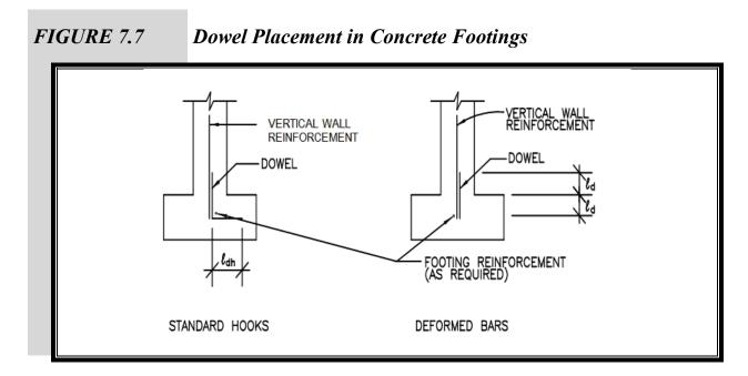
The minimum embedment length is a limit specified in ACI-318 that is not necessarily compatible with residential construction conditions and practice; therefore, this guide suggests a minimum embedment length of 6 to 8 inches for
