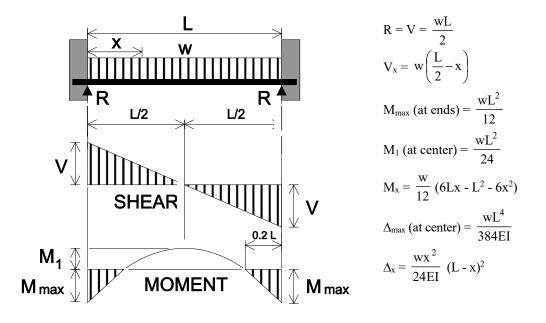
Figure A.11. Beam Fixed at Both Ends—Uniformly Distributed Load
