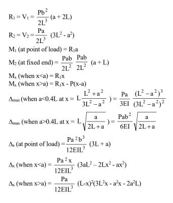
Figure A.10. Beam Fixed at One End, Supported at Other—Concentrated Load at Any Point
