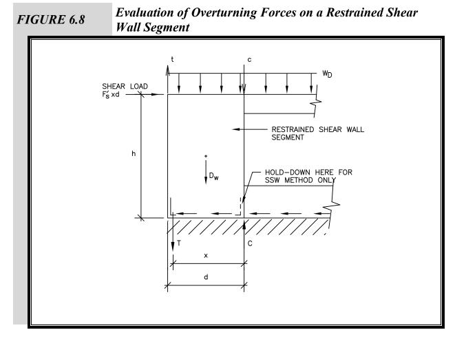
For a more simplified analysis of overturning forces, the effect of dead load may be neglected (the normal case in practice) and the chord forces determined as follows, using the symbols defined as before.
