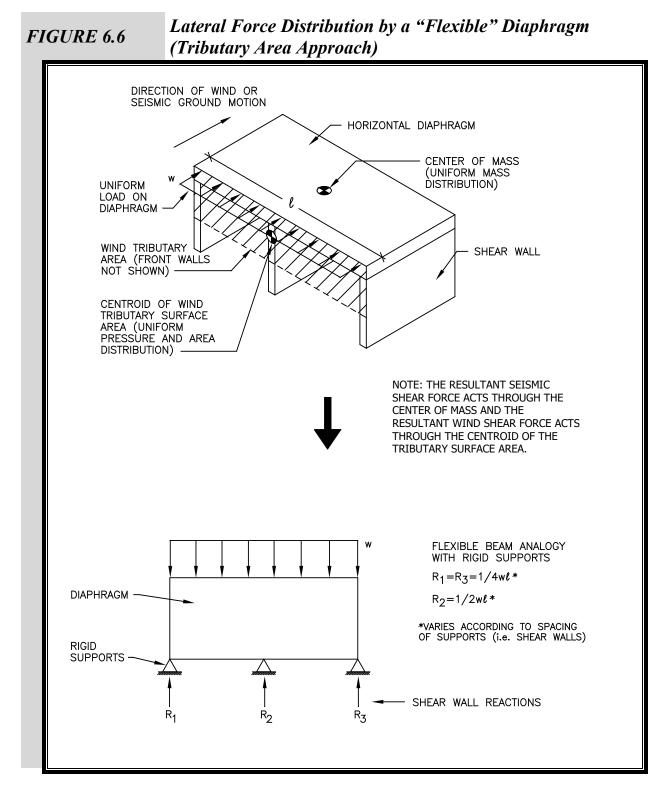
In seismic design, tributary areas are associated with uniform area weights assigned to the building systems (that is, roof, walls, and floors) that generate the inertial seismic load when the building is subject to lateral ground motion (refer to chapter 3 on earthquake loads). In wind design, the tributary areas are associated
