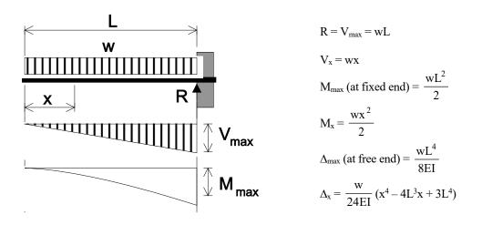
Figure A.7. Cantilever Beam—Uniformly Distributed Load
