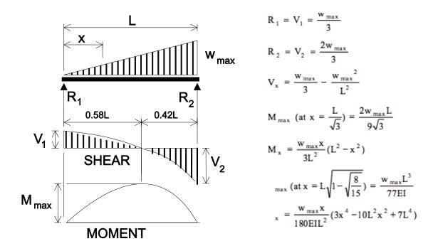
Figure A.4. Simple Beam—Load Increasing Uniformly to One End
