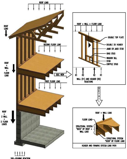
SOIL-BEARING REACTION (= ROOF + 2 WALLS + 2 FLOORS
