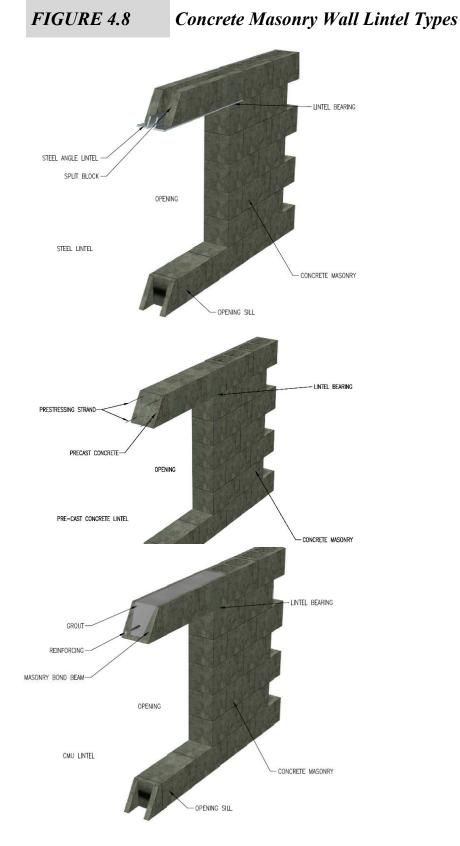
minimum 1/4-inch thick. Figure 4.8 illustrates some lintels commonly used in residential masonry construction.
