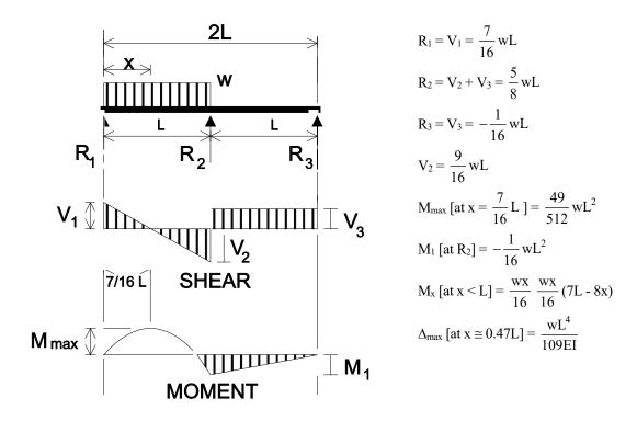
Figure A.16. Continuous Beam—Two Equal Spans With Uniform Load on One Span
