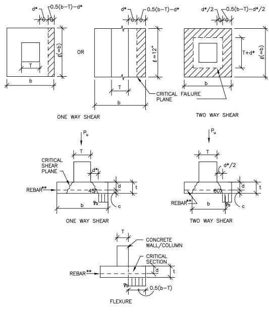
NOTES: \* SUBSTITUTE t FOR d AS REQUIRED FOR PLAIN CONCRETE FOOTING DESIGN \*\* REBAR IS REQUIRED ONLY IN REINFORCED CONCRETE FOOTING DESIGN AND IS SHOWN HERE FOR THAT PURPOSE ONLY. IN REINFORCED SQUARE FOOTINGS, THE REBAR MUST BE PLACED IN TWO DIRECTIONS.
