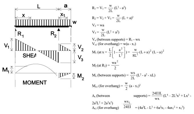
Figure A.13. Beam Overhanging One Support—Uniformly Distributed Load
