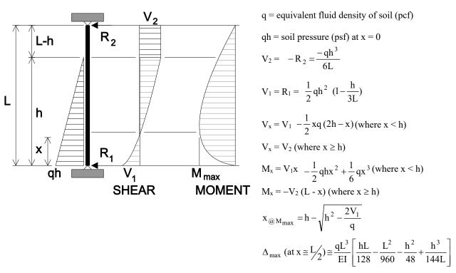
Figure A.1. Simple Beam (Foundation Wall)—Partial Triangular Load
