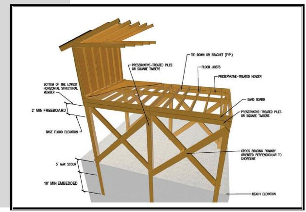
FIGURE 4.11 Basic Coastal Foundation Construction
