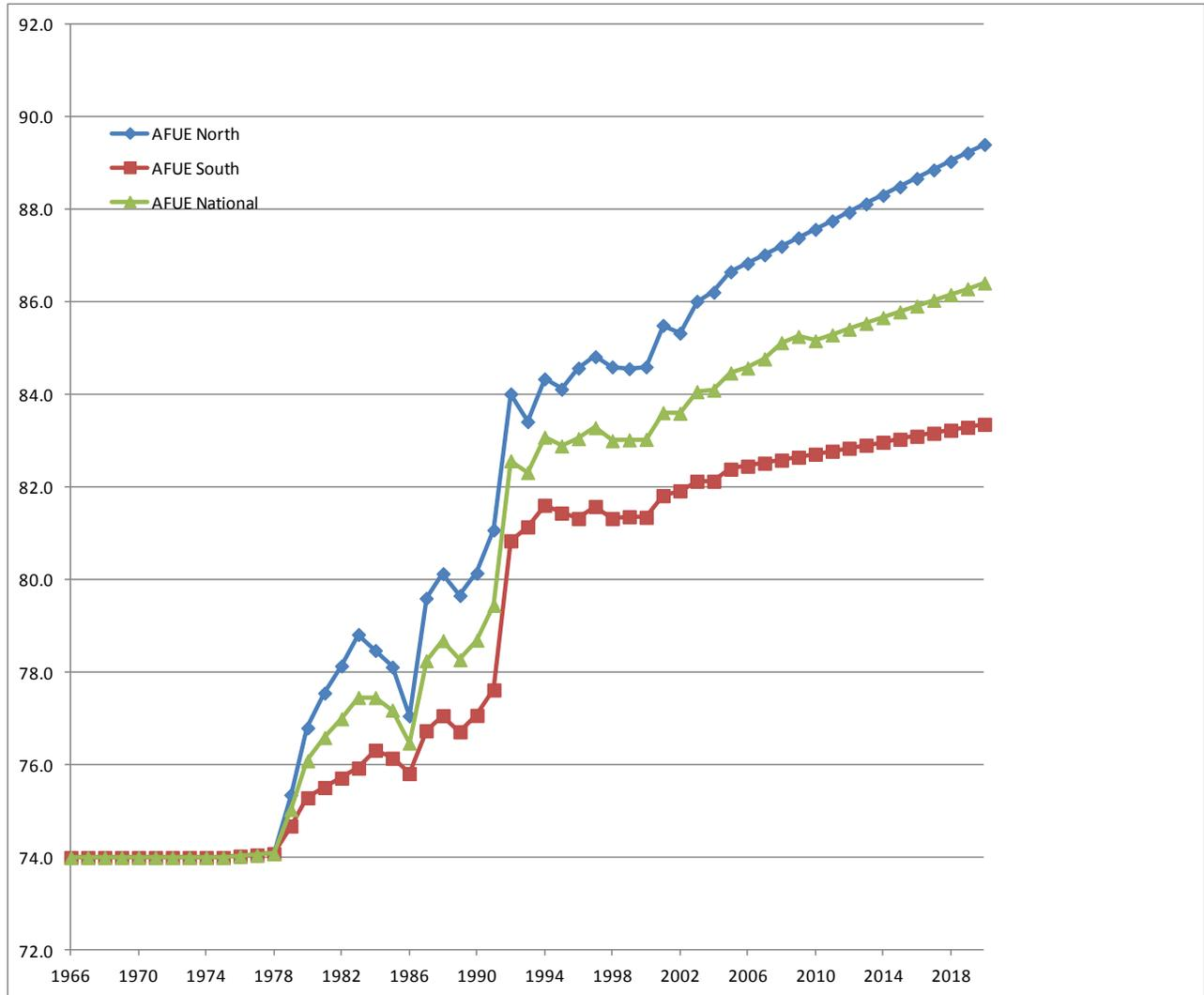
Figure 12. Estimated Shipment Weighted Furnace AFUE
