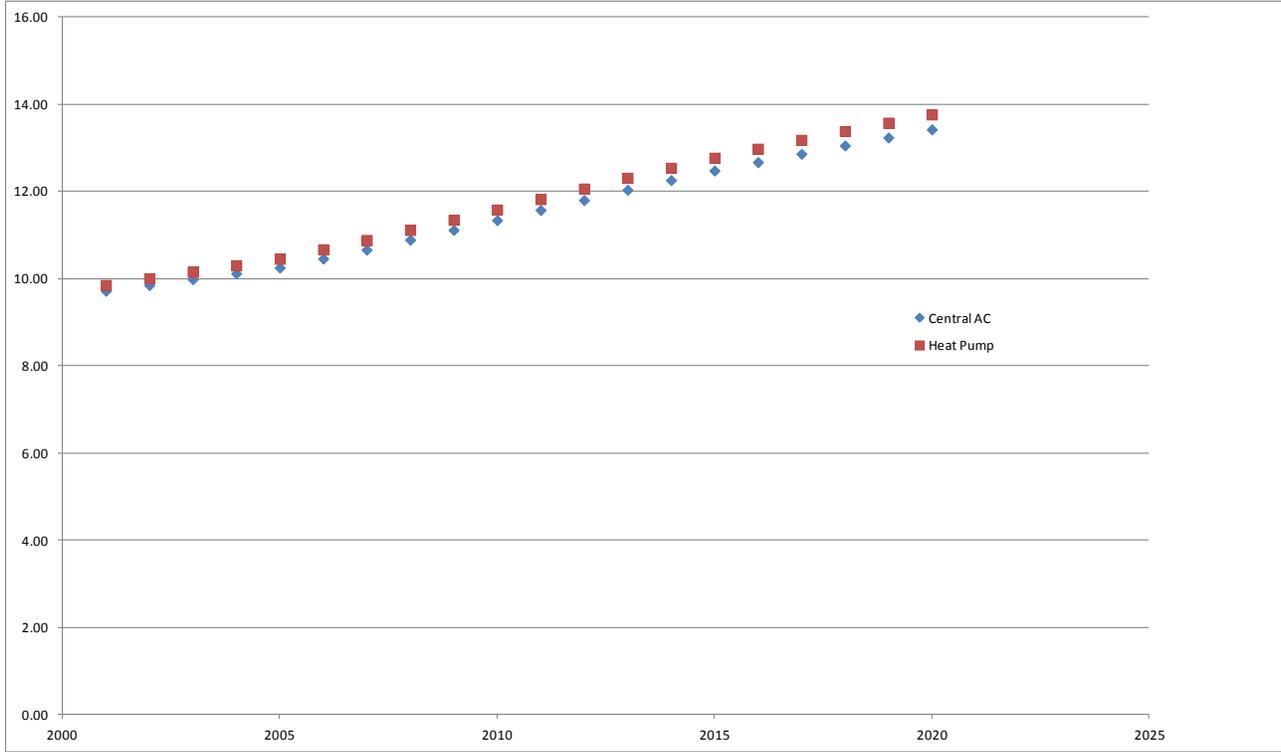
Figure 7. Estimated Average Cooling Efficiency Installed in Residences
