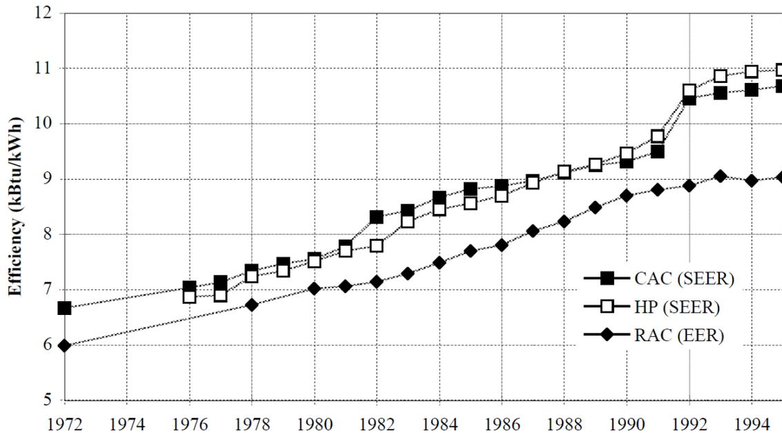
Figure 4. Shipment Weighted Efficiencies for Cooling Equipment 1972-1995
