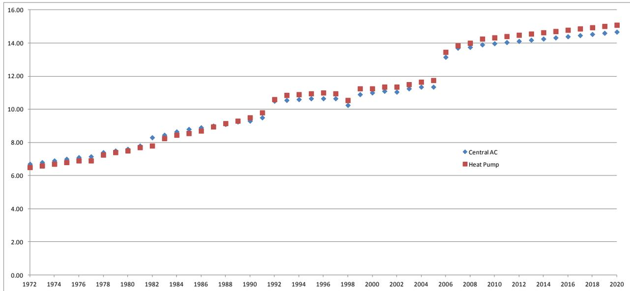
*Figure 5. Estimated Shipment Weighted Cooling Efficiencies*
