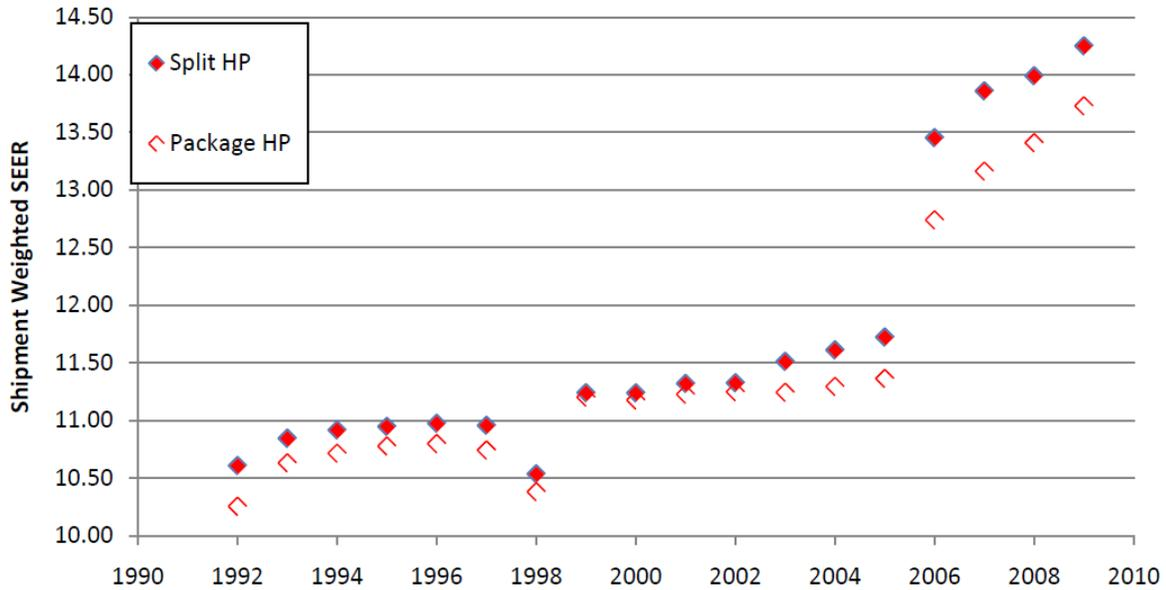
Figure 3. Heat Pump Historical Shipment-Weighted Efficiencies
