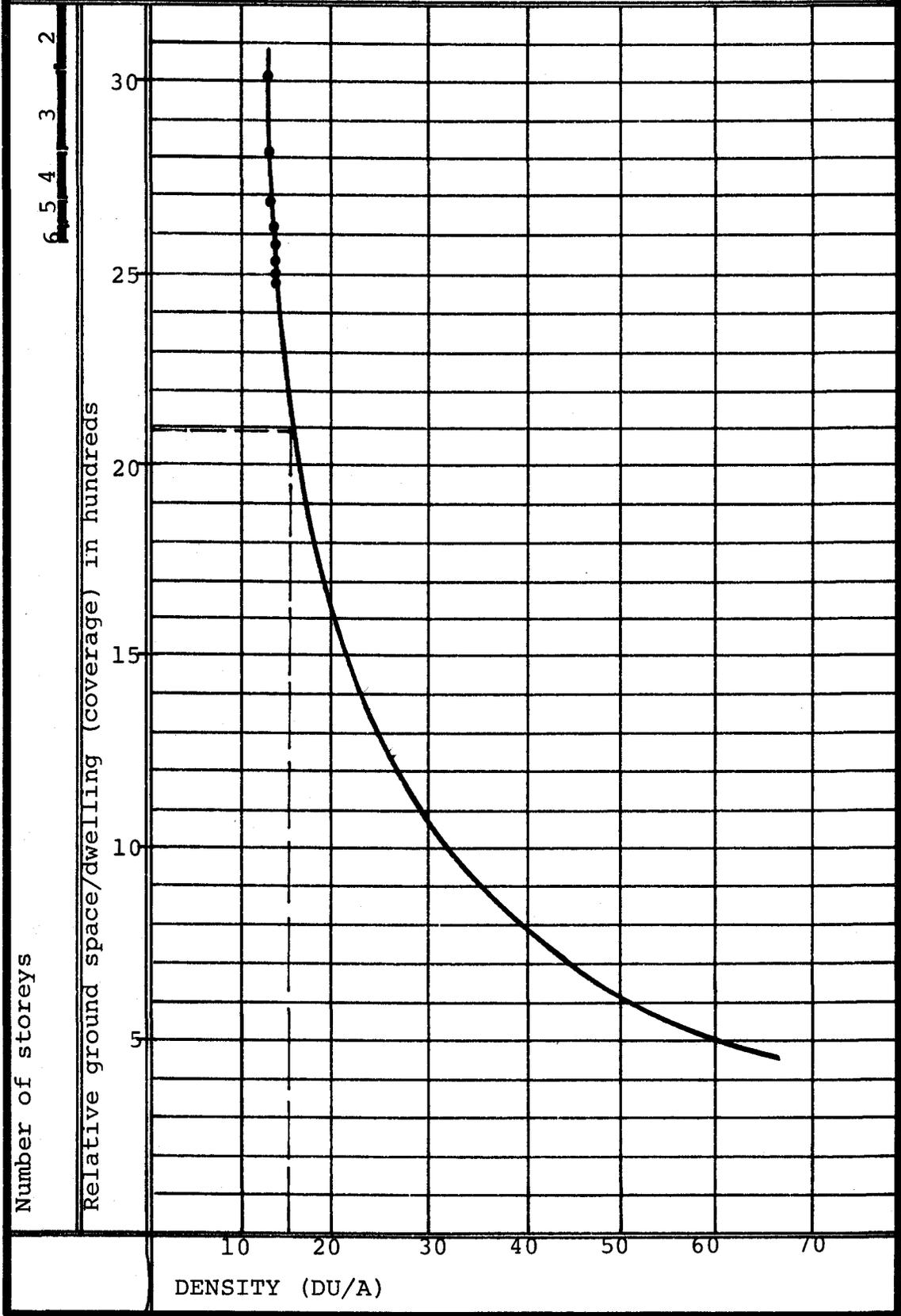
Fig. 11.12 BASIC DENSITY CURVE (WITH 75 FAM. RATIO FOR OPEN SPACE)
