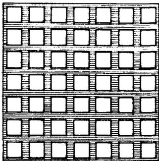
These diagrams reticulate the two contrasting built forms illustrated above. The shaded area represents open space which equals the area of built space (unshaded).
