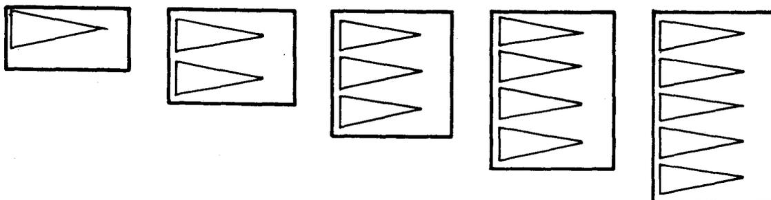
PARKING The width of a parking space dictates the minimum width of a dwelling unit. In stack schemes of 2 to 3 dwelling units, the number of cars to park requires a unit 4 modules wide. If this width is excessive, parking should be separated from dwlg unit
