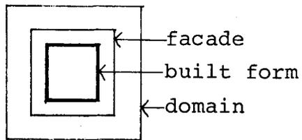
(NO) "pavilion form" isolated in the centre of its domain with four facades and no faces of extension
