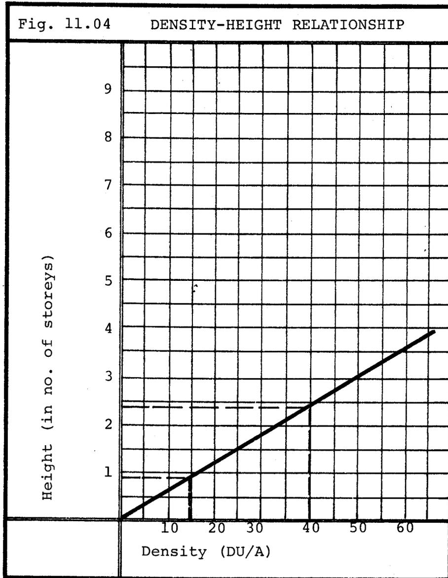
The theoretical curve given in Fig. 11.03 can be read off exactly. The answers are not, of course, practical - for example two and a half storeys would not be built. Fig. 11.05 illustrates that equal volumes may be distributed in a variety of ways while satisfying practical requirements.
