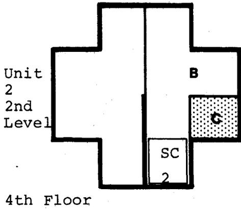
The plan below has a ground floor area of 12 modules. Therefore for a single family on two floors, the unit is oversize. It should be 9 modules.
