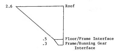
The designer is to consider the AF's noted above as acting independently in order to simplify the analysis and eliminate the use of combined loading requirements.
