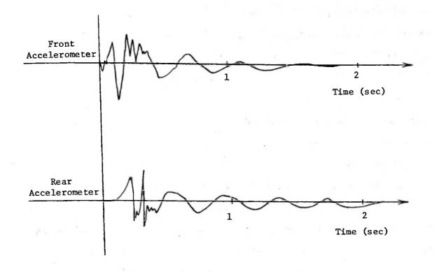
FIGURE 14. FRONT AND REAR VERTICAL ACCELEROMETER TRACES FOR T-7A NATURAL FREQUENCY TEST
