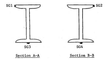
Note: Strain gages 1 through 4 were added only for static loading.
