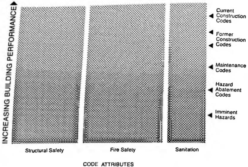
Conceptual Diagram of Various Levels of Building Performance Implied by Various Types of Building Regulations
