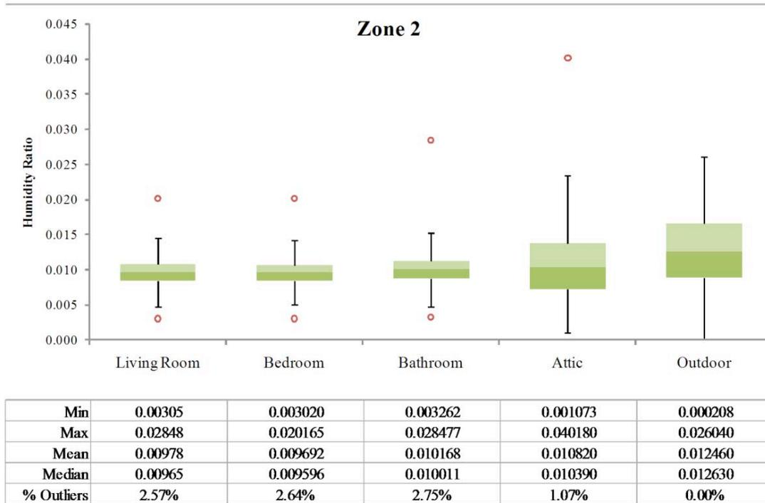
**Figure 11. Relative Humidity Box Plots for Zone 2, Hot-Humid Southeast Climate for Each Sensor Location**
