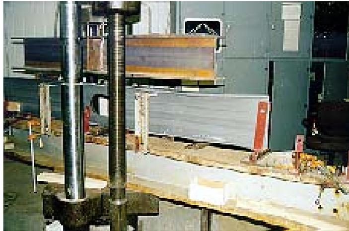
Joist Failure – Combined Shear and Bending
