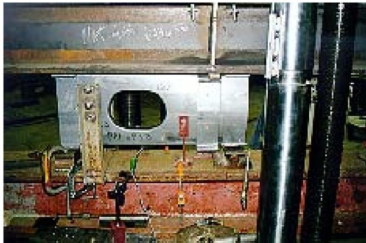
Joist Failure – Shear Test
