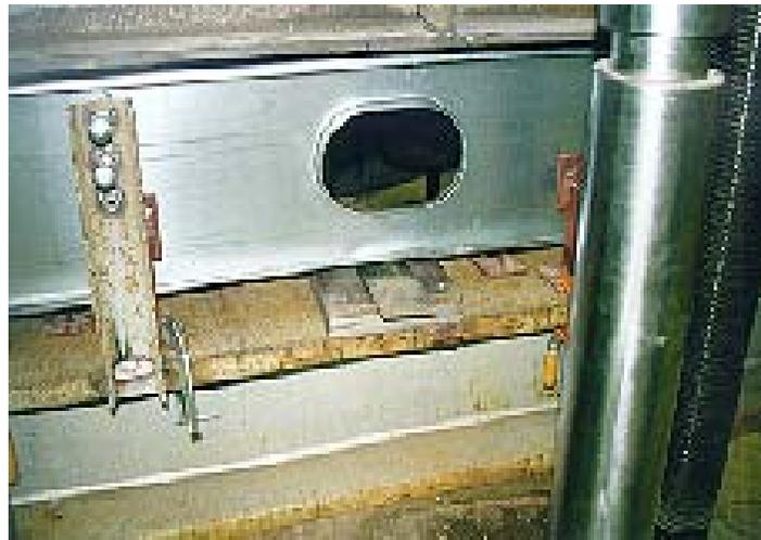
Joist Failure –Combined Shear and bending Test
