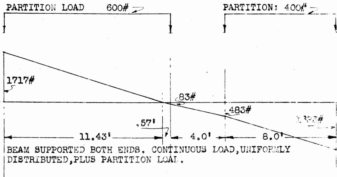
BEAM SUPPORTED BOTH ENDS, CONTINUOUS LOAD, UNIFORMLY DISTRIBUTED, PLUS PARTITION LOAD.
