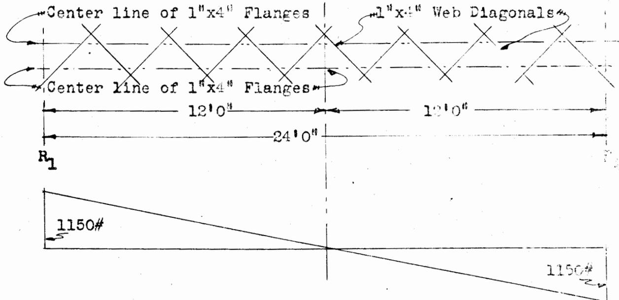
BEAM SUPPORTED BOTH ENDS, CONTINUOUS LOAD, UNIFORMLY DISTRIBUTED.
