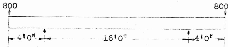
Inasmuch as this truss carried a balanced load, the reactions are equal and based upon the assumptions of 96 #/lineal foot, total load is found to be:
