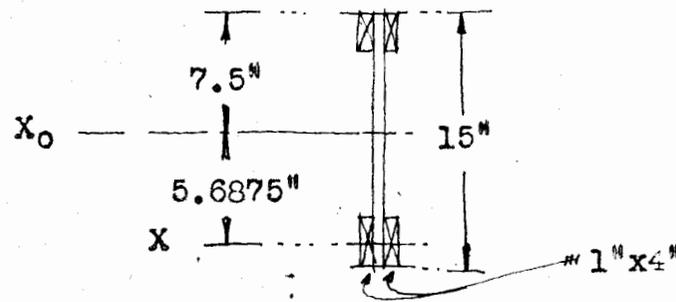
But there is another consideration. The web, composed of diagonals at  $45^\circ$  with the horizontal, must be able to withstand the vertical shear, which is a maximum at the support.
