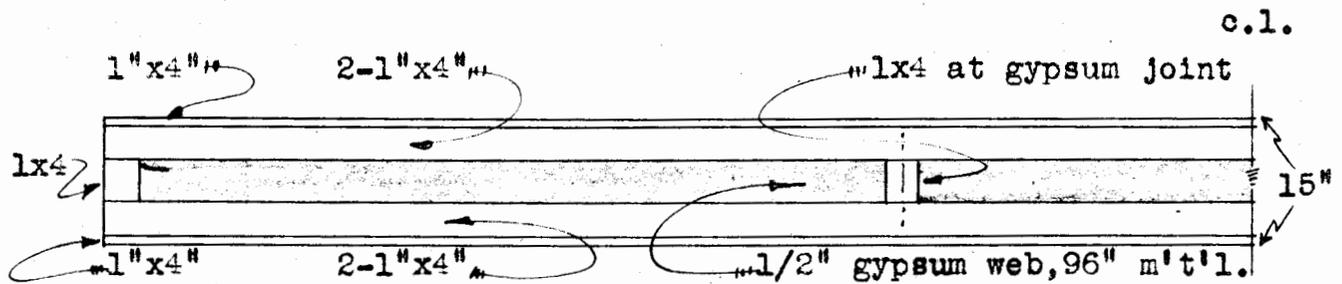
Based upon calculations made for Floor Truss Test #120. No basis for allowing values for web material.
