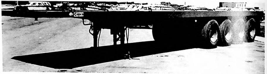
AN EXPANDABLE FLATBED SUITABLE FOR TRANSPORTING COMPONENTS
