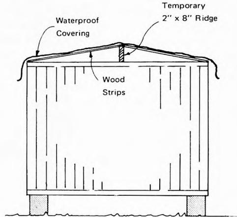
MSC MODULE SHOWING TEMPORARY ROOF COVERING STRUCTURE
