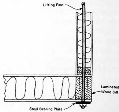
EMBEDDED LIFTING ROD DETAIL
