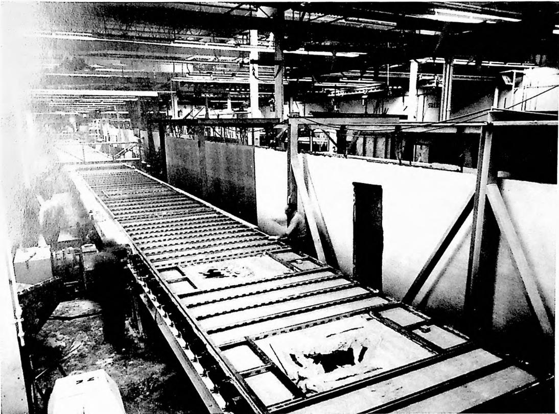
FABRICATION OF THE GENERAL ELECTRIC "CAST PLASTER" WALL
