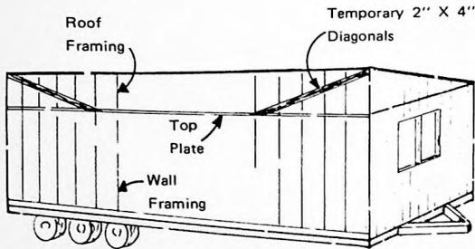
TEMPORARY 2" X 4" DIAGONALS INSTALLED IN SIDEWALL ABOVE WALL PLATE LINE TO RESTRAIN LONGITUDINAL MOVEMENT CAUSED BY SUDDEN BRAKING.
