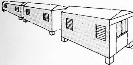
LOUVERS INSTALLED TO REDUCE INTERIOR MOISTURE ENTRAPMENT
