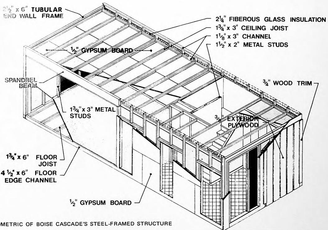
ISOMETRIC OF BOISE CASCADE'S STEEL-FRAMED STRUCTURE
