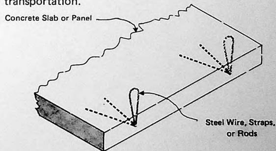
HANDLING & ERECTION LOOPS
