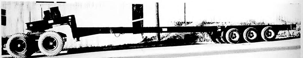
LEVELING SYSTEM POWER-SOURCE LOCATED ABOVE FIFTH-WHEEL HITCH
