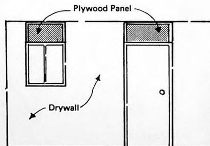
HBC CONSTRUCTION METHOD TO PREVENT DAMAGE
