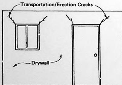
DAMAGE WITH TRADITIONAL CONSTRUCTION METHOD
