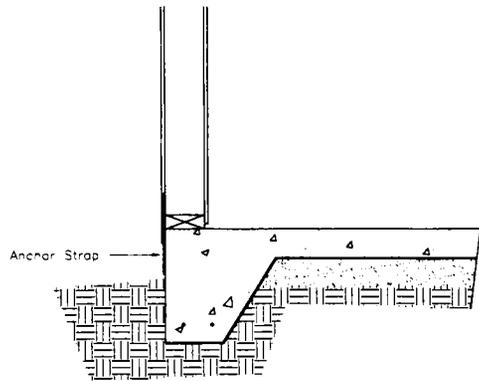
**Figure 12. Hydraulic Shot-Nail Wall Anchorage.**
