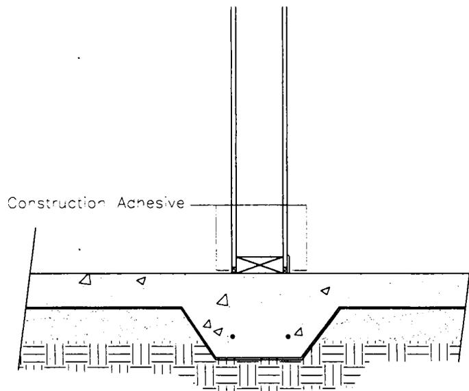
**Figure 13. Construction Adhesive Securing Partition Walls**
