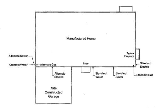
These suggestions assume utilities are located in the street. If utilities are along the rear or side lot lines, adjustments would be made. Also, frost protection measures would modify some of these set-ups
