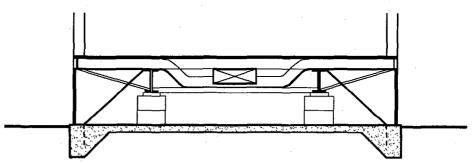
Pier and tie-down foundation on full concrete slab or transverse strip slabs.
