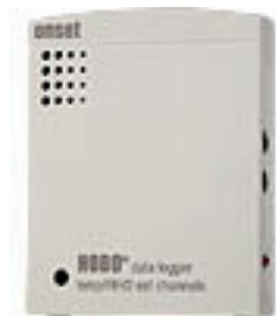
Subsequent to the short-term assessment, engineers installed the HOBOS for long-term monitoring of temperature and relative humidity. The data loggers collected the following data:
