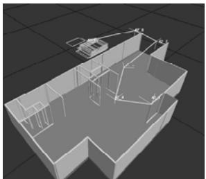
Fig. 2.7: Path complexity increases to avoid interference with standing panels
