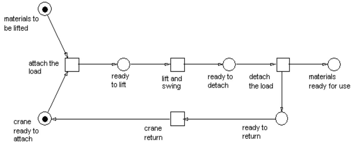
Figure 2.2: Tokens “fired” through the “attach-to-load” transition into the “ready-to-lift” place-circle
