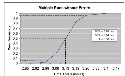
Figure 3.62: Cumulative frequency distribution of multiple panel simulation run without errors
