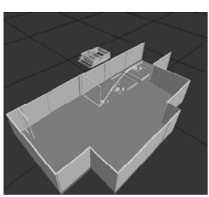
Fig. 2.6: Exterior panels set, paths for interior panel staging
