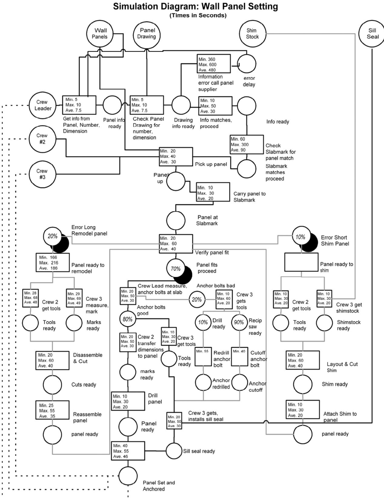
Fig. 3.59: Petri Net simulation diagram for wall panel setting
