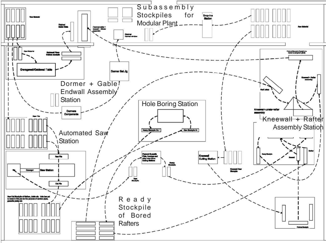
Fig. 3.1: Component plant layout diagram
