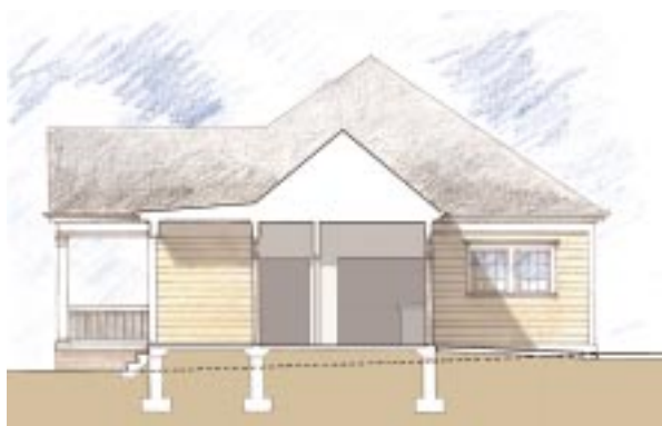
Cross section indicating raised slab construction with alignment of the accessible route indicated by the dotted line.
