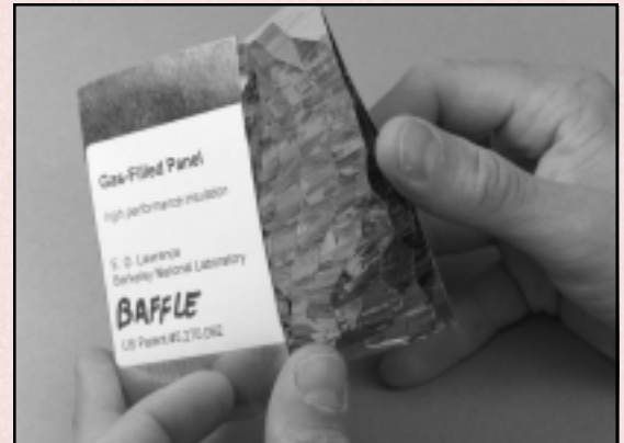
A sample of a GFP baffle, removed from its barrier bag. Inert gas fills the sealed interior of the panel.
