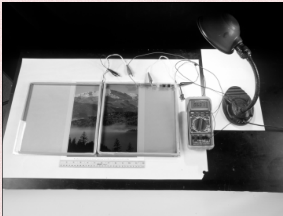
Mid-sized photoelectrochromic window turning dark under a voltage applied by two small PV cells attached to the side of the window.
