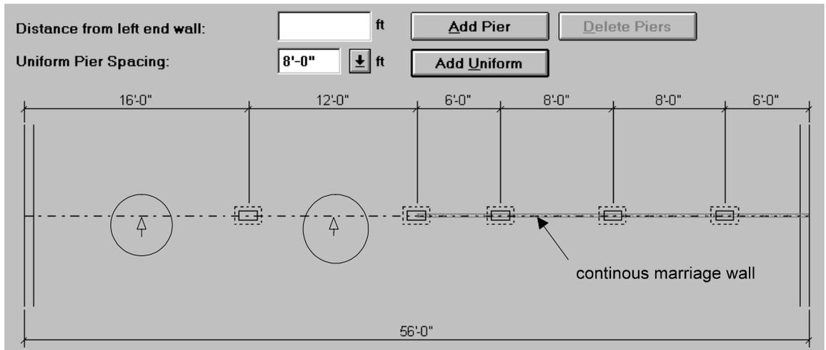
It is possible to move any individual pier by placing the mouse pointer on the pier. Note that a double arrow head will appear similar to that shown below within the dotted circle. Hold the mouse key down and scroll left or right to
