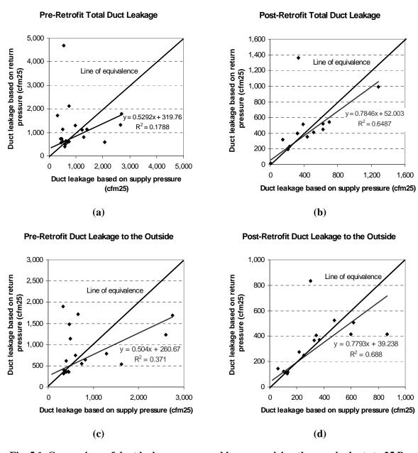
Fig. 5.1. Comparison of duct leakages measured by pressurizing the supply ducts to 25 Pa with those measured by pressurizing the return ducts to 25 Pa.
