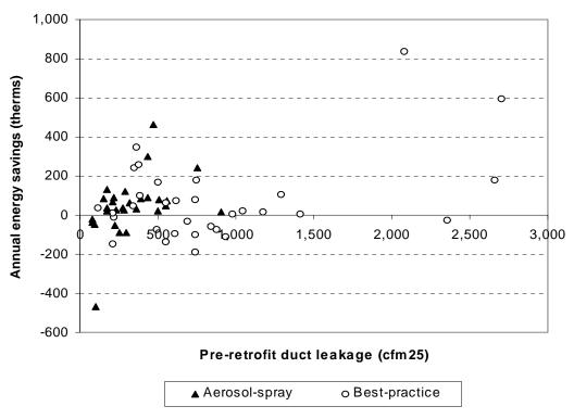
Fig. 7.2. Energy savings as a function of pre-retrofit total duct leakage based on supply pressure.
