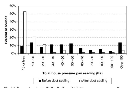
Fig. 6.1. Pre- and post-retrofit distributions of total house pressure pan readings.
