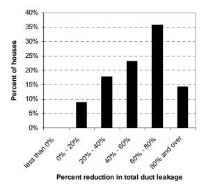
Fig. 5.4. Distribution of total duct-leakage reductions based on pressurizing the supply ducts to 25 Pa.
