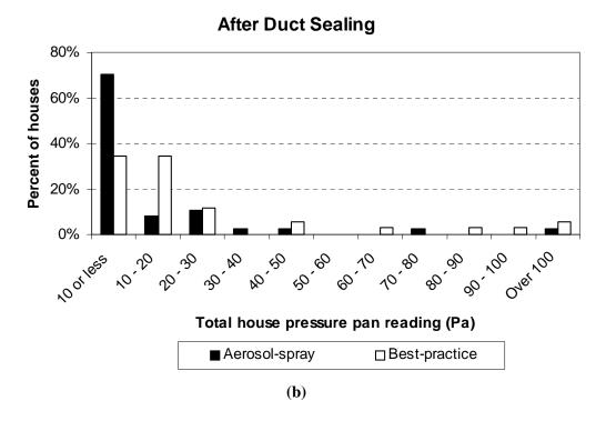
Fig. 6.4. Pre- and post-retrofit distributions of total pressure pan readings for the aerosol-spray-treated and best-practice-treated houses.
