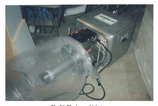
Fig. 2.1. The Aeroseal injector.
