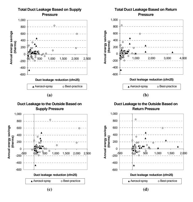
Fig. 7.1. Energy savings as a function of duct leakage reduction.
