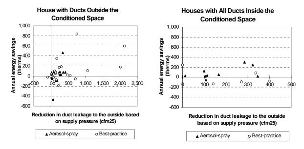
Fig. 7.3. Annual savings for houses with ducts located completely inside the conditioned space of the house and for those with some ducts located outside the conditioned space.
