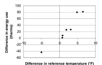
Fig. 3.2. The difference in energy use calculated by the ASAP and alternative analysis methods for a sample of houses as a function of the difference in reference temperature used in each model.
