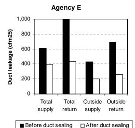
Fig. 5.8. Average pre- and post-retrofit duct leakages for each of the five weatherization agencies participating in the field test.
