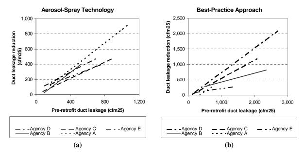
Fig. 5.10. Comparison of total duct leakage reductions (based on supply pressure) achieved by each weatherization agency, as a function of pre-retrofit total duct leakage using the aerosol-spray and best-practice technologies.
