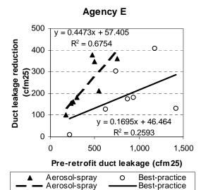
Fig. 5.11. Comparison of total duct leakage reductions (based on supply pressure) achieved by each weatherization agency using the aerosol-spray and best-practice technologies.
