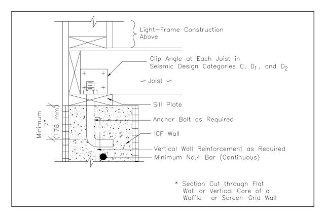
Figure 6.2 Floor on ICF Wall Connection (Top-Bearing Connection)
