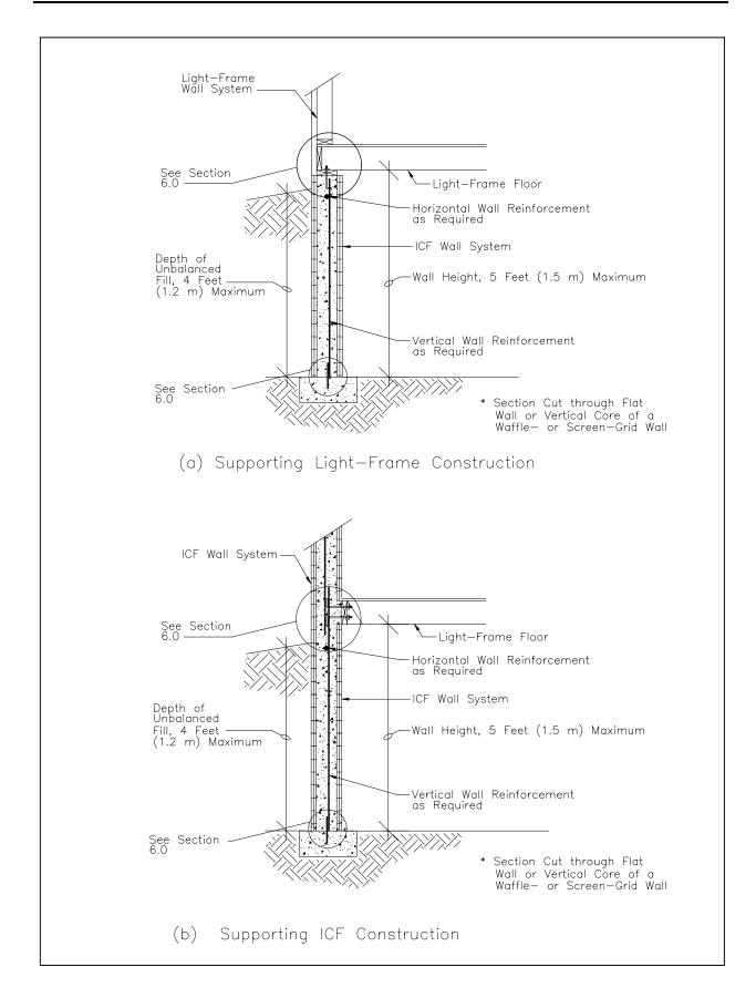
Figure 3.2 ICF Crawlspace Wall Construction
