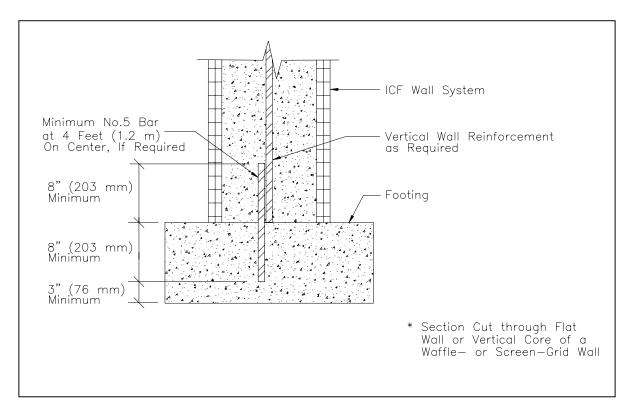
Figure 6.1 ICF Foundation Wall-to-Footing Connection
