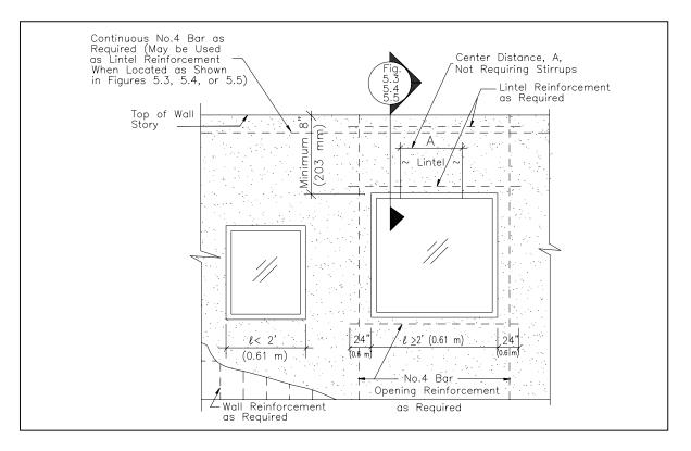
Figure 5.2 Reinforcement of Openings
