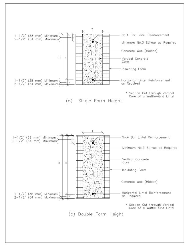
Figure 5.4 Waffle-Grid ICF Lintel Construction
