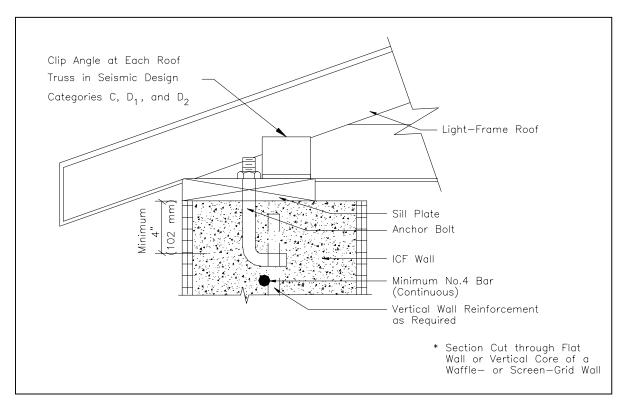
Figure 6.8 Top Wood Sill Plate-ICF Wall System Connection
