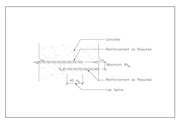
Figure 2.4 Lap Splice Requirements
