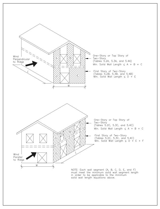
Figure 5.1 Variables for Use with Tables 5.2 through 5.4
