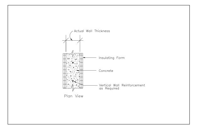
Figure 2.1 Flat ICF Wall System Requirements
