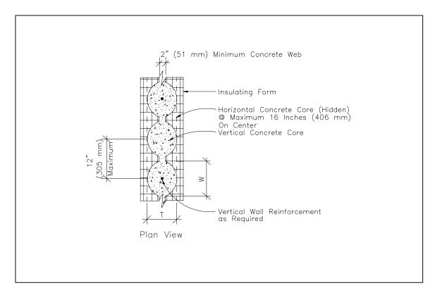
Figure 2.2 Waffle-Grid ICF Wall System Requirements
