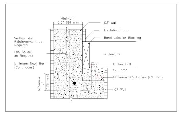
Figure 6.3 Floor on ICF Wall Connection (Top-Bearing Connection) (Not Permitted is Seismic Design Categories C, D<sub>1</sub>, or D<sub>2</sub> Without Use of Out-of-Plane Wall Anchor in Accordance with Figure 6.5)
