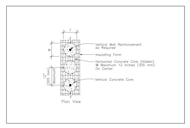
Figure 2.3 Screen-Grid ICF Wall System Requirements
