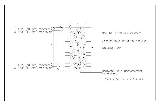
Figure 5.3 Flat ICF Lintel Construction
