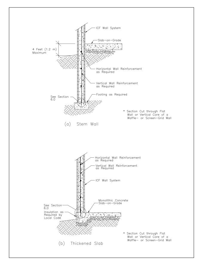
Figure 3.1 ICF Stem Wall and Monolithic Slab-on-Grade Construction
