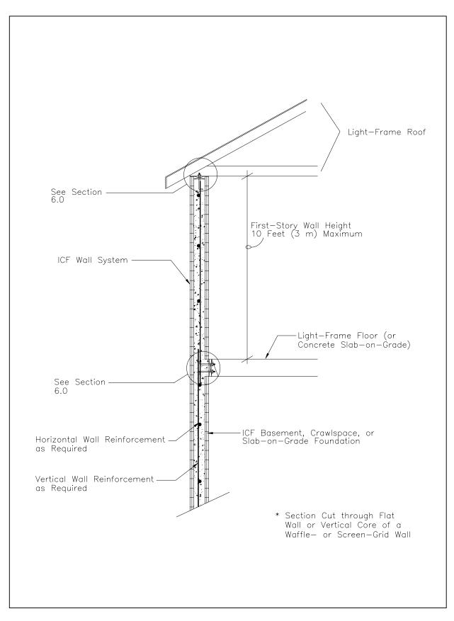
Figure 4.1 ICF Wall Supporting Light-Frame Roof
