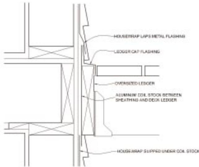
FIGURE 2 LEDGER FLASHING
