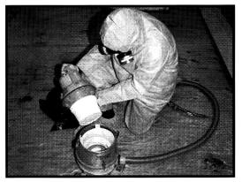
Figure 11.16e Wash or Replace Coarse Prefilters if Necessary.
