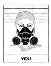
A Half-Mask, Air-Purifying Respirator with HEPA Cartridges Is Appropriate for Many Residential Lead Hazard Control Jobs. Paper Dust Masks are NOT Adequate.
