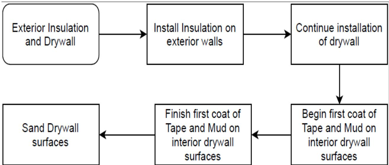
**Exhibit 81. Station 7: Exterior Insulation and Drywall**
