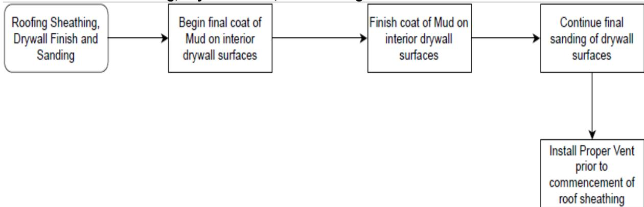
**Exhibit 85. Station 9: Roof Sheathing, Drywall Finish, and Sanding**
