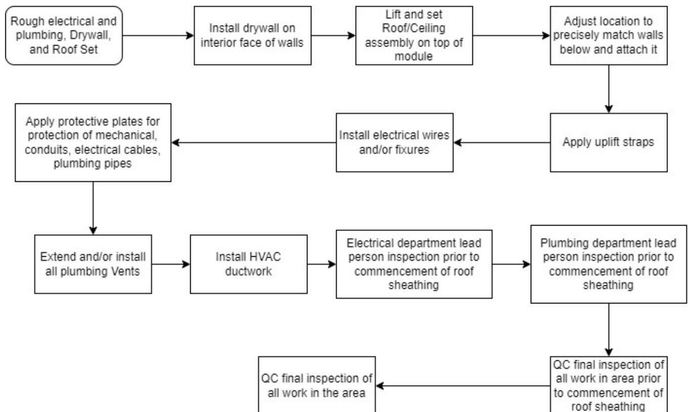
**Exhibit 79. Station 6: Rough Electrical and Plumbing, Drywall, and Roof Set**
