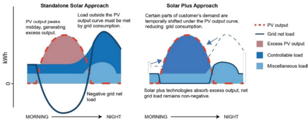
**Figure 2. Customer load shifting through solar plus**
