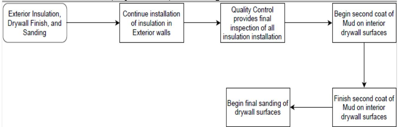
**Exhibit 83. Station 8: Exterior Insulation, Drywall Finish, and Sanding**
