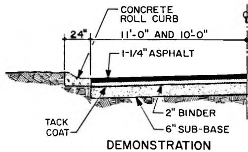
Street widths were reduced from 26 to 20 feet on permanent dead end streets and from 26 to 22 feet on all other subdivision streets. Paving thickness requirements were reduced from 8-inch base, 2-inch binder, and 2-inch asphalt top coat to 6-inch base, 2-inch binder, tack coat, and 1-1/4-inch asphalt top coat. The asphalt top coat was applied after 75 percent of construction was completed.
