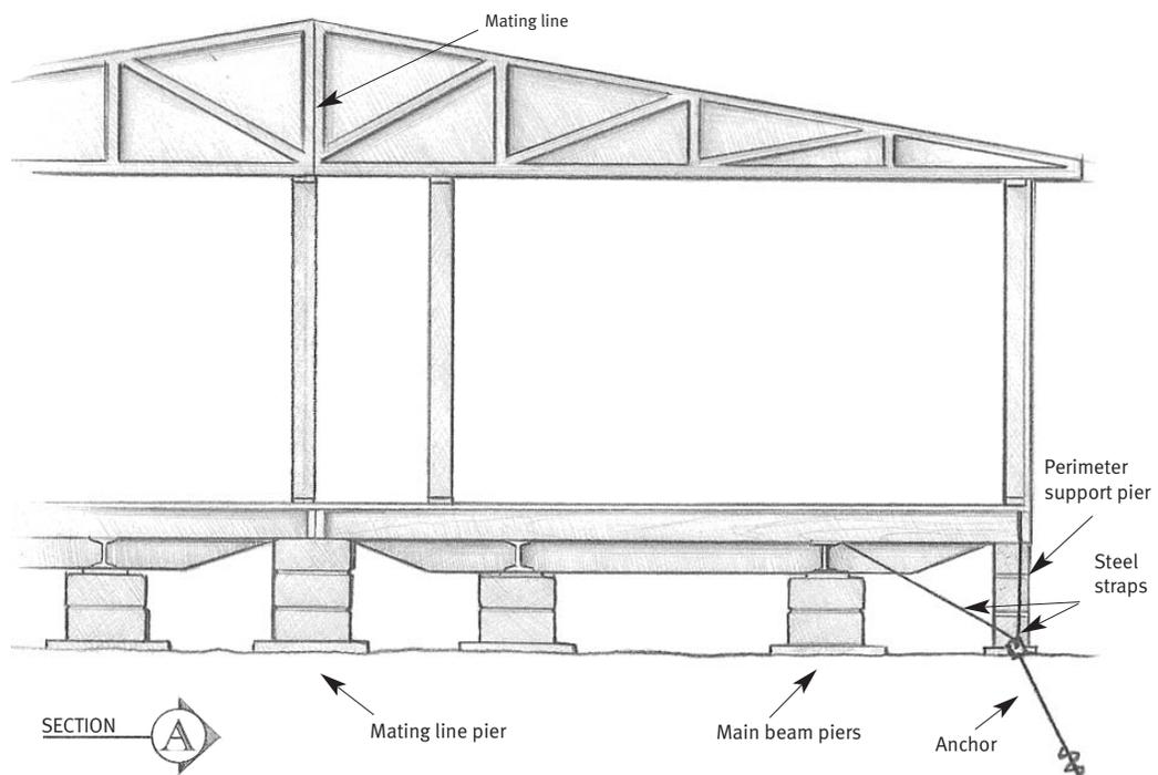
**Figure 3.2** Cross section of pier and anchor foundation.
