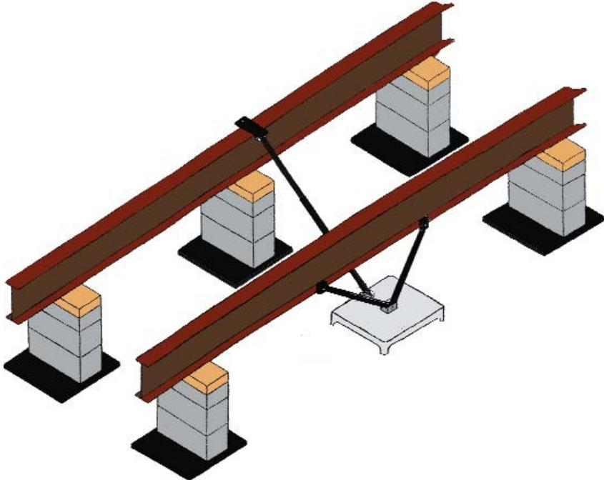
**Figure 4.2** All Steel Foundation Model #1100 "V."
