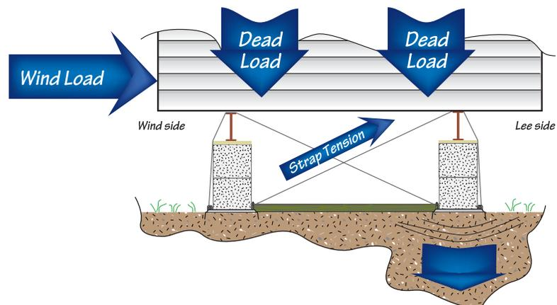
**Figure 4.35** The dynamics of the Vector system.
