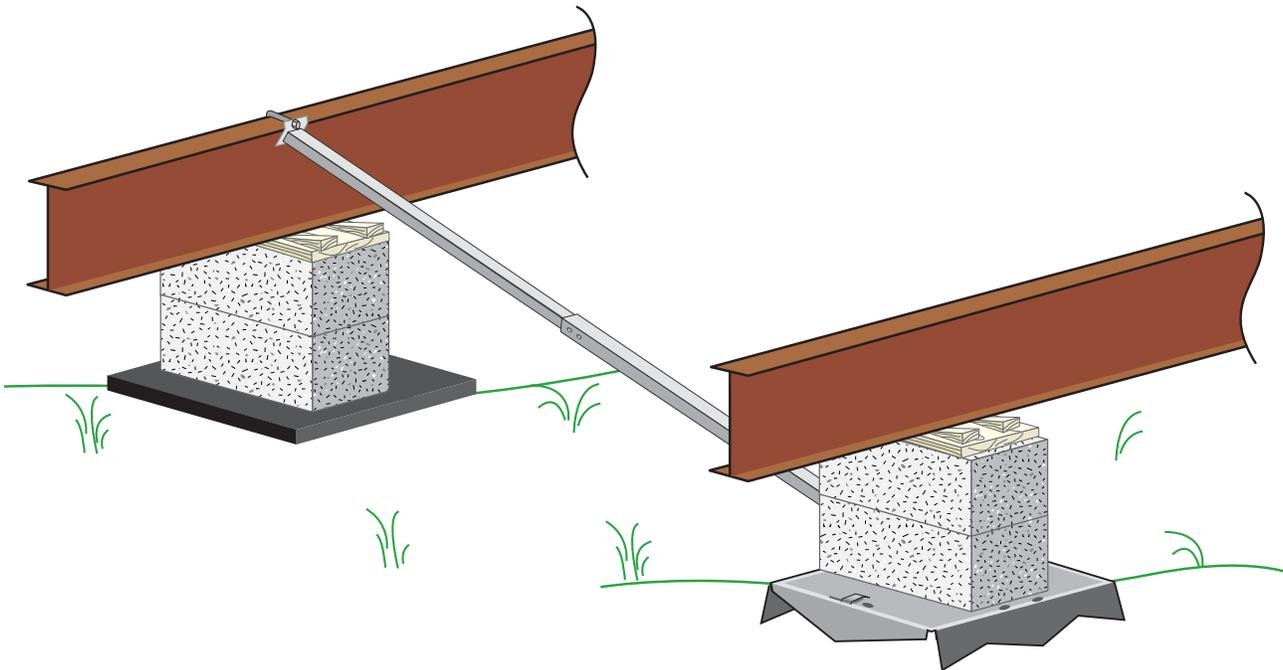
Figure 4.37 Wind Zone 1 with concrete pier lateral system.
