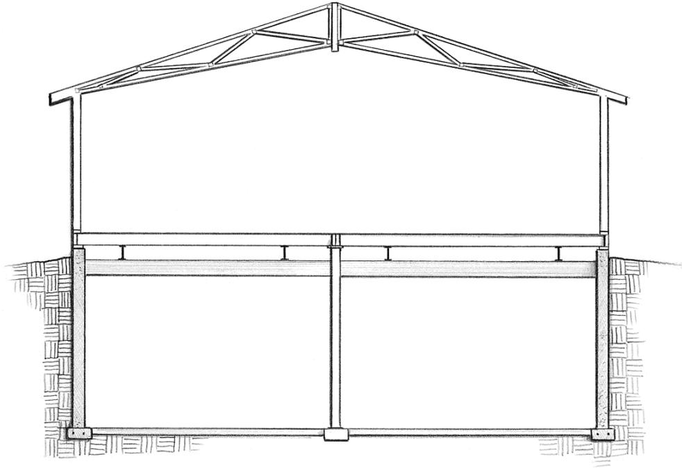
**Figure 3.59** Cross section of a typical basement. The depth of the foundation walls lends this system to use in areas with deep frost.
