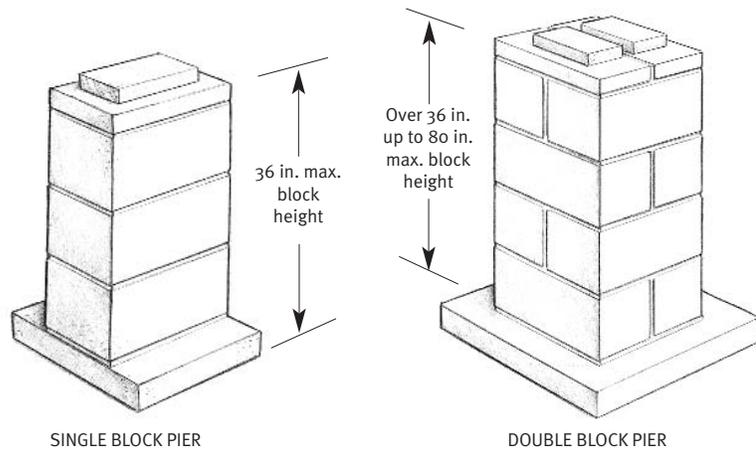
**Figure 3.3.** Common configuration of concrete block piers.
