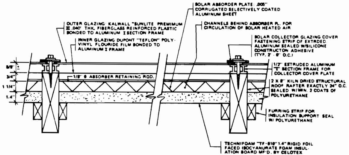
HORIZONTAL SECTION THRU ROOF INTEGRATED SOLAR COLLECTOR
