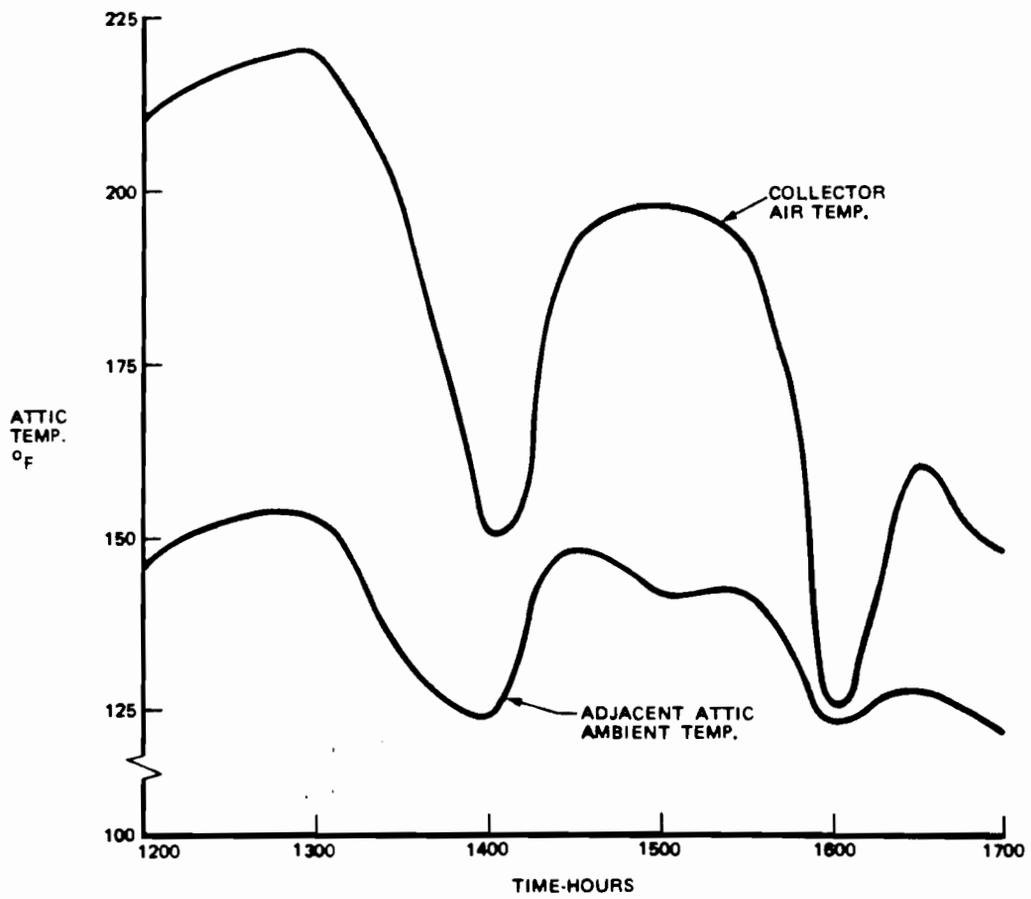
Figure 5-6. Maximum Air Temperatures, Site-Built Collector, Configuration 3
