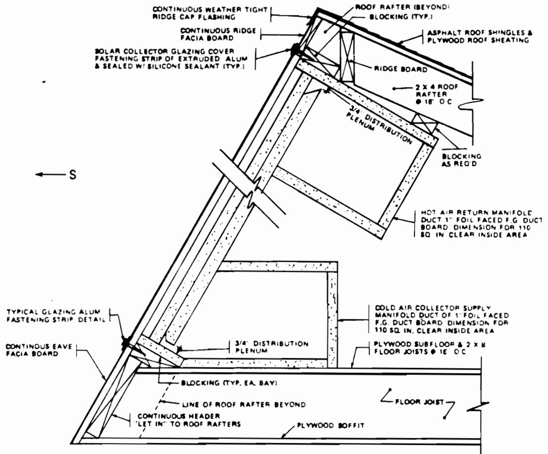
VERTICAL SECTION THRU ROOF INTEGRATED SOLAR COLLECTOR WITH SUPPLY & RETURN
