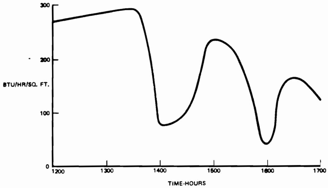
Figure 5-5. Solar Insolation, Site-Built Collector, Configuration 3
