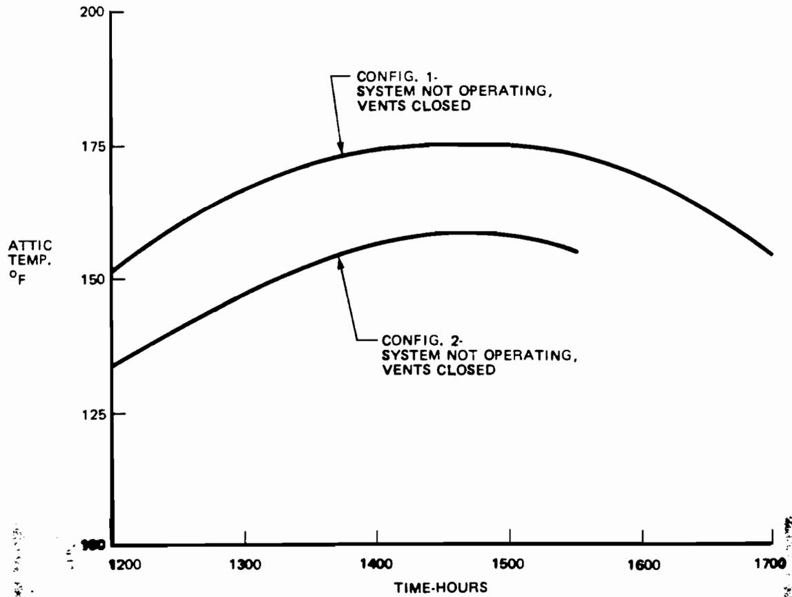
Figure 5-3. Maximum Attic Ambient Temperatures, Vents Closed
