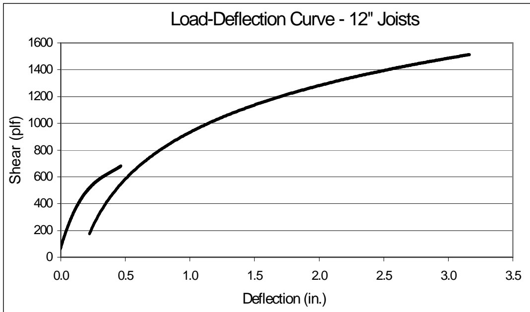
Figure B4 - Shear Load-Deflection Curve for FD12-54-2
