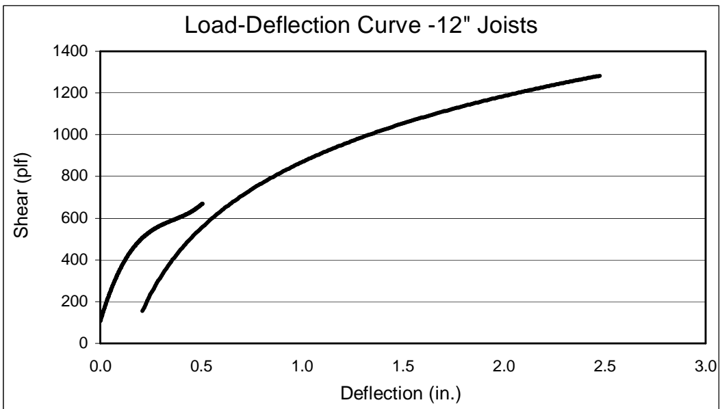
Figure B2 - Shear Load-Deflection Curve for FD12-54-1
